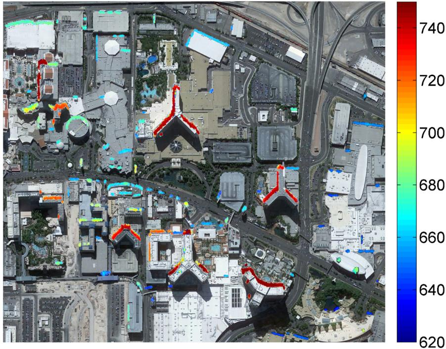
Fig. 19. Extracted façade points from TomoSAR point cloud depicted in Figure 16 overlaid onto the corresponding optical image (©Google).
