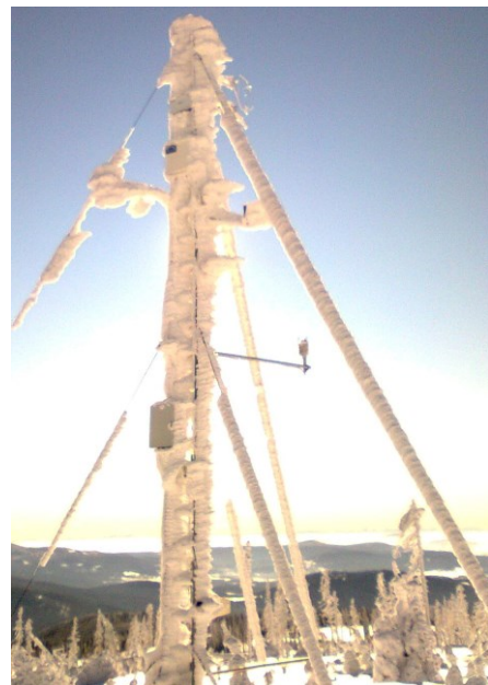
Figure 19: Measurement tower in January 2012. Most time of the winter instruments are frozen. (Photo: B. Wolpert)
