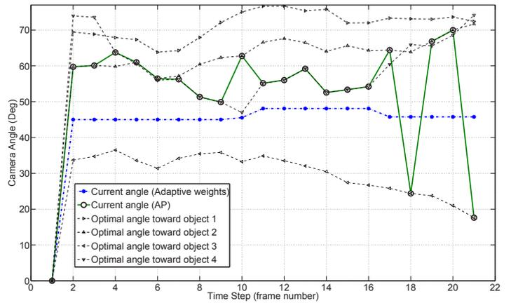
Fig. 4: Camera angle of simulation with static objects: Blue star line: actual pan angle with TAC; Green circle line: actual pan angle with AP; Other lines: the directions when the camera faces directly towards objects.
