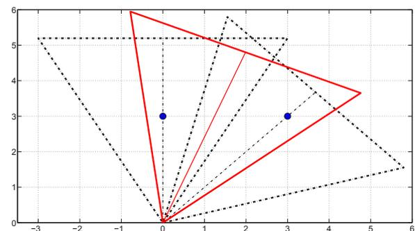
Fig. 1: Temporal attention control: due to the limited field of view, the camera direction is switched to achieve an optimal tracking performance. Some possible directions and fields of view: towards a single object (black dash dot line); covering multiple objects (red solid line).
