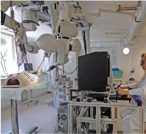
Fig. 1. **The ARAMIS system.** Four ceiling mounted manipulators are tele-operated via a master console. The robots can either be equipped with a surgical tool or an endoscopic stereo camera. For a high immersion, the surgeon is located in front of a stereo display and operates the system with haptic devices.
