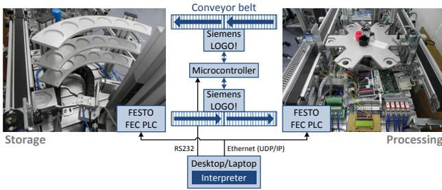
Fig. 2. A demonstrator setup of the FESTO Modular Production System.
