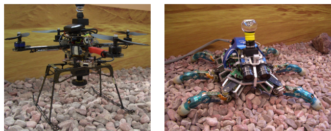
(a) flying robot with a catadioptric (up) and fisheye (down) camera (b) crawling robot with a catadioptric (up) and fisheye (down) camera
