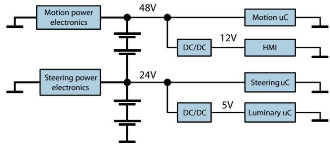
Fig. 4. Overview of the energy network of the eCar
