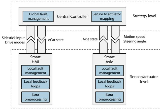
Fig. 6. Software architecture of the eCar
