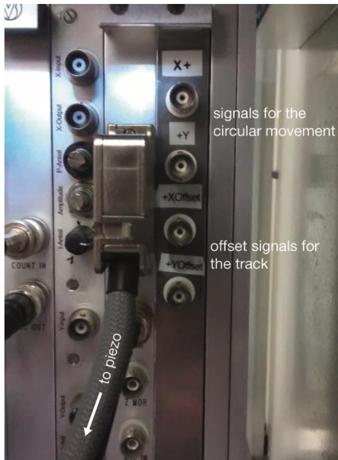
Figure 12. Addition board (right slide), which takes up the circular movement signals as well as the offset signals (which will be described later) coming from the LabVIEW program and adds them to the position signals coming from the control system. The resulting voltages are applied to the piezo through the cable pointing downwards.
