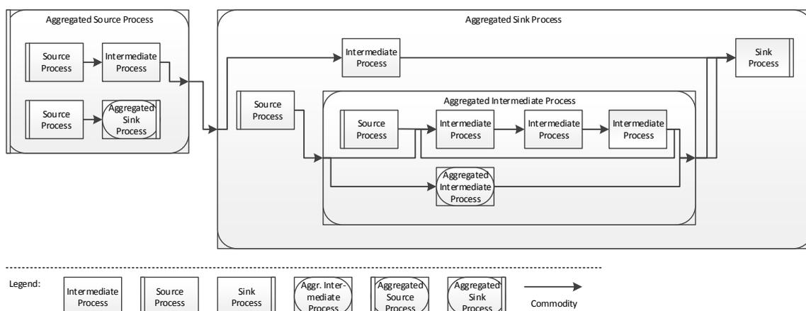
Figure 2: Abstract energy system showing the relationships between all of the defining elements of USES including their sub-elements by taking advantage of the default graphical USES representation.
