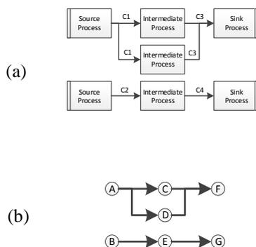
Figure 9: Abstract energy system in (a) USES (b) graph representation, fully disaggregated.
