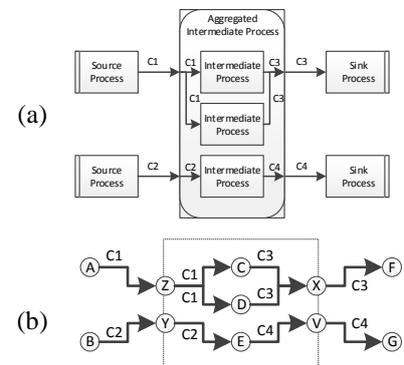
Figure 11: Abstract energy system in (a) USES (b) graph representation, aggregated and disaggregated.
