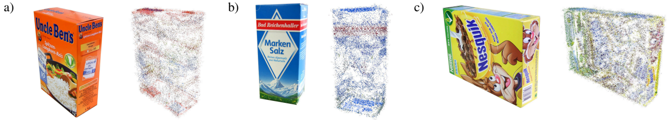
Fig. 5. Photos (left) and initial keypoint models (right) of the objects used in the evaluation. a) rice, b) salt, c) cereals. Note that the photos are shown for illustration only, they have not been used during model generation.
