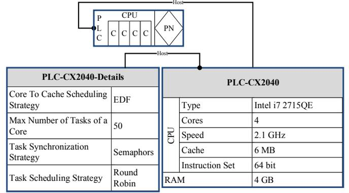
Fig. 2. MPLC modeling elements
