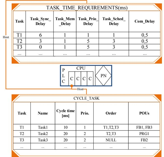
Fig. 3. Automation task requirements
