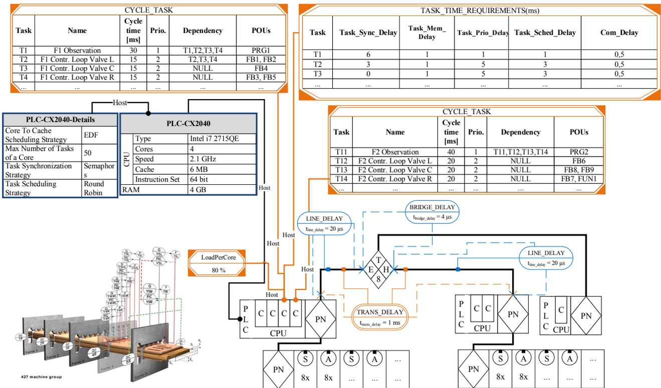
Fig. 4. Using MPLC modeling notation for modeling a hydraulic press
