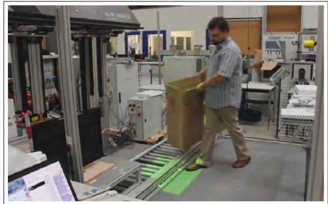
Fig. 2. An image of the CustomPacker HRI packaging cell prototype showing a worker putting the carton on the conveyor belt during the productive mode. The assistance system is providing instructions and light patterns (green light on shop floor) to guide the worker.
