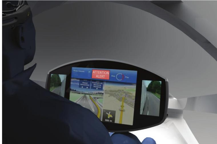
Figure 4. The EEG helm can be comfortably worn while the prototype vehicle is driven with conventional human-machine interfaces (Image by Juan Jose Gonzalez Herrero)
