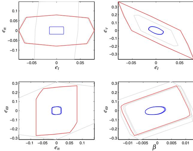
Fig. 6. Reachable sets on which the *enclosure condition* (3) has been tested for all three maneuvers  $m_i$  which connect to the *RS*-maneuver. The three initial sets are plotted in gray, the final sets in blue (sometimes overlapping), and the initial set of the *RS*-maneuver in red. The enclosure conditions are fulfilled since the final sets are all included in the initial set of the *RS*-maneuver.
