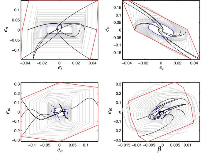
Fig. 5. Reachable sets on which the *enclosure condition* (3) has been positively tested for a transition from the *parameterized RR* maneuver to itself. The initial set of the maneuver is plotted in red, the final set in blue, reachable sets of intermediate time intervals in gray, and exemplary simulations of the system behavior in black. The enclosure condition is fulfilled since the final set is fully contained in the initial set.
