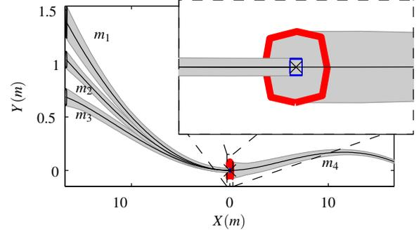
Fig. 2. Valid concatenation of predecessor maneuvers  $\{m_1, m_2, m_3\}$  to a successor maneuver  $m_4$ . Final sets  $\mathcal{R}^i(t_i^f)$  are plotted by thin blue lines, the initial set  $\mathcal{R}_0^4$  by thick red lines, the reachable sets in gray color, and the marker 'x' refers to the point  $x_{\text{ref}}^i(t_i^f) = x_{\text{ref}}^4(t^0)$  where the nominal partial reference trajectories are concatenated.
