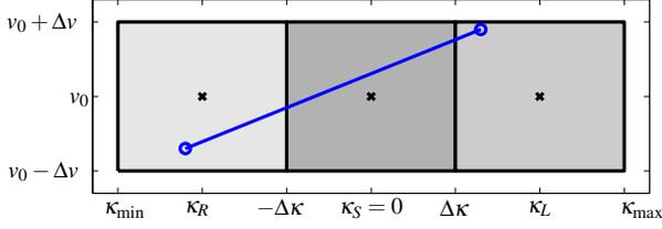
Fig. 3. Parameter space with valid example trajectory. Each parameterized motion primitive allows the uncertain set-trajectory parameters  $p_1, p_2$  to vary inside one of the grey boxes and  $p_3, p_4$  to vary inside another (or the same) box.
