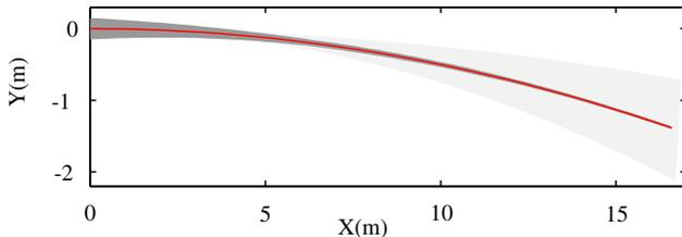
Fig. 8. Closer look at the *RR* maneuver. The red line shows the nominal reference trajectory, the light gray area shows the area covered by the reference trajectory when the parameters are uncertain, and the dark gray area shows the reachable set when following the nominal reference trajectory.
