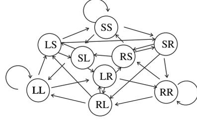
Fig. 4. The resulting maneuver automaton.  $S$  denotes the parameter set for straight movement,  $L$  for left movement, and  $R$  for right movement. Their combination refers to the transition between the parameter sets  $S, L$ , and  $R$ .
