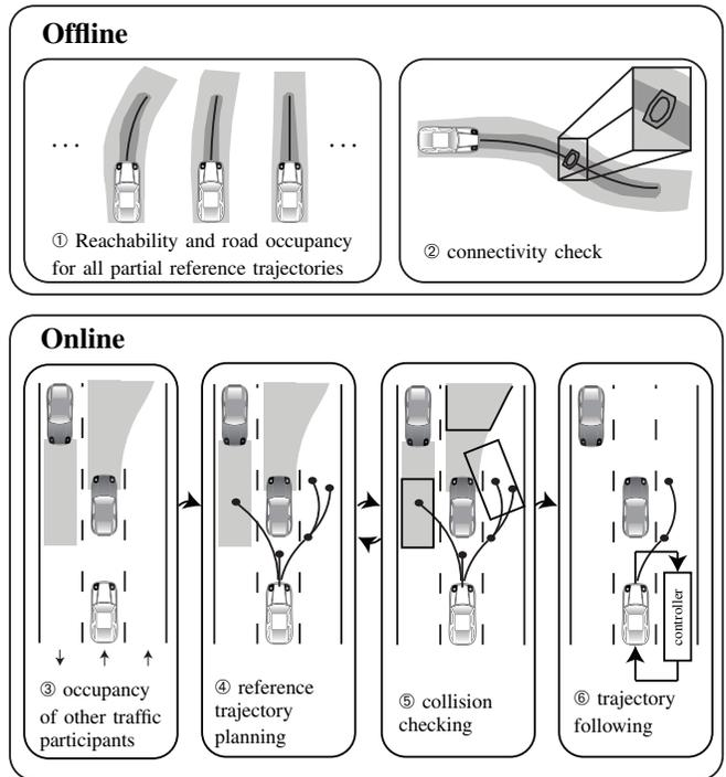
Fig. 1. Overview for formally verifying automated vehicles on-the-fly.
