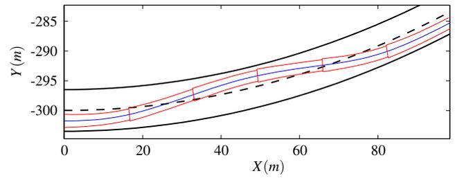
Fig. 9. Evasion maneuver on a curved road. The red areas show the occupancy of the vehicle, the blue line shows the complete reference trajectory assembled from partial reference trajectories.
