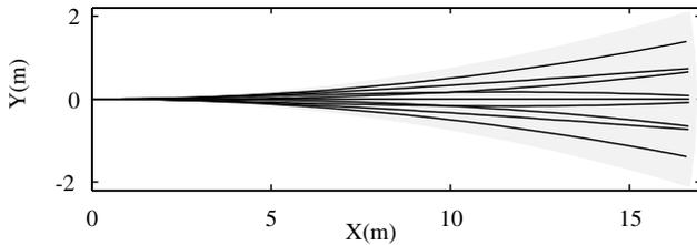
Fig. 7. Position region covered by the 9 parameterized reference trajectories for the full range of parameter values. Black lines show the 9 nominal reference trajectories (parameter value is the volumetric center of the parameter sets  $\mathcal{P}^i$ ) and the gray region shows the coverage of all reference trajectories when the parameters are within  $\mathcal{P}^i$ .
