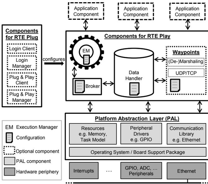
Fig. 1. Architecture of the XME run-time environment.
