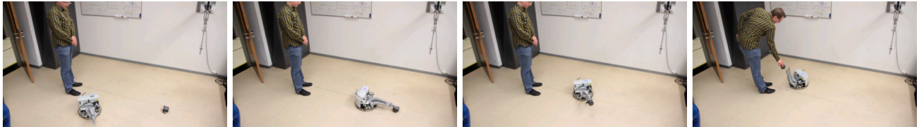
Fig. 6: The Figure shows our approach to solve pick-up tasks using the Robotino XT. First, the robot approaches the object it wants to grasp—in this case, a mug on the floor. Second, the learned policy for object grasping is employed. Subsequently, the robot delivers the object to the user, as shown in the most right picture.
