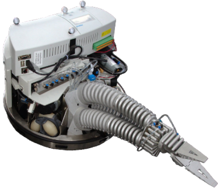
Fig. 1: The Festo Robotino XT, a mobile service robot with a pneumatic arm, used for evaluation.
