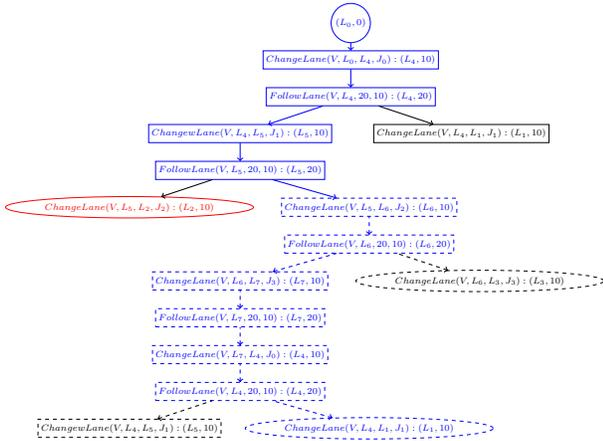
Fig. 7. Task planning for Round-about scenario. The dashed tasks are planned after detecting the task  $ChangeLane(V, L_5, L_2, J_2)$  in red is inexecutable. The node  $ChangeLane(V, L_6, L_3, J_3)$  is also a solution, but  $ChangeLane(V, L_4, L_1, J_1)$  is better with less time cost. The solution is colored in blue.
