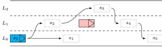
Fig. 4. Overtaking scenario: There are three lanes in one direction of a motorway. The blue rectangle is the ego vehicle and the red rectangle is a slower vehicle in front. The initial state is  $s_0$ . The arrows show the possible driving tasks planned with the internal states  $\{s_1, s_2, s_3, s_4, s_5\}$ .
