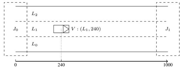
Fig. 2. Example of a world model: Places  $L_0$ ,  $L_1$  and  $L_2$  are lanes and  $J_0$  and  $J_1$  are junctions.  $L_2$  is left to  $L_1$ , while  $L_0$  is on the right of  $L_1$ .  $J_0$  is before the lanes and  $J_1$  is after them. The axis below shows a lane coordinate starting from 0 to 1000m. Object  $V$  is a vehicle at the location  $(L_1, 240)$ , i.e., on the lane  $L_1$  at position 240m.
