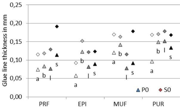
**Figure 9:** Mean glue line thickness of the test specimens produced with different timber species (a-ash; b-beech; l-larch; s-spruce)
