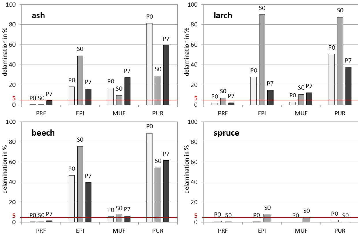
**Figure 5:** Mean delamination of the test specimens made of four different timber species (P0-planned, fresh; S0-sanded, fresh; P7-planned, 7 days of storage)
