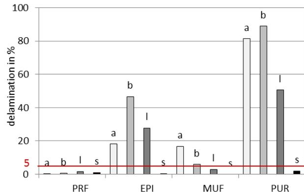
**Figure 4:** Mean delamination of the test specimens produced with different adhesives (a-ash; b-beech; l-larch; s-spruce)
