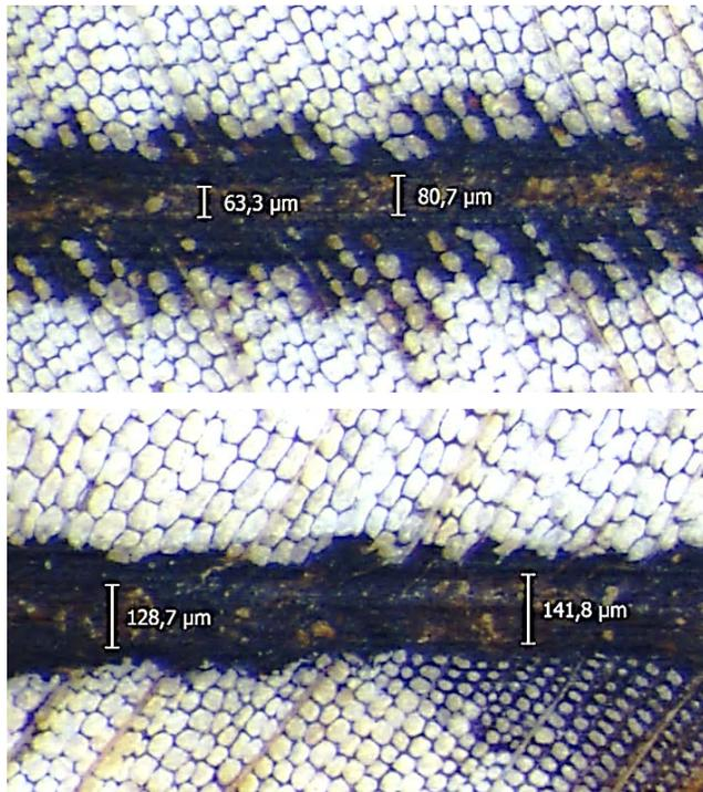
**Figure 10:** Microscopic photographs of the glue lines formed by PRF adhesive on planned (top) and sanded (bottom) surfaces of larch
