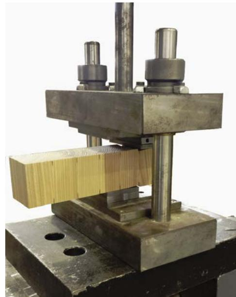
**Figure 2:** Device for the block shear test
