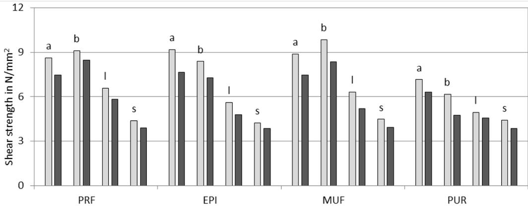
**Figure 7:** Mean shear strength of the test specimens after treatment A2 (light grey bars) and A4 (dark grey bars) (a-ash; b-beech; l-larch; s-spruce)
