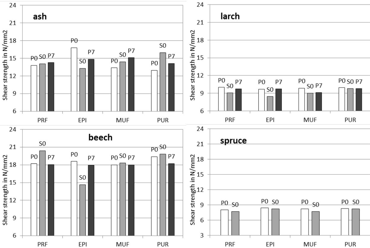
**Figure 8:** Mean shear strength of the test specimens produced with different timber species (P0-planned, fresh; S0-sanded, fresh; P7-planned, 7 days of storage)
