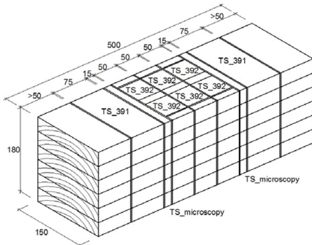
**Figure 1:** Geometry of test beams (in mm)
