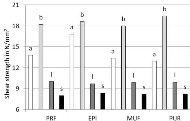
**Figure 6:** Mean shear strength of the test specimens without further conditioning (a-ash; b-beech; l-larch; s-spruce)
