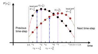
Fig. 2. Two subsystems compete for channel access by randomly choosing their waiting times  $\nu_k^1$  and  $\nu_k^2$ , according to their corresponding local probability mass functions with error-dependent means  $\mathsf{E}[\nu_k^1]$  and  $\mathsf{E}[\nu_k^2]$ .
