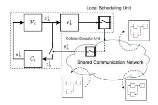
Fig. 1. A multi-loop NCS with a shared communication channel and local scheduling mechanism.
