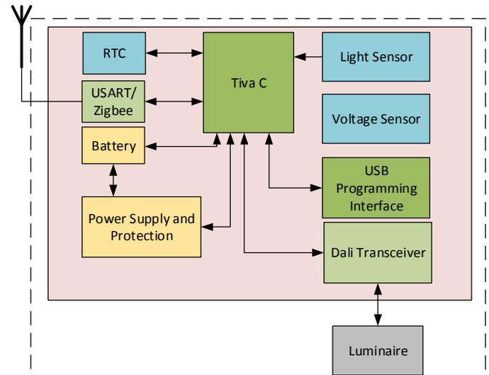
Fig. 2. Schematic of the proposed device.
