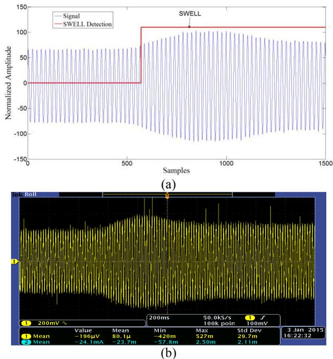
Fig. 13. Voltage waveforms. (a) Swell detection. (b). Voltage at output of the voltage sensor.
