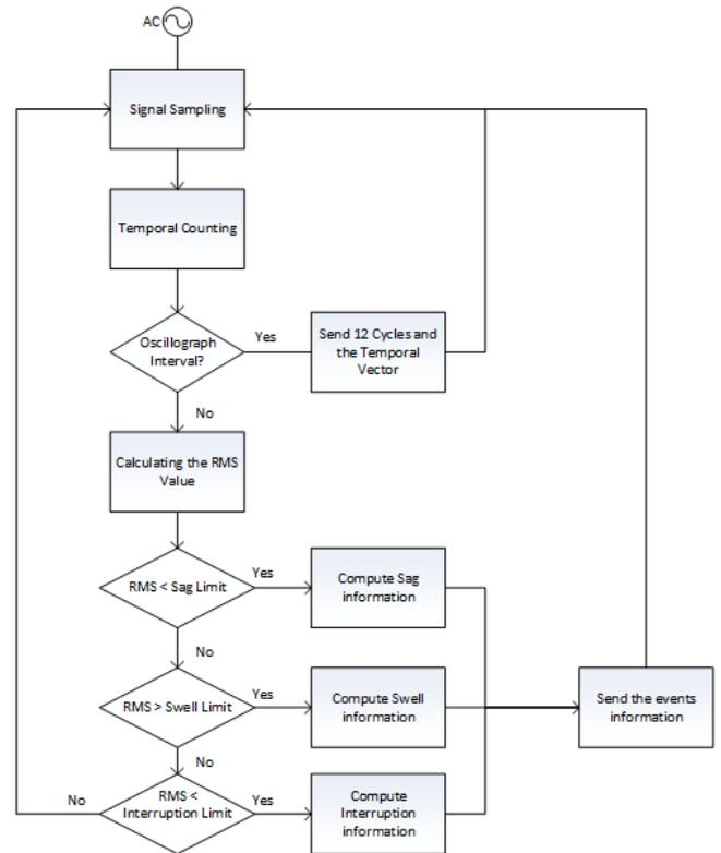
Fig. 4. Algorithm for the power quality parameters estimation and disturbances detections.
