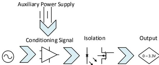
Fig. 3. Schematic of the voltage sensor.
