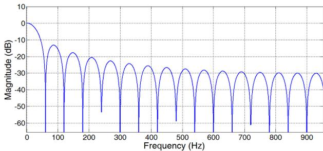
Fig. 5. Magnitude response of the recursive DFT with  $k$  equal to zero.
