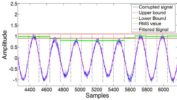
Fig. 8. Simulation result for the computation of the test signal RMS value.
