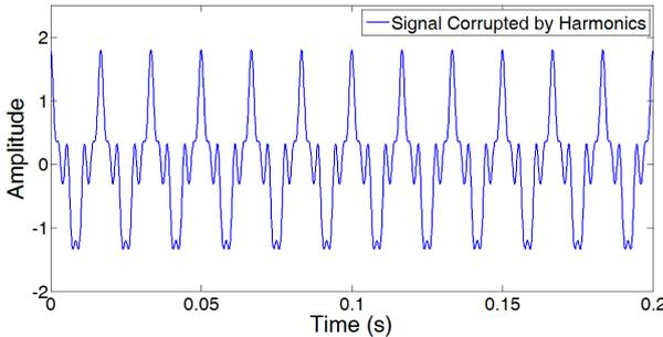
Fig. 9. Signal corrupted by third (50% energy) and sixth (30% energy) harmonics.
