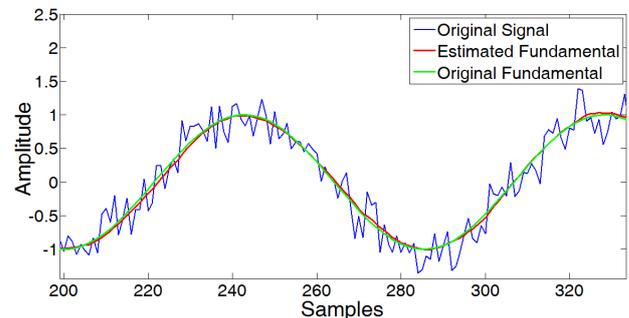
Fig. 7. Result of the filtered fundamental component utilizing the SWRDFT filter.
