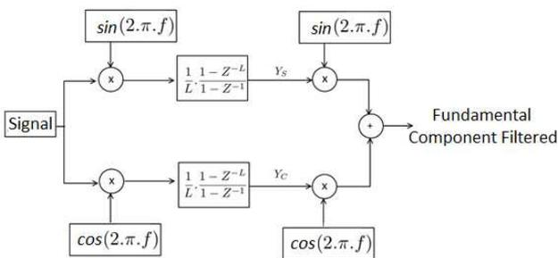
Fig. 6. Filter structure based on SWRDFT.
