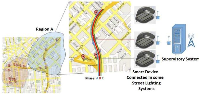
Fig. 1. Concept of the proposed smart management and control system.
