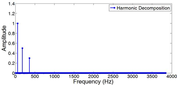
Fig. 10. Spectral estimation performed by the supervisory system showing harmonic decomposition.
