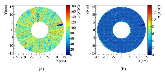
**Figure VIII.1:** Mean (a) and width (b) of the noise distribution in units of ADC channels as a function of the pad position. The dark blue areas correspond to defect electronic channels. In average a noise width of 1.83 ADC channels was achieved.
