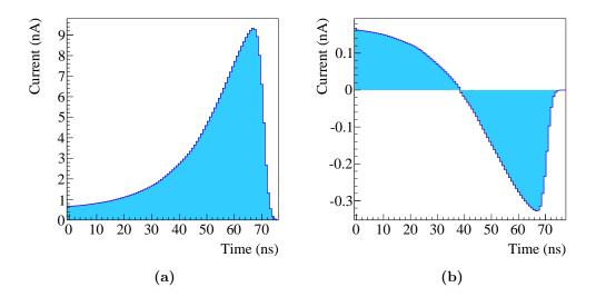
Figure VII.15: The instantaneous current on a pad as a function of the time. The left panel shows the resulting distribution for an electron cloud generated directly above the center of the pad, while the electron cloud for the distribution in the right panel was generated 3.3 mm away from the pad center.
