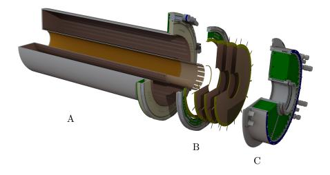
**Figure II.1:** Exploded CAD view of the GEM-TPC. Part A is the field cage with media flange, part B the GEM flange and part C the readout flange.
