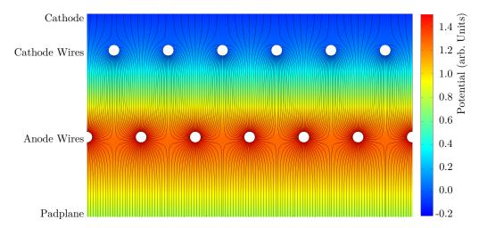
**Figure I.2:** Exemplary field configuration in a MWPC. The color code represents the potential while the field lines are illustrated in black.
