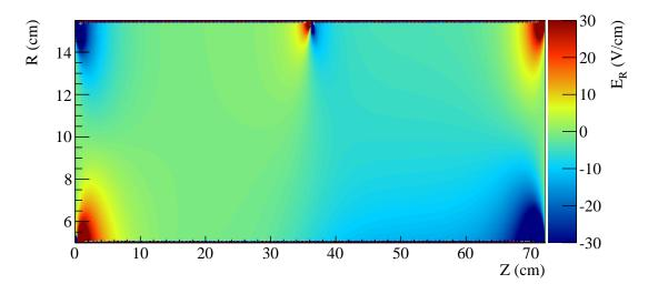
**Figure VII.6:** Radial component of the TPC drift field calculated with FEM taking field distorting effects into account. The radial field component should be zero throughout the TPC in the ideal case.
