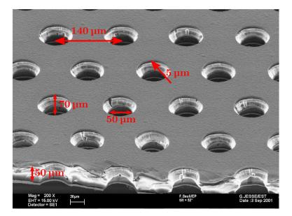
Figure II.13: A microscope image of a "standard" GEM foil with all specific dimensions.
