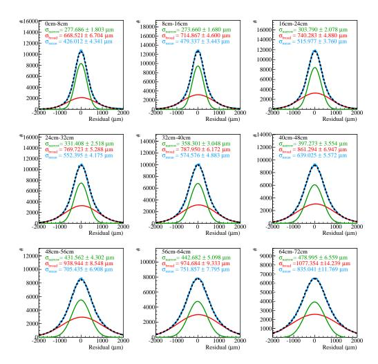
Figure D.1: Residual distributions with fits without any corrections in U direction.
