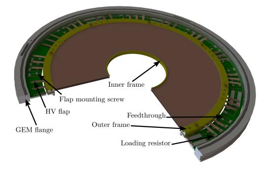
Figure II.12: Cut CAD drawing of the GEM flange.
