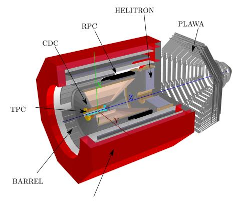
Superconducting 0.6 T Solenoid Magnet
