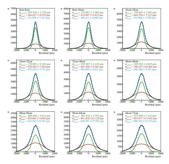
Figure D.9: Residual distributions with fits without any corrections in X direction.
