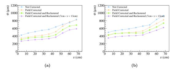
**Figure VIII.9:** Width of the residual distributions as a function of z and for several applied corrections. The residual components in the u and v directions thet define the virtual detector plane are shown in panel a and b respectively. The additional violet distribution is obtained when a cut on the radial position of the cluster is applied, to remove the remaining influences of the field distortions. The lines between the data points are drawn for a better visibility.
