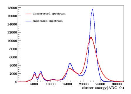
Figure VII.2: Krypton spectrum recorded with the GEM-TPC at a gain of  $\approx 2000$  with an Ar/CO<sub>2</sub> 90/10 drift gas. The uncorrected spectrum is depicted in red, while the blue spectrum is obtained after three iterations of gain equalization [61].
