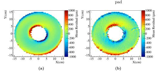
**Figure VII.9:** Mean x-component of the residual as a function of the cluster position in the xy plane obtained from a simulation taking the calculated distortions into account (a) and from a measurement of cosmic muons (b).
