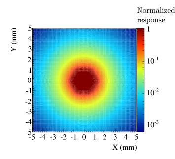
Figure VII.16: The normalized pad response as a function of the start position of the electron cloud.
