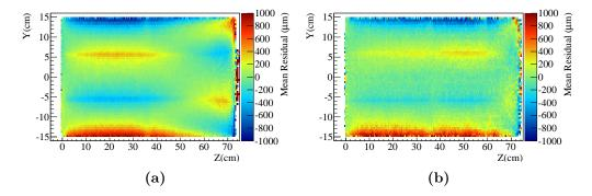
Figure VII.10: Mean x-component of the residual as a function of the cluster position in the yz plane obtained from a simulation taking the calculated distortions into account (a) and from a measurement of cosmic muons (b).
