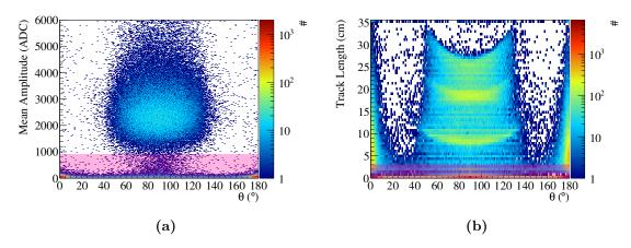
Figure VIII.3: Mean cluster amplitude and track length as a function of the inclination angle  $\theta$ . The pink shaded area illustrates the cuts. For details see text.
