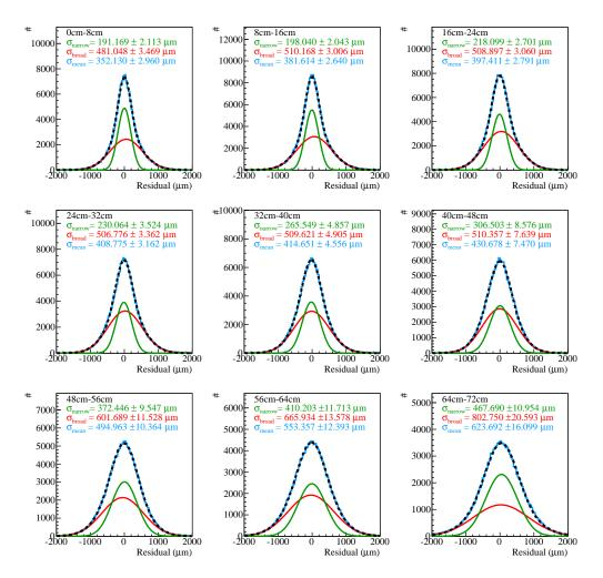
**Figure D.8:** Residual distributions with fits with field correction and reclustering and additional cut of the radial cluster position in V direction.
