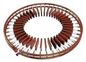
Figure II.26: The setup for the cooling water distribution as it was used in the first step of the simulations. The blue coin represents the inlet of cold water and the red one the outlet.
