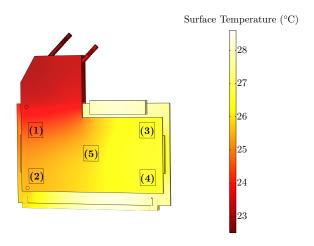
Figure II.28: Simulated surface temperature distribution of one front end card. The five rectangles indicate the measurement positions.
