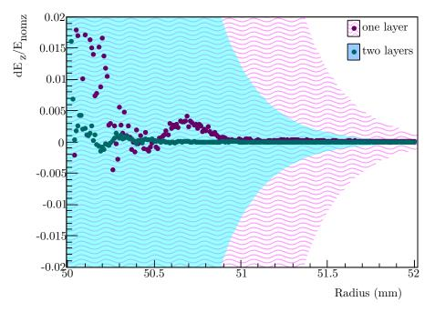
**Figure II.8:** Average deviation from the nominal drift field as a function of the radius. The averaging is done along lines of constant radius. The magenta dotted curve shows the case with only one layer of field strips, while the cyan dotted curve shows the two layer case. The colored bands correspond to one standard deviation.
