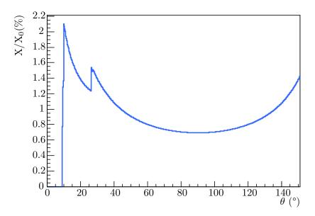
**Figure II.6:** Radiation length of the GEM-TPC calculated along tracks originating from the target position as a function of their polar angle.
