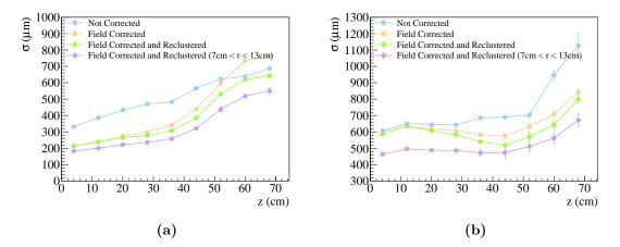
**Figure VIII.10:** Width of the residual distributions as a function of z and for several applied corrections. The component of the residual in x direction of the virtual detector plane is plotted in panel (a) and in z direction in panel (b). The additional violet distribution is obtained when a cut on the radial position of the cluster is applied, to remove the remaining influences of the field distortions. The lines between the data points are drawn for a better visibility.
