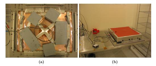
**Figure II.18:** Image (a) shows a GEM foil inside the stretching tool with the frame and glue already applied. Led weights are distributed on a frame, which applies the pressure only on the frame. The cable with the metal end is the temperature sensor for the temperature controller. The heating hood with the silicon heating pad (red) and the temperature controller (little grey box) put on top of the stretched and weighted foil is shown in the photograph (b).
