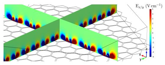
**Figure VII.14:** The induction field between the last GEM foil and padplane calculated with COMSOL<sup>®</sup>. Shown are the slices through the setup with the field component in x direction and y direction plotted along the x- and the y-axis, respectively.
