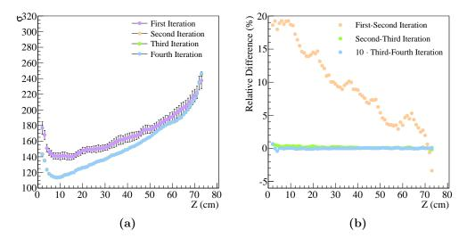
**Figure VI.19:** Panel (a) shows the evolution of the track point to Monte Carlo point residual for several parameter fit iterations. The width of the residual distribution is plotted as a function of the z position. The points for the second and third iteration are covered by the points of the fourth iteration, since the differences are already below 1% for these as one can see in panel (b) where the relative difference between consecutive iterations is plotted.
