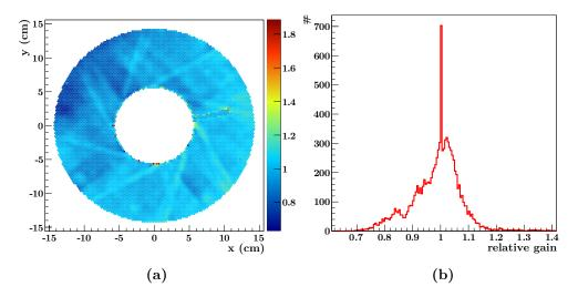
**Figure VII.3:** Panel (a) shows the equalization factor as a function of the pad position. The sector boundaries of the GEM foils are visible as bright iris shaped lines. The right panel shows the distribution of all equalization factors. The high peak at 1 comes from a dead FE chip which equalization factors were set to 1. The distribution is centred at one with a RMS of 0.09.
