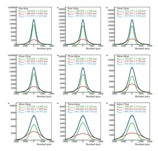
**Figure D.3:** Residual distributions with fits with field correction and reclustering in U direction.
