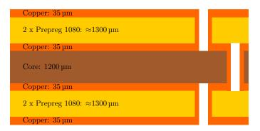
Figure II.21: The layer stacking of the padplane with their individual thickness. The placement of the vias to achieve gas tightness is also illustrated.
