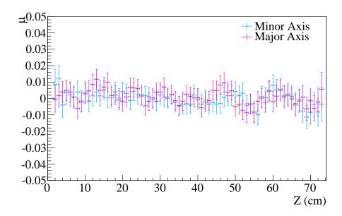
Figure VI.13: Mean position as a function of z for the pull distribution calculated with the fit and the parametrized covariance matrix.
