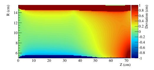
Figure VII.8: Radial deviation from the straight drift as a function of the starting point.
