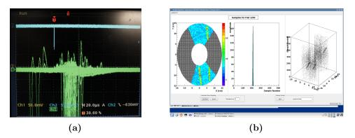
Figure IV.1: Examples of the first measured cosmic muons. The left panel shows a measurement with an analog readout (see text). The right panel shows one of the first recorded moun tracks (see text).
