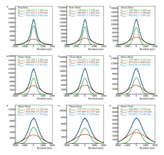
Figure D.6: Residual distributions with fits with field correction in V direction.
