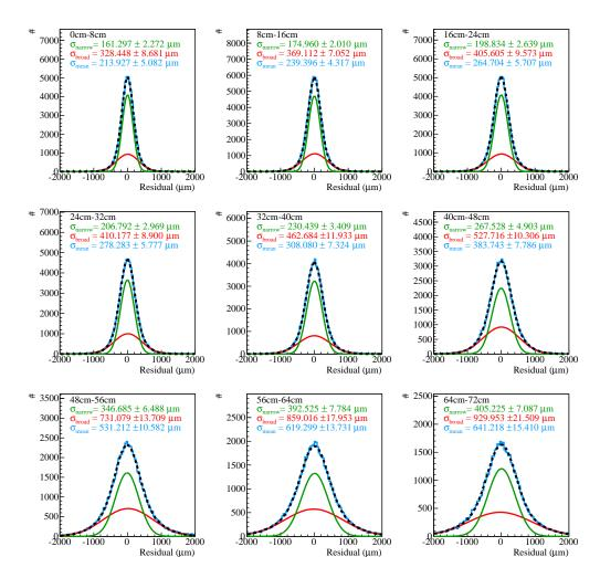
**Figure D.11:** Residual distributions with fits with field correction and reclustering in X direction.
