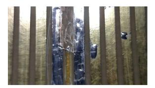
Figure II.3: The soldered connection of the two strip foils for the outer field cage.
