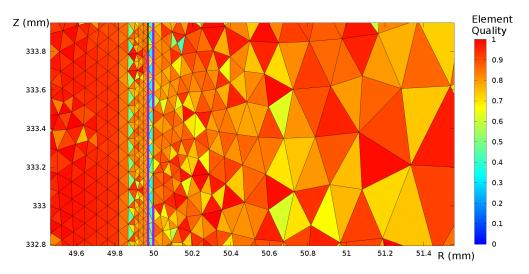
Figure VII.5: Closeup of the FEM mesh near the field cage strips. The strips are highlighted in violet and the color code represents the mesh element quality.
