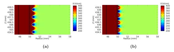
**Figure II.7:** The magnitude of the electric field near the field cage strips without (left) and with (right) the second strip layer. The gas volume begins at radius=50 mm.
