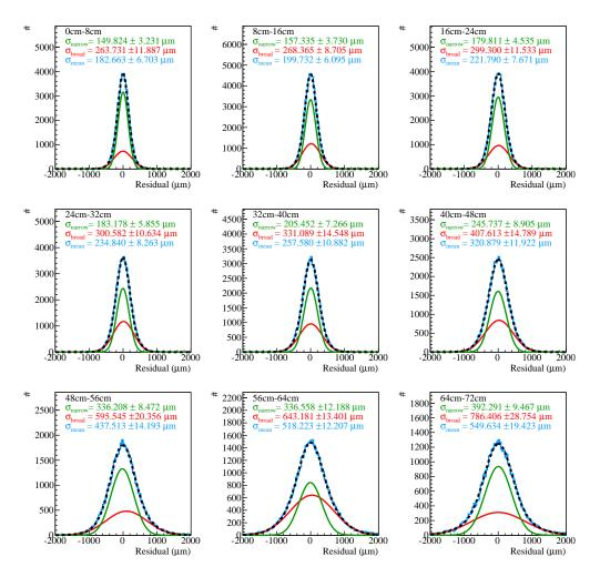
**Figure D.12:** Residual distributions with fits with field correction and reclustering and additional cut of the radial cluster position in X direction.
