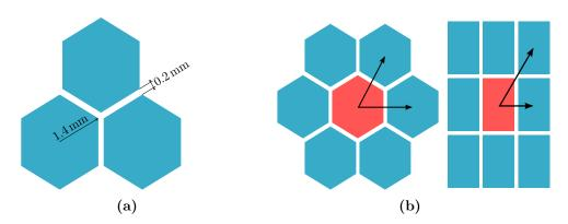
Figure II.19: The geometry, size and distance between pads is depicted in the left panel. The right panel shows a comparison of the distance to the next neighbors between hexagonal and rectangular pads [20].
