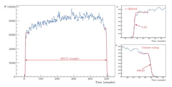
Figure VII.1: Occupancy as function of the time bin for drift velocity calculation with fitted step functions at both ends of the distribution. The measurement was done with a drift field of  $309.6 \,\mathrm{V \, cm^{-1}}$  and a  $\mathrm{Ar/CO_2} \, 90/10$  gas mixture.
