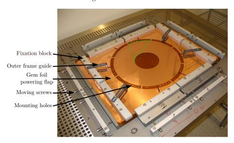
Figure II.17: A GEM foil in the stretching tool during framing. One of the eight sectors is marked by a green line.
