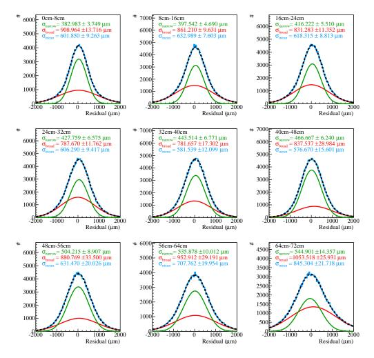
Figure D.14: Residual distributions with fits with field correction in Z direction.
