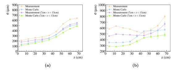
**Figure VIII.12:** Track point resolution for measurement and simulation as a function of the drift length. The left panel shows the distribution of the track point resolution along the x-coordinate while the resolution along the z-coordinate is depicted in the right panel.
