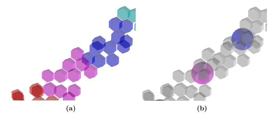
Figure VI.2: The pad hits are shown as hexagonal shapes with their height proportional to their amplitude. In the left panel only the pad hits already associated with a cluster (indicated by the colors) are drawn. The right panel shows the resulting clusters depicted as spheres.
