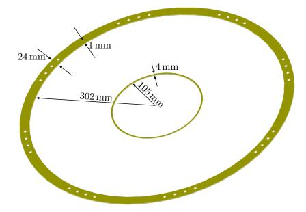
Figure II.16: The inner and outer frame for the GEM foils with their dimensions and the holes for installation on the GEM flange.
