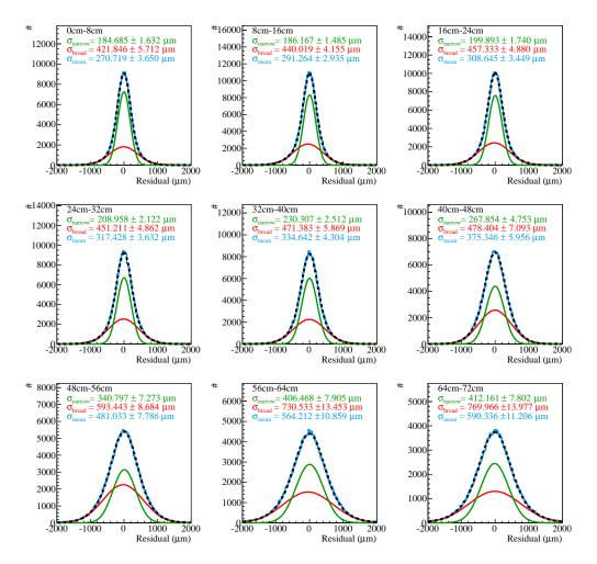
**Figure D.4:** Residual distributions with fits with field correction and reclustering and additional cut of the radial cluster position in U direction.
