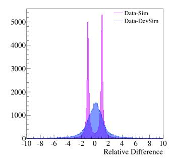
**Figure VII.11:** Relative difference of the x-component of the residuals between data and simulation. The magenta distribution was obtained with a simulation not taking into account the drift field distortion, while the blue distribution is extracted from a simulation with distortions.
