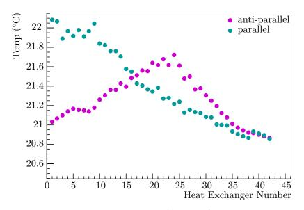
**Figure II.29:** Mean temperature at position 5 (Fig. II.28) as a function of the heat exchanger. The flow of the cooling liquid through each heat exchanger defining the temperature can be found in Fig. II.27.
