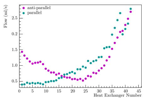
**Figure II.27:** Cooling liquid flow through the 42 heat exchangers for two different supply mechanisms.
