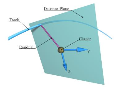
**Figure VI.5:** Virtual detector plane with the spanning vectors U and V for a space point hit. For the GEM-TPC a space point is a cluster.
