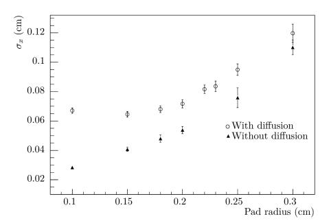
**Figure II.20:** Cluster residual width along x as a function of the pad radius, with diffusion (open circles) and without (full circles). A 2 T magnetic field was taken into account [21].
