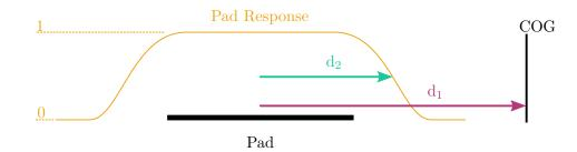
Figure VII.18: Schematic view of the calculation of the expected distance. The orange curve indicates the pad response function. The arrows represent the distance between pad and center of gravity (violet,  $d_1$ ) and the expected distance (turquoise,  $d_2$ ).  $d_2$  is defined by the pad response function and the fraction of the total amplitude of the pad in question.
