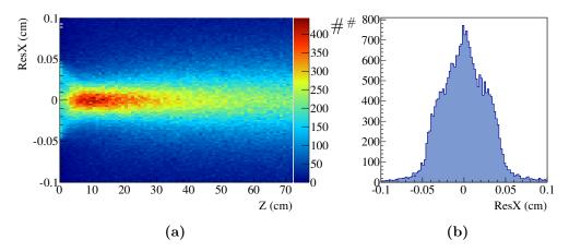
**Figure VII.17:** Residuals to the Monte Carlo point along the x-axis as a function of the drift length for uncorrected cluster positions are shown in panel (a). Panel (b) shows a projection of the first three bins of the drift length. One can clearly see the signature of the finite pad size effect.
