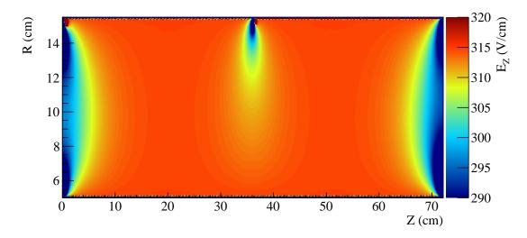
**Figure VII.7:** Longitudinal component of the TPC drift field calculated with FEM taking field distorting effects into account.
