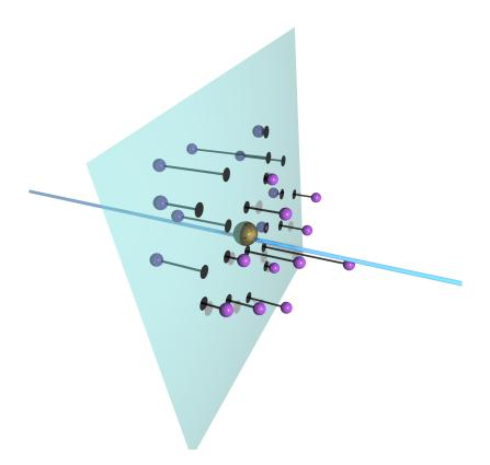
**Figure VI.9:** Visualization of the projection of the pad hits (purple spheres) onto the detector plane (turquoise plane). The projections are marked as black circles. The resulting cluster (golden sphere) and the track (turquoise line) are also shown.
