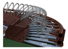
(b) Closeup view of the cut through one front end card.
