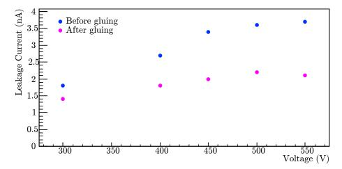
Figure II.15: The leakage currents of one GEM foil before (blue) and after (pink) the framing process.
