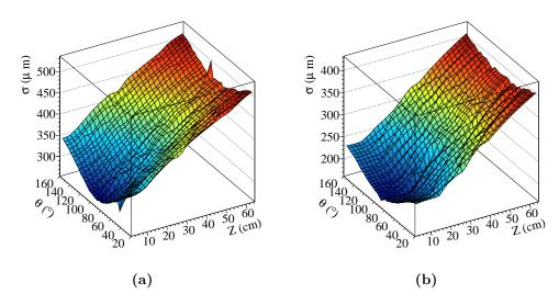
Figure VI.15: Cluster position uncertainty as a function of the track inclination angle and the z position of the cluster. The left panel shows the value of the uncertainty along the first eigenvector, the right panel along the second.
