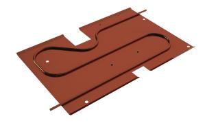
Figure II.30: CAD rendering of the ADC cooling sheet metal.
