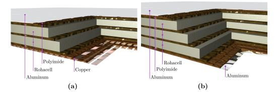
**Figure II.5:** Schematic view of the layer stacking for the field cage (a) and the cathode (b). The glue in between all layers is not explicitly shown and the thickness of each layer is scaled arbitrarily for a better visibility. For the materials and exact layer thicknesses see Tab. II.1.
