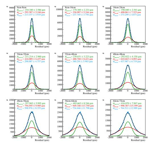
Figure D.10: Residual distributions with fits with field correction in X direction.
