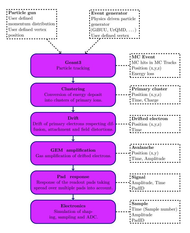
**Figure V.1:** Flowchart of the steps in the simulation. The violet boxes represent the simulation steps while the dashed boxes illustrate the object produced in each step with their main characteristics. The two dashed boxes on top show the possible input generators.
