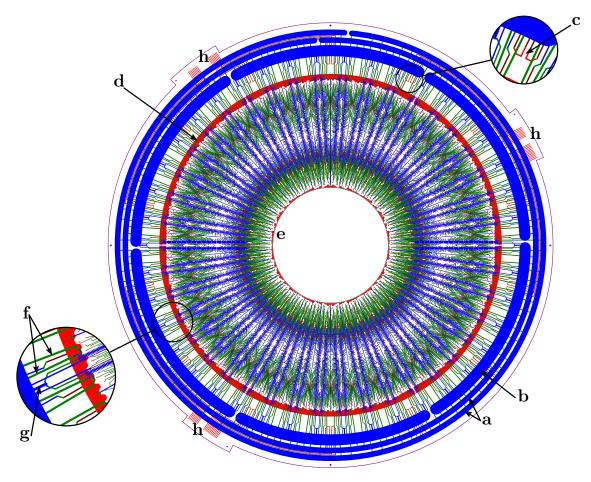
Figure II.22: The layout of the padplane. The pads are for a better visibility of other features not shown. For details see text.
