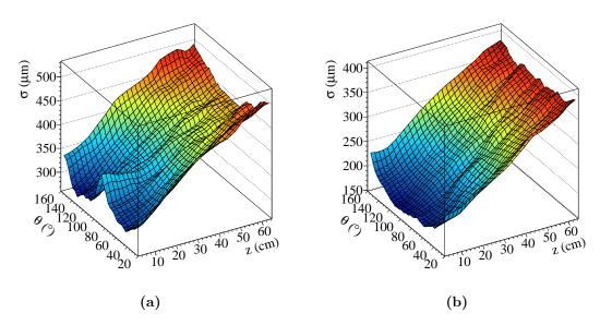
**Figure VI.11:** Width of the residual distribution as a function of the polar angle  $\theta$  and the z position for the major (a) and minor (b) axis. For details see text.
