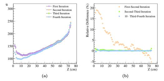
**Figure A.1:** Panel (a) shows the evolution of the v-component of the track point to Monte Carlo point residual for several parameter fit iterations. The width of the residual distribution is plotted as a function of the z position. The points for the second and third iteration are covered by the points of the fourth iteration, since the differences are already below 1% for these as one can see in panel (b) where the relative difference between consecutive iterations is plotted.
