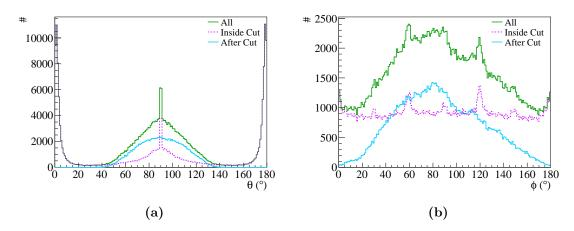
Figure VIII.5: Angular distributions of the tracks before any cut (green), after applying the cuts (blue) and the tracks inside the cuts (violet). Panel (a) corresponds to the polar angle and panel (b) to the azimuthal angle of the cosmic muon tracks.
