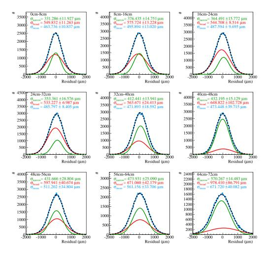
Figure D.16: Residual distributions with fits with field correction and reclustering and additional cut of the radial cluster position in Z direction.
