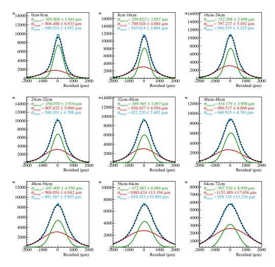
Figure D.5: Residual distributions with fits without any corrections in V direction.
