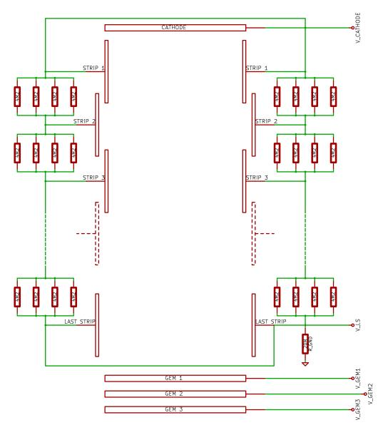
Figure II.4: Schematic of the electric design of the field cage.
