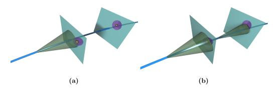
Figure VI.6: Illustration of the working principle of the Kalman filter track fitting. The left panel shows the first step of the fitting procedure. In the right panel the second step is shown, where the uncertainty cone of the track extrapolation is already much smaller, since the track extrapolation obtained in the first step as well as the information of the next hit is taken into account.
