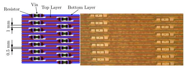
**Figure II.2:** The left side shows a schematic view of the field cage strips with the resistors of the resistor chain and the connections between top (red) and bottom (blue) layer. On the right side a photograph of the field cage strips is shown.
