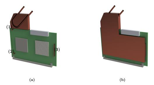
Figure II.23: CAD rendering of one front end card with its cooling components. Panel (a) shows the front end card with partially removed cooling system. One copper plate for heat transfer as well as one heat conducting pad between the copper plate and T2K chips (grey squares) has been removed. (1), (2) and (3) indicate the soldering positions of the copper plate. The front end card with the complete cooling system attached is depicted in panel (b).
