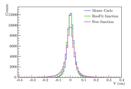
**Figure VI.16:** Position of the mean in v direction from the fit of the free function (magenta), the RooFit function (green) and the Monte Carlo value (blue).
