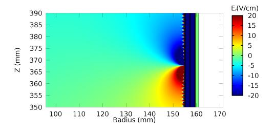
Figure II.10: Radial component of the electrical field inside the field cage at the outer rim near the position where the two strip foils had to be soldered together.
