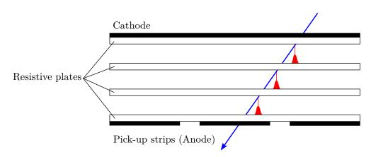
**Figure III.2:** Schematic of a multi-gap multi-strip RPC with four gaps. Only the electrons from primary ionization caused by a particle traversing the detector (blue) which are close to the resistive plates gain enough energy to perform avalanche multiplication (red).
