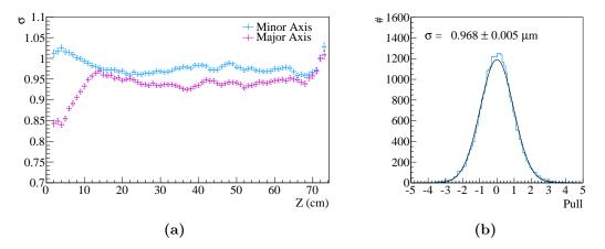
Figure VI.12: Pull distributions from cluster uncertainties calculated with the parametrized covariance matrix. The left panel shows the resulting width of the pull distribution as a function of the z position along the directions of the eigenvectors from the covariance matrix. The pull distribution at a z position of 33 cm for the pull distribution along the major axis together with the Gaussian fit is exemplary shown in the right panel.
