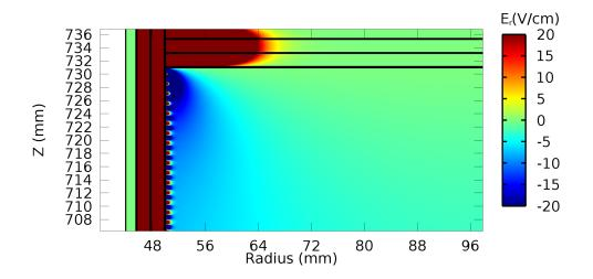
Figure II.9: Radial component of the electrical field inside the field cage close to the cathode.
