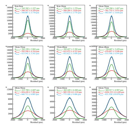
Figure D.2: Residual distributions with fits with field correction in U direction.
