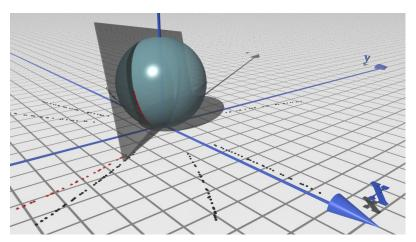
Figure VI.3: Example of the Riemann transformation with a circular track originating from charged pions. The tracks have been scaled to better fit the Riemann sphere. The transformed points of one track (red) together with the resulting plane are also shown. [41]
