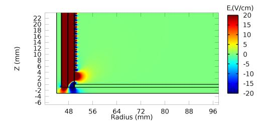
Figure II.11: Radial component of the electrical field inside the field cage close to the anode.
