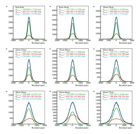
**Figure VIII.11:** The individual z-bin distributions of the residuals in x direction from the data set with all corrections applied and an additional cut on the radial cluster position. The distributions are fitted with the sum of two Gaussian functions depicted by the black dashed line with the individual components visible in red and green. The mean width, which is plotted in Fig. VIII.10(a) is calculated with VIII.2.
