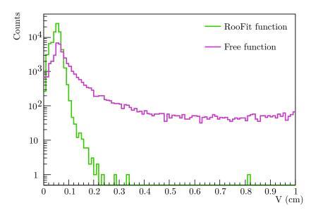
Figure VI.17: Error of the mean position in the v direction for the free function (magenta) and the RooFit function (green).
