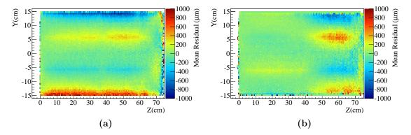
**Figure VIII.7:** X component of the mean cluster to track residuals as a function of the position projected onto the yz plane. Panel (a) shows the uncorrected data, while the distribution in panel (b) is obtained after the correction with the distortion map as explained in Sec. VII.3.
