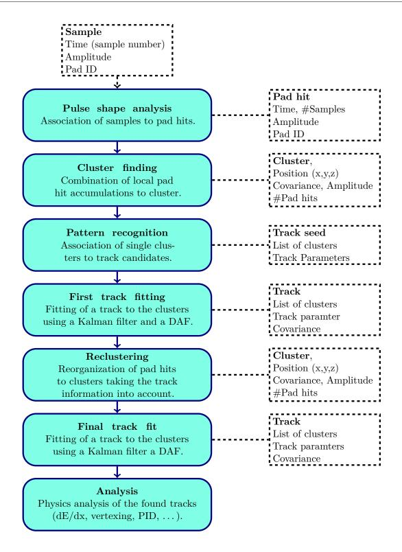
Figure VI.1: Schematic overview of the sequence of reconstruction algorithms. The turquoise boxes depict each reconstruction step with the entities they generate and their main properties in dashed rectangles.
