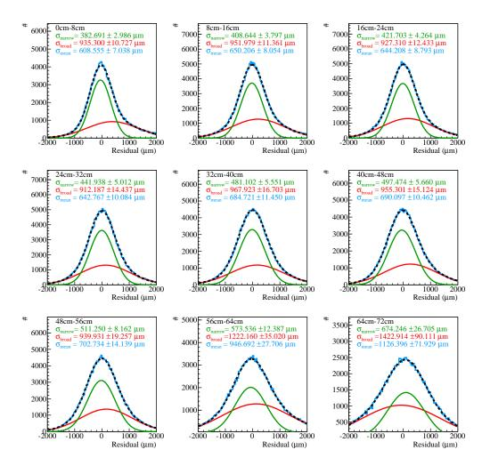
Figure D.13: Residual distributions with fits without any corrections in Z direction.
