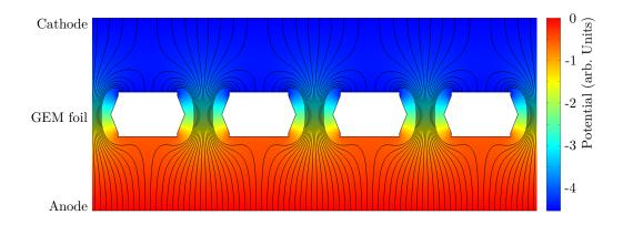
**Figure I.3:** Exemplary field configuration of a GEM foil. The white regions show the cross section of the GEM foil, the field lines are illustrated in black while the color code visualizes the potential.
