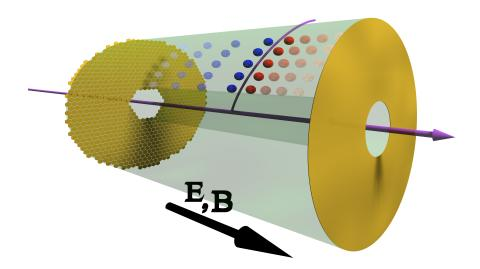
Figure I.1: Basic working principle of a TPC. For details see text.
