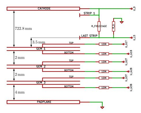
Figure II.14: Electrical schematic of the GEM stack and the field cage. The field cage resistor chain and strips are condensed into the single resistor  $R_{\text{field cage}}$ .
