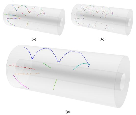
**Figure VI.4:** In panel (a) all pad hits recorded in an event from an experiment with a pion beam are shown. The colors already indicate to which cluster they belong. The active volume of the GEM-TPC is illustrated in light gray. Panel (b) shows the resulting clusters. The found tracks from the pattern recognition with the corresponding clusters are visible in panel (c).
