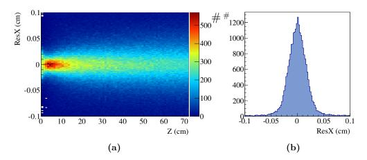
**Figure VII.19:** Residuals to the Monte Carlo point along the x-axis as a function of the drift length for corrected cluster positions are shown in panel (a). Panel (b) shows a projection of the first three bins of the drift length.
