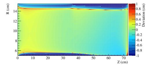
Figure B.2: Deviation along the drift direction as a function of the starting point.
