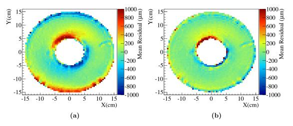
Figure VIII.6: X component of the mean cluster to track residuals as a function of the position on the padplane. Panel (a) shows the uncorrected data, while the distribution in panel (b) is obtained after the correction with the distortion map as explained in Sec. VII.3.
