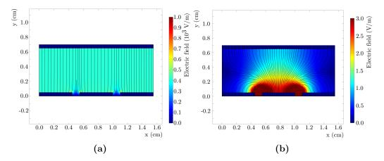
**Figure VII.12:** Figure (a) shows the magnitude of the electric field with the resulting field lines. The top electrode is set to 250 V, while the three bottom electrodes are on zero potential. In figure (b) one can see the resulting weighting field for the central bottom electrode.
