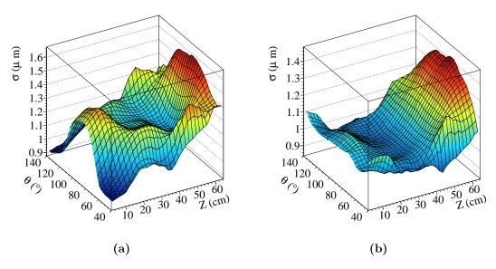
Figure VIII.8: Distribution of the pull distribution width as a function of the track inclination angle  $\theta$  and the cluster z position for the major axis (a) and the minor axis (b). The widths are obtained from Gaussian fits to the pull distributions.
