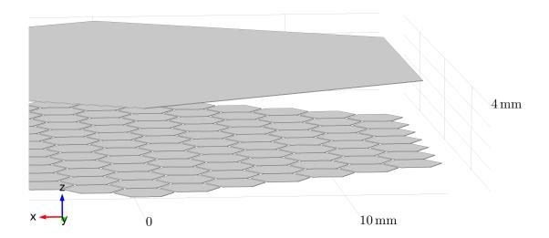
**Figure VII.13:** The geometrical setup of the COMSOL<sup>®</sup> model for the pad response calculation.
