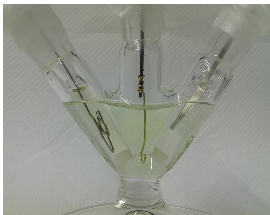
Figure 8.3: Three electrode glass setup: platinum counter electrode and gold working electrode in EC:DEC (1:1, wt%) electrolyte containing \text{LiClO}_4 concentrations from 0.1 \times 10^{-3} to 2 M and 50 \mu\text{M} ferrocene and lithium reference electrode in same electrolyte without ferrocene.
