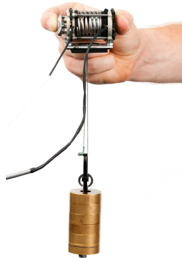
Figure 2.7: Second version of the Grip Perturbator held in a pinch grasp with attached weights (reproduced from [HMvdS13]).
