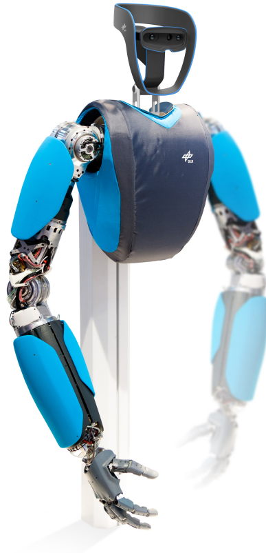
Figure 1.6: The DLR Hand Arm System — 26 joints with variable stiffness, 19 for the hand, and 7 for the arm.
