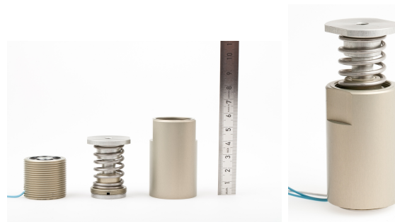
Figure 2.2: First version of the Grip Perturbator (reproduced from [HLU + 11] ©2011 IEEE). — This version is used within section 2.2; from left to right: electromagnet, moving part, rigid part, whole.
