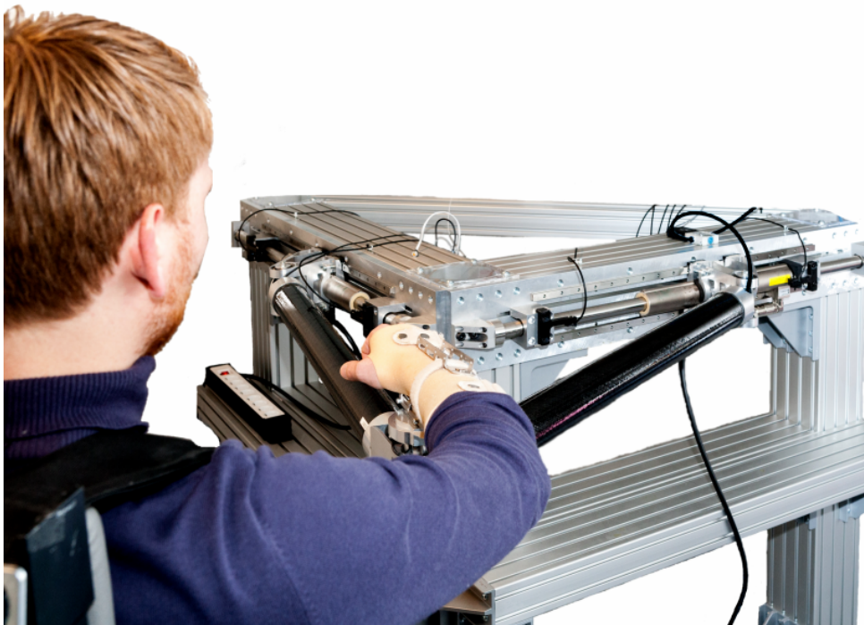
Figure 3.3: Manipulandum in real (reproduced from [HGvdS15] ©2015 IEEE). — The subjects are attached via a plastic cuff to the end-effector. In order to ensure subject's safety, the connection is realized using a permanent magnetic clutch in order to allow subjects to decouple in each experimental situation.
