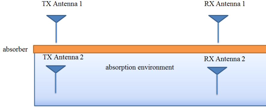
Figure 3.6: 2×2 MIMO system with absorber and absorption environment.
