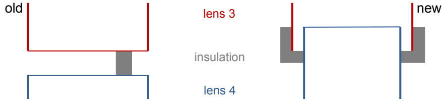
Figure 4.3: Cross-sectional, principal sketch of the transition between 'lens 3' and 'lens 4' (as defined in figure 4.2) in the original (left) and new (right) design, where the electric field in the lens system is not disturbed by a gap.
