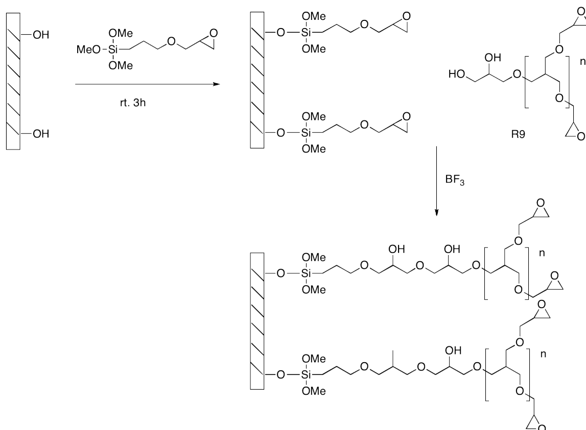
Fig. 16: Schematic description of silanization of glass wall with GOPTS and its reaction with R9
