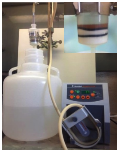
Fig. 43: Setup of improved MAF(Big) with O-ring and stacked-disk
