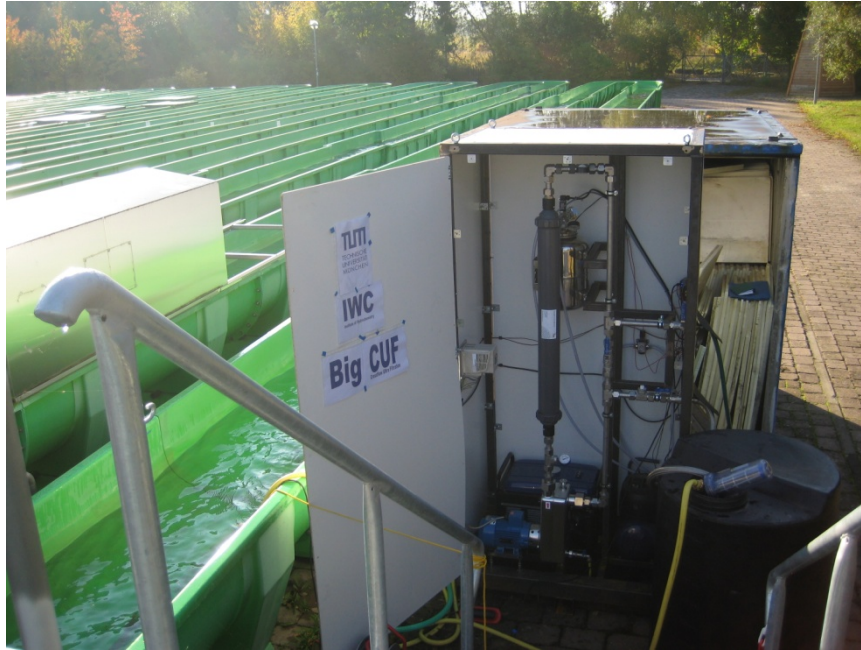
Fig. 34: UF instrumentation at the artificial stream and pond simulation system in Marienfelde, Berlin.
