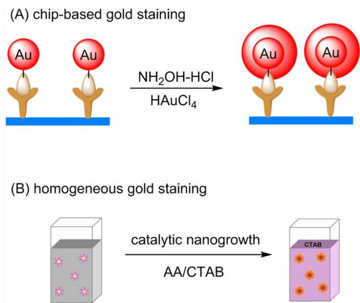
**Figure 3.14** Schematic illustration of chip-based (A) and homogeneous gold staining (B).
