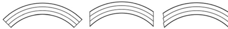
Fig. 2-6 Laminate bending modes Kirchoff bending (left), with intra-ply shear (center) and a combination with inter-ply shear (right) [12]
