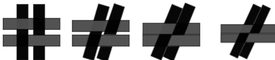
Fig. 2-2 Different states in shearing a woven fabric Initial state; sheared state; sheared up to locking angle; further shearing leading to fiber jamming (from left to right)
