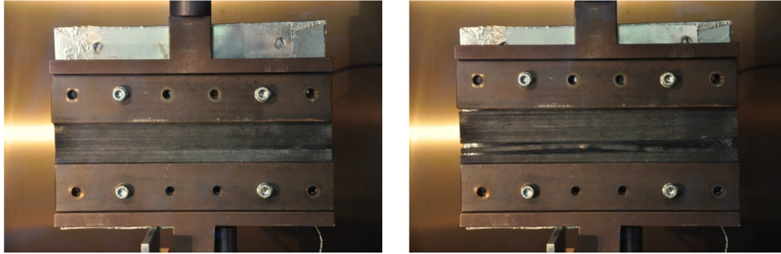
Fig. 4-30 LCC tension test with 4-layers laminate Initial state (left); final state after rupture (right)
