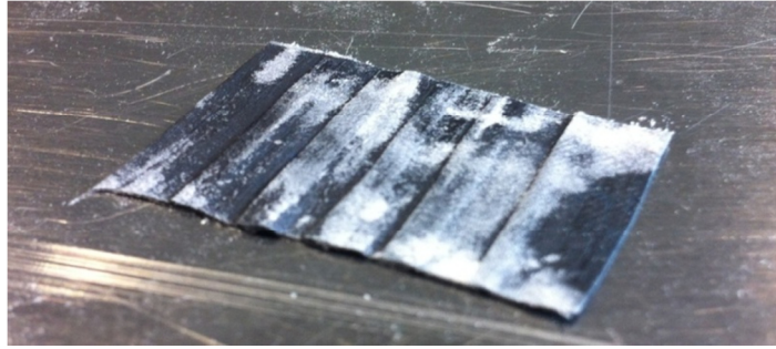
Fig. 4-22 90°-specimen used for the bending test
