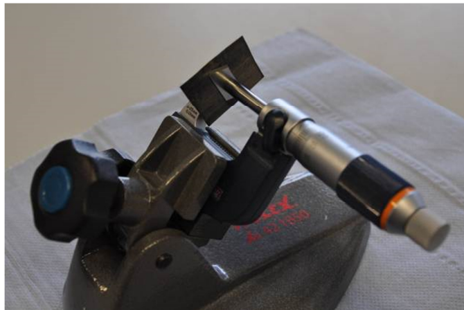
Fig. 4-34 Thickness measurement using a micrometer The razor blades are used to avoid a compression of the specimen
