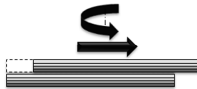
Fig. 2-14 Rotational and translational motion between plies [19]
