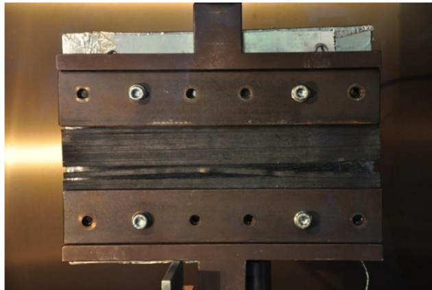
Fig. 5-4 Tensile test of 4-layers AFP material when rupture started
