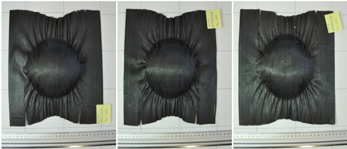
Fig. 6-11 Top view of three preforms from the hemisphere forming experiments
