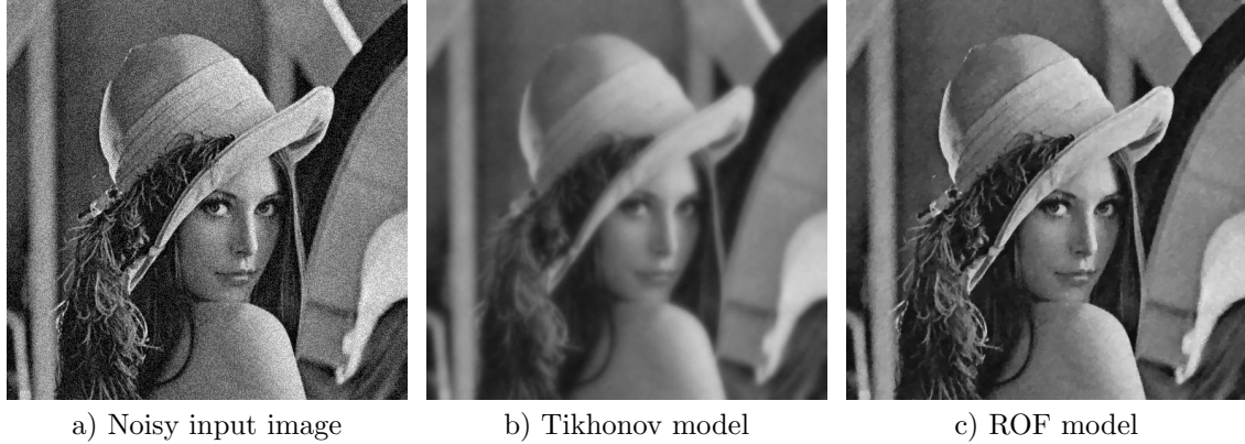
Figure 3.2: TV regularization preserves edges. The noisy input image a) is denoised by using b) the Tikhonov model and c) the ROF model with \lambda = 30 . While the ROF model preserves the edge information in the recovered image, the Tikhonov regularization technique not only removes the noise but also blurs prominent structures such as edges.
