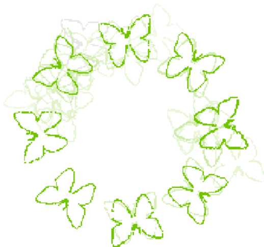
Figure 4.25: Robustness to pose variations. Independent of their location and rotation, all butterflies are found. Correct fits appear more often and have a lower energy.
