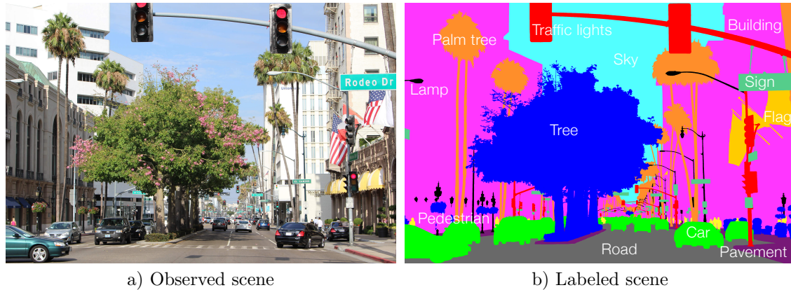
Figure 1.1: Semantic labeling and interpretation of a typical road traffic scene. “Multiple cars are driving on the road guided by signs, road markings and traffic lights. Pedestrians are walking on the pavements between street lamps and palm trees.” Humans are confronted with such scenes in their daily life. Drivers as well as pedestrians have to analyze the road traffic and interpret the observed scene to ensure road safety.
