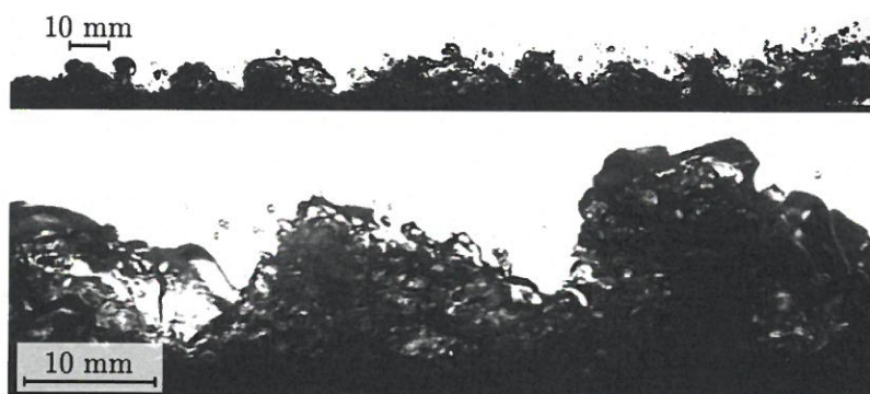
Figure 4. Vapor structure over a larger area (above) and in detailed recording of the middle section (below), both for fully developed nucleate boiling at inlet subcooling of 9 K and flow superficial velocity of 0.6 m/s (images not synchronous). The images are rotated by 90 degrees, i.e. the inlet is on the left side.
