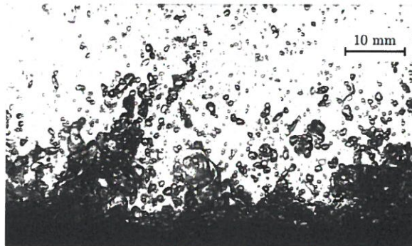
Figure 8. Vapor Structure at CHF(-) for with an orifice insert for a subcooling of 9 K and v_s=0.6\text{ m/s} (image rotated by 90^\circ ). The flow without inserts is shown above in Figure 4.
