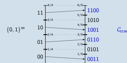
Figure 2: Diagram of a constant composition arithmetic encoder with  $P_{\tilde{A}}(0) = P_{\tilde{A}}(1) = 0.5$ ,  $m = 2$  and  $n = 4$ .
