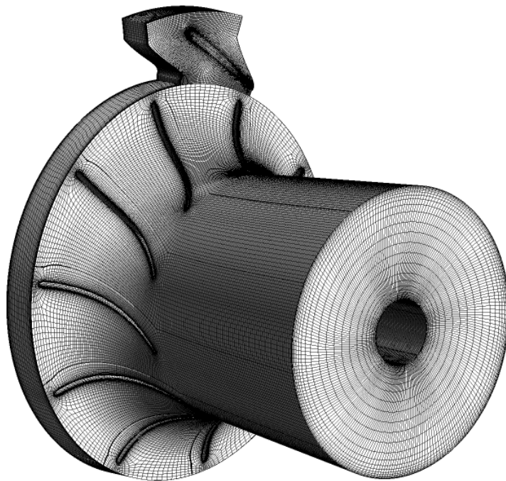
Figure 5.5: Control volume with one nozzle passage.
