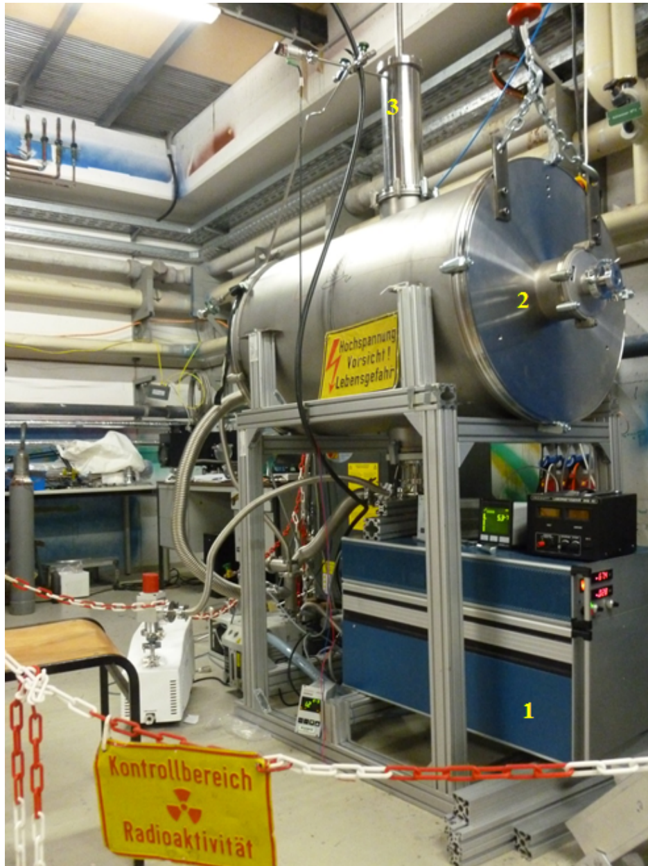
Figure 2.79: Test setup during the “training” of the high-voltage equipment: 1. High-voltage source ( U=0-150 kV); 2. Vacuum chamber; 3. The chamber for the electronic equipment.
