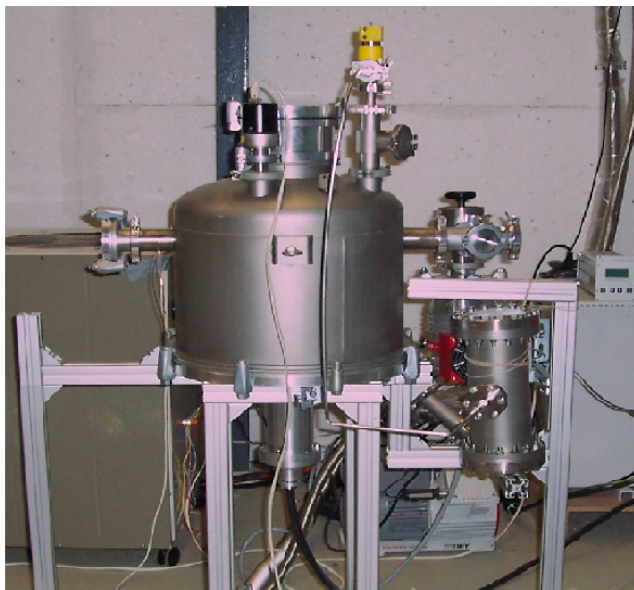
Figure 2.34: Test equipment: 1) Vacuum chamber (vessel V=50 l); 2) Gas cylinder with ^{129}\text{Xe} ( V=3 l); 3) Vacuum sensor.
