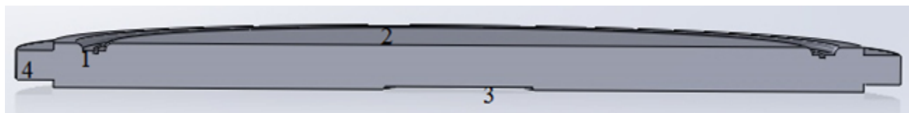
Figure 2.73: High-voltage electrode (SolidWorks simulation): 1. Groove for insulator ring. A second groove inside this groove is for an O-ring; 2. Flat part of the electrode, designed to provide a uniform electric field within the neutron chamber; 3. Circular recess for the high-voltage connector; 4. The outer part of the high-voltage electrode with slots for clamps for fixation. The thickness of the HV electrode is 30 mm, the diameter is 600 mm. The drawing of the high-voltage electrode is shown in Fig. A.6.1, see App. 6.
