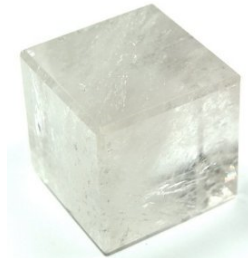
Figure 2.28: The quartz crystal cube (with the side of 20 mm), which was used for the measurement.
