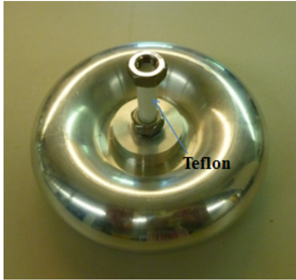
Figure 2.48: The ground electrode with a fixed insulator (Teflon rod).
