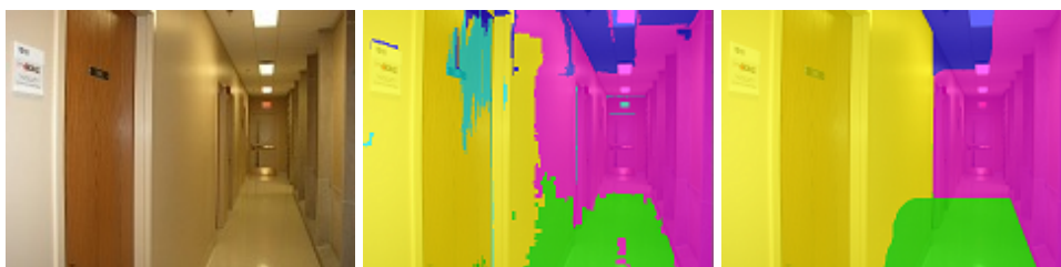
Figure 5.5: Failure case for the five regions layout. Since the data term ( center ) is very misleading, the ordering constraints do not allow to recover the desired solution. From left to right: input image, data term, result with ordering constraints.
