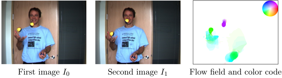
Figure 8.11: Optical flow with large displacements. When employed for optic flow, the proposed method can successfully capture large displacements without the need for coarse-to-fine approaches, since a global optimization is performed over all labels. In contrast to existing methods, our solution is within a known bound of the global optimum.
