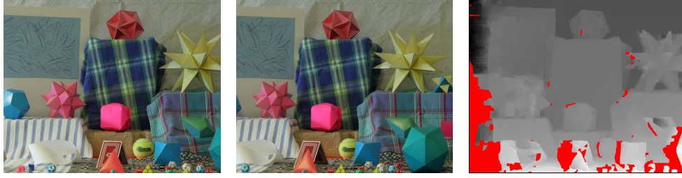
Figure 8.9: Displacement with occlusion maps. The proposed method can be employed to simultaneously optimize for a displacement and an occlusion map. This problem is also too large to be solved by alternative relaxation methods on current GPUs. From left to right: Left and right input image I_L and I_R , and computed disparity and occlusion map; red areas denote occluded pixels.
