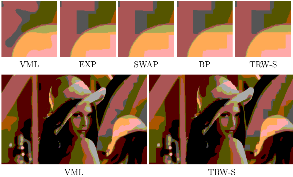
Figure 8.6: Comparison of the algorithms. Closeups of 4 \times 4 \times 4 RGB label segmentations ( top ) using different algorithms reveal a typical problem of discrete approaches: they exhibit a preference for horizontal and vertical region boundaries since they penalize an l^1 -distance instead of the correct Euclidean length [68, 143]. The error can be reduced by increasing the neighborhood connectivity, but only at extremely high costs of memory and computation time. Overall, these metrication errors lead to blocky and visually less pleasing segmentation results ( bottom ).
