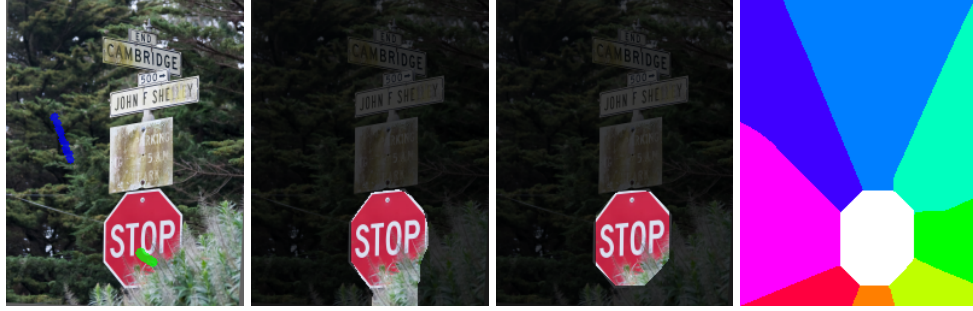
Figure 5.11: Convex shape prior. Beyond existing approaches, the proposed framework allows to model priors on convex shapes. From left to right: input image with user scribbles, Potts partitioning, partitioning using the convex shape prior, prior encoding. The prior is modeled by a n -gon, here an octagon, with edges pointing in all directions.
