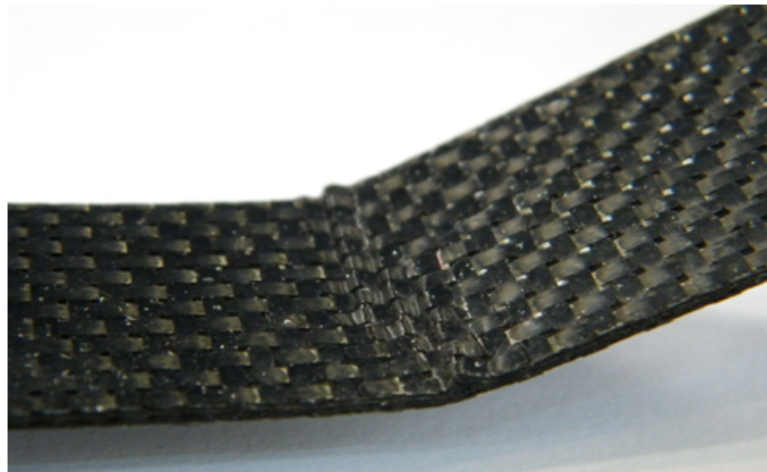
Figure 5.5.: Microbuckling on a CFRS laminate
