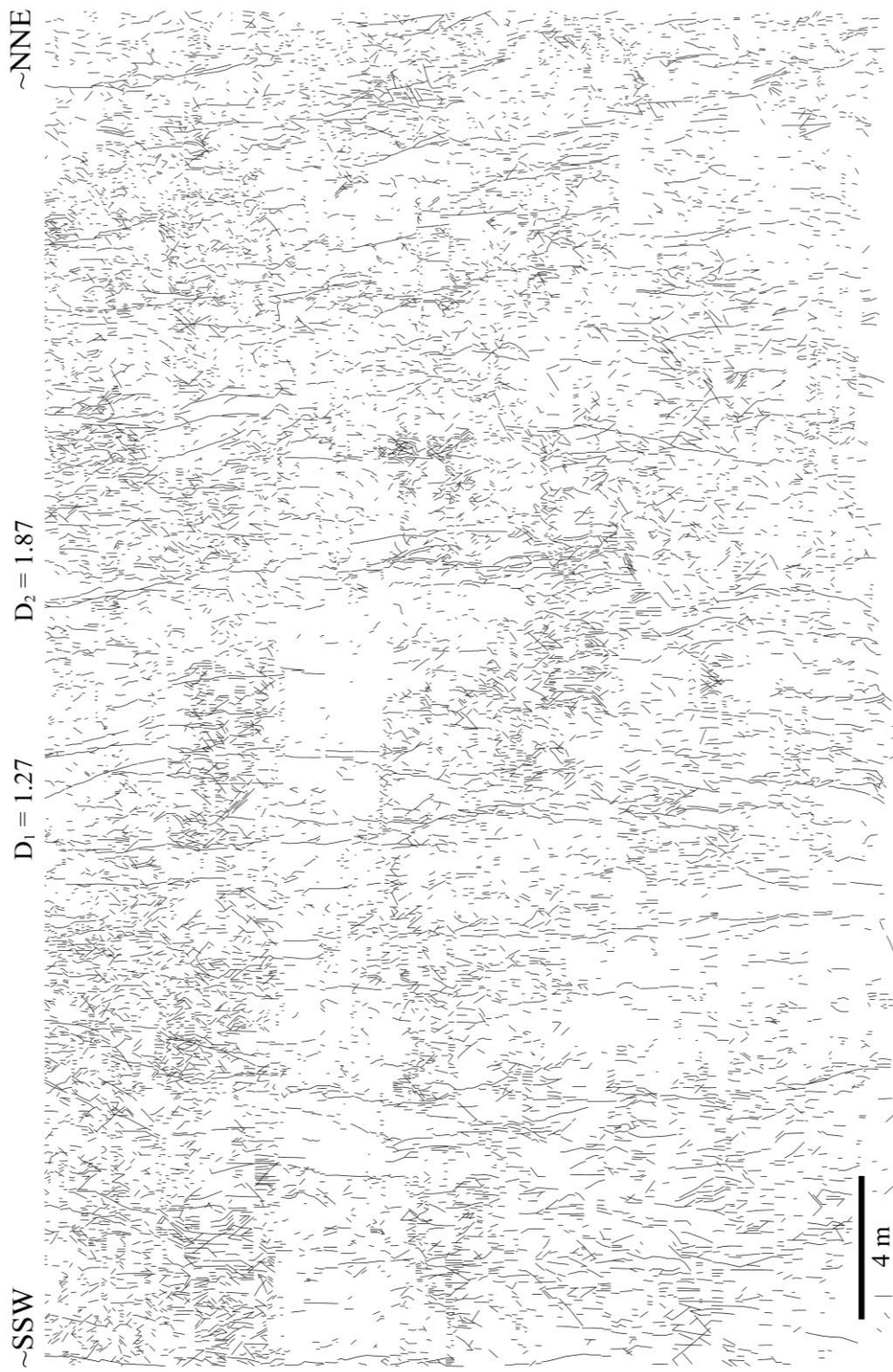
Figure App. 1.2: Binary image of fracture patterns in a vertical section in the Solnhofen quarry (~30 km E of the crater centre) after merging, digitizing and processing of 3 high-resolution digital field photographs. The vertical section is oriented at ~N20E. One pixel in the binary image = 1.98 mm on the ground. The fractures were manually drawn on the basis of the digital field photographs. Fractality ( D -value) of the fracture patterns is quantified by 2D box counting using the Benoit software. Two fractal dimension values are indicated by D_1 and D_2 (on top).
