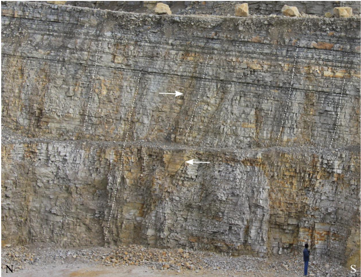
Figure 4.3: Approximately N–S oriented vertical section in the Eireiner quarry (location in Fig. 4.4) with centimetre- to 1-decimetres-thick bedding in Malm limestone, slightly inclined to the south. Zones of intense fragmentation (dashed lines) transect the bedding. These zones are typically several metres long and decimetres-wide and composed of shorter, irregular, centimetre-spaced fractures. In general, the zones are perpendicular to the bedding, regardless of bedding inclination. Locally, fractures show cm-wide opening (arrows).
