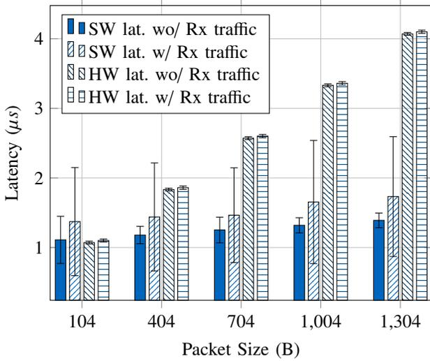
Fig. 5. SW and HW transmit latencies observed in experiment 1 and 2
