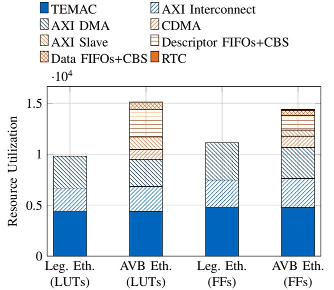
Fig. 8. Hardware resources used by the AVB Ethernet controller compared to a legacy controller
