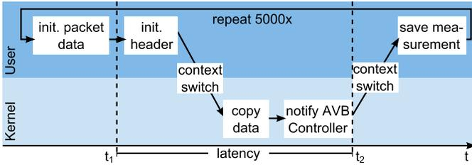
Fig. 4. Measurement flow to determine software latencies (Experiment 2)
