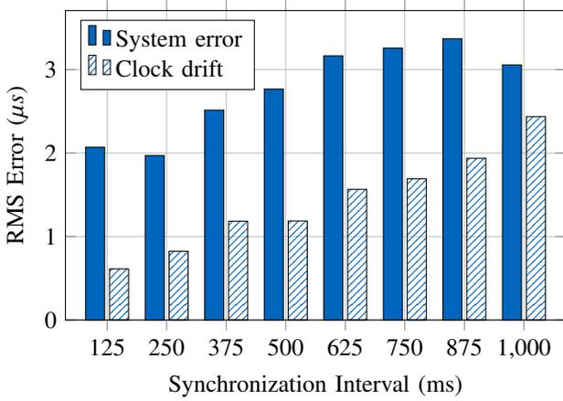
Fig. 7. Synchronization error from system non-idealities as well as clock drift in experiment 3
