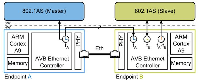
Fig. 6. Measurement setup to determine synchronization errors (Experiment 3)
