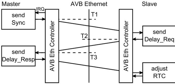
Fig. 2. Time synchronization between two endpoints using 802.1AS
