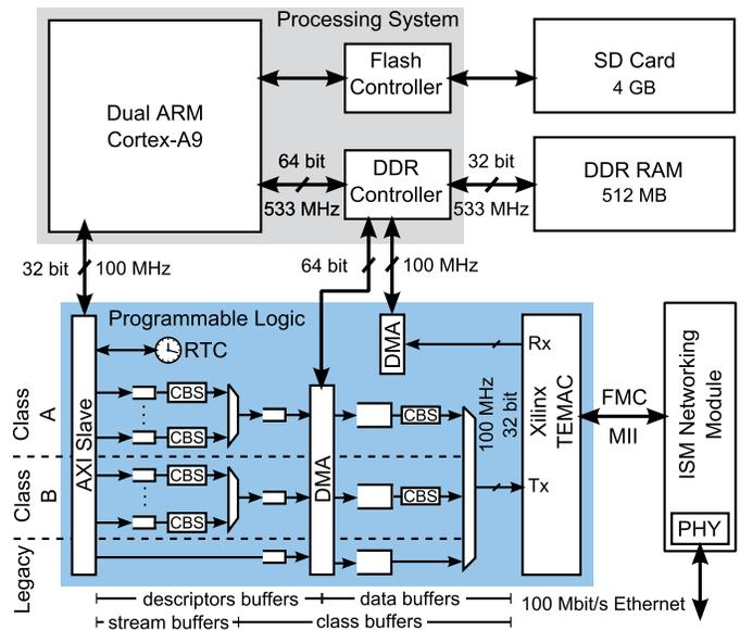
Fig. 1. System overview with detailed presentation of the AVB Ethernet controller implementation
