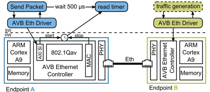
Fig. 3. Measurement setup to determine latencies within the AVB Ethernet controller (Experiment 1)
