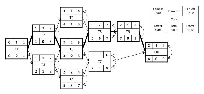
Figure 2-10: Determination of float time and critical path for the construction project introduced in Figure 2-1. Boxes: tasks, arrows: precedence relationships, dashed arrows: steps of the calculation, fat arrows: critical path, fat boxes: critical tasks.
