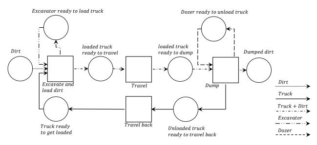
Figure 3-11: Earth moving process represented with an ACD
