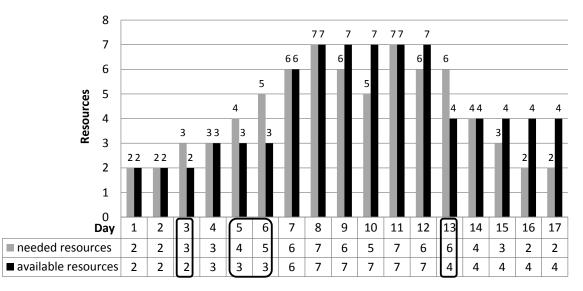
Figure 1-4: Diagram of the available and necessary resources of a short project (necessary resources: gray, available resources: black, resource limits exceeded: black box)
