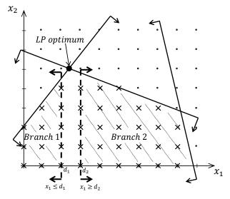
Figure 6-10: The branching process of the introduced IP problem combined with the cutting plane algorithm (B&C)
