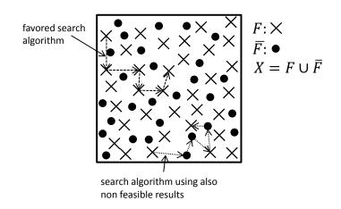
Figure 6-4: Different possibilities of neighborhood solution-based algorithms for a discrete search space to traverse between the solutions. Feasible solutions are marked with a cross, infeasible with a round circle. The first search algorithm also considers infeasible solutions in some cases. The favored search algorithm traverses only between feasible solutions.
