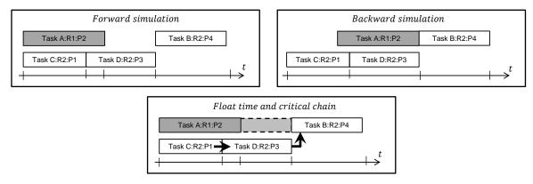
Figure 5-9: Applying the new priorities based on the priority-by-end-date method for the backward simulation. The new priorities are set according to the finish date of the task in the forward simulation. The result is an identical execution sequence of the tasks with the backward simulation, therefore total float and the critical chains are determinable. (Float: dasher gray box, critical chain: large arrows)
