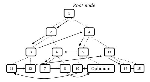
Figure 6-13: Schematic representation of the working mechanism of the best first search without fathoming any nodes (numbers: order of determination)
