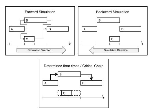
Figure 5-5: Concept of determining total float and critical chain by combining forward (left) and backward simulation (right). (Critical chain: large arrows; float: dashed box)
