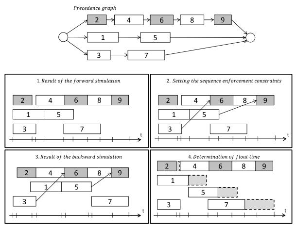
Figure 5-15: Determination of the sequence enforcement constraints for the backward simulation after the forward simulation. (Different colors: different resource needs, arrows: new constraints, dashed boxes: float time)
