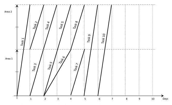
Figure 2-5: Linear schedule representation of the introduced construction project in Figure 2-1. Task 2 and task 8 have been accelerated (duration 1 day) in order to get more parallel execution lines and a more compact schedule.
