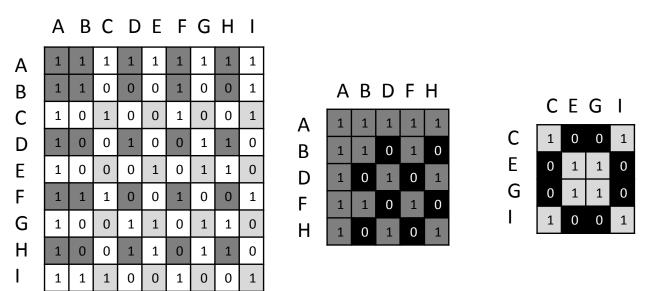
Figure 7-4: The dependency matrix and the fragmented dependency matrices for the different resource classes (dark and light gray). Black elements with white text: independent pair of tasks
