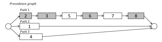
Figure 5-16: An example with large path length differences (|Path 1| >> |Path 2| + |Path 3|)
