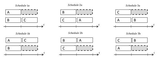
Figure 5-4: Solution combinations for the introduced example (dashed gray box: total float time)
