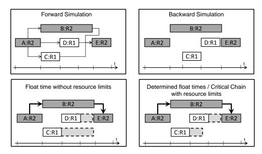
Figure 5-6: Determination of float time taking resource limitations into account (tasks: A, B, C, D, E; resources: R1 (white), R2 (dark gray); precedence relationships:  $A \rightarrow B$ ,  $A \rightarrow C$ ,  $A \rightarrow D$ ,  $B \rightarrow E$ ,  $C \rightarrow E$ ,  $D \rightarrow E$  (thin arrows); float time: dashed light gray boxes; critical chain: large arrows)
