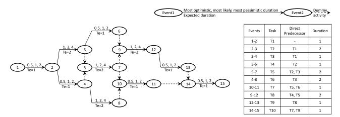
Figure 2-12: AOA-based PERT representation of the introduced construction project in Figure 2-1. On the arrows PERT uses three task duration estimates: the most optimistic, the most likely and the most pessimistic one. Below each arrow is the expected duration of the task.
