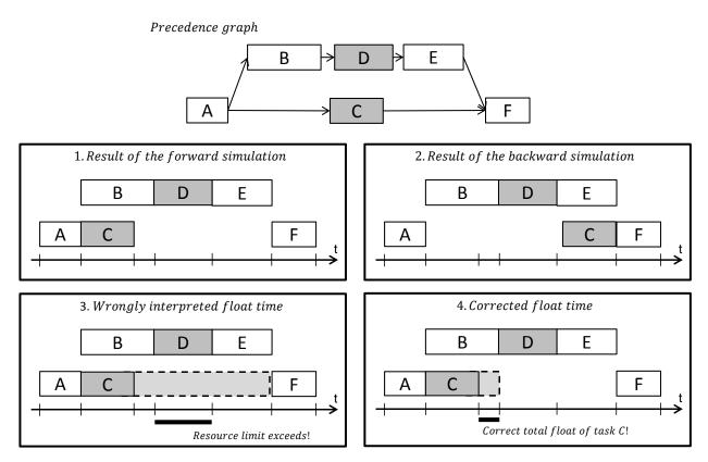
(1) Figure 5-14: Results of the forward and backward (2)simulations. the The problem the resource limits time period (3): exceeding at of float time. The solution (4): maintain the relative order of C and D  $\rightarrow$  shorter total float time for C. (different colors: different resource needs))
