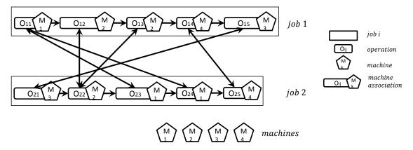
Figure 2-17: Disjunctive graph model of the first two jobs of the introduced job shop problem in Figure 2-16. Simple arrows: conjunctive arcs, double arrows: undirected disjunctive arcs.
