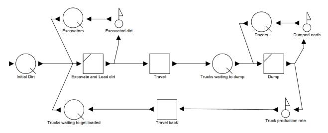
Figure 3-13: Simple cyclic earthwork simulation model with CYCLONE.
