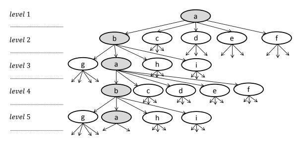
Figure 7-8: The effect of re-swapping: a loop inside the enumeration tree. The child nodes of *node a* and *node b* are determined at every  $2^{nd}$  level. The nodes represent a feasible schedule. The re-swapping is marked with gray node-background. To avoid this behavior a tabu search algorithm is applied that forbids to re-swapping of previously swapped priorities.
