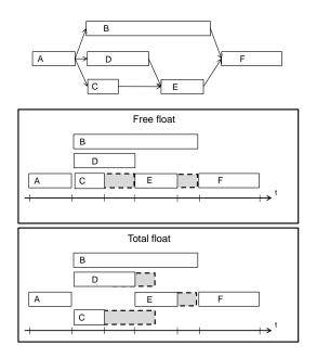
Figure 5-1: Difference between the free and the total float (top: precedence graph of the tasks, middle: free float, bottom: total float, dashed box: float)
