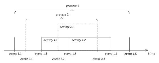
Figure 3-9: Relationship between events (vertical lines), activities (boxes) and processes (curly brackets) represented with an example of two processes. A process might be the complete construction process of a wall. Activities could be assembling the reinforcement and formwork of the wall or pouring concrete. Events might represent the start of assembling the reinforcements, or finishing the pouring concrete activity.
