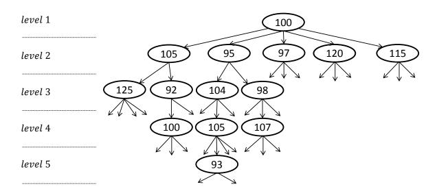
Figure 7-7: Schematic representation of a part of the enumeration tree. Every node symbolizes one schedule. On the top is level 1 representing a randomly generated base schedule. The number in the nodes represents the makespan of the schedule. One arrow accords to one applied reasonable priority swap.
