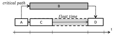
Figure 1-5: Representation of float time and critical path within a schedule. Tasks: boxes; task interrelationships: arrows; critical path: dotted arrows; float time: grey, dashed box
