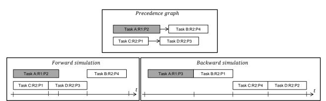
Figure 5-8: Issue with reversed priority settings for the backward simulation: change in the execution order of the tasks (R: resource class, P: priority)
