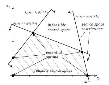
Figure 6-5: Representation of the introduced two-dimensional LP problem
