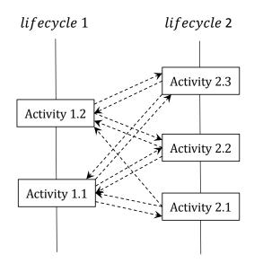
Figure 3-10: Parallel execution of two lifecycles (processes). The arrows represent interaction between the activities of the processes.
