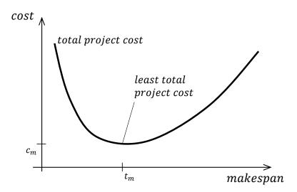
Figure 1-2: Relation between the schedule makespan and the total cost of a project (based on Berthaut et al. 2011 and Baker 1991)
