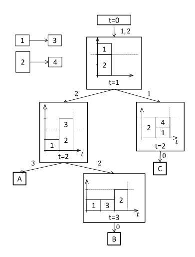
Figure 6-16: The Branch-and-Bound tree of the example determined by delay alternatives
