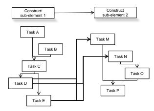
Figure 4-8: The process of mapping high-level precedence-constraints to the task-level: set a new constraint between all the tasks of the predecessor component that have no successor within the component (task D, E) as precedence of all the tasks in the successor component without predecessor within the component (task M,N)
