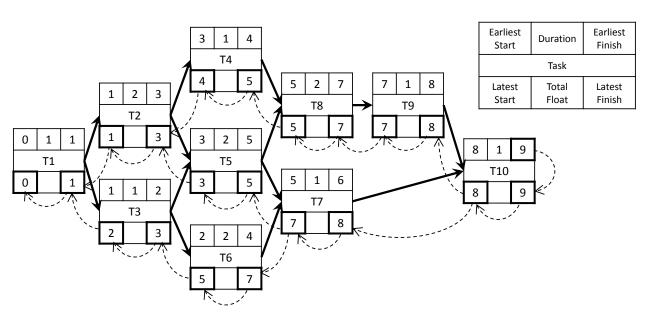
Figure 2-9: Schematic representation of the backward pass for the construction project introduced in Figure 2-1. Determination of the latest start and finish time of the tasks. Boxes: tasks, arrows: precedence relationships, dashed arrows: steps of the calculation.
