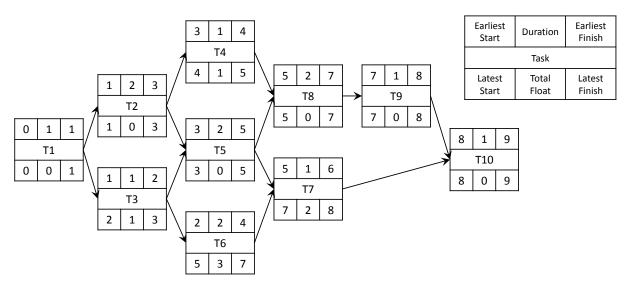
Figure 2-7: Activity-on-Node representation of the introduced construction project in Figure 2-1. Boxes: tasks, Arrows: precedence relationships. Information about the tasks like earliest or latest start time are represented inside the tasks box.
