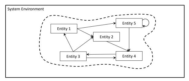
Figure 3-3: Representation of a closed system that has no interaction at all with its environment.
