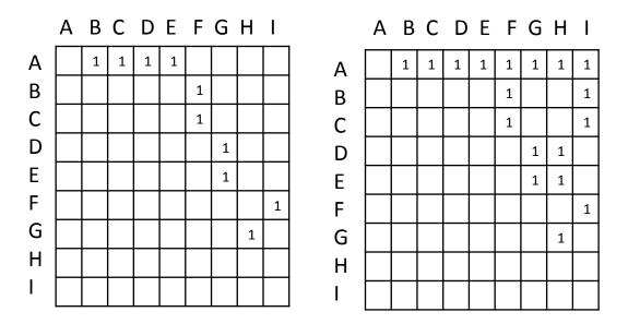
Figure 5-11: Adjacency matrix (left) and the transitive closure (right) of the introduced precedence graph (Figure 5-10)
