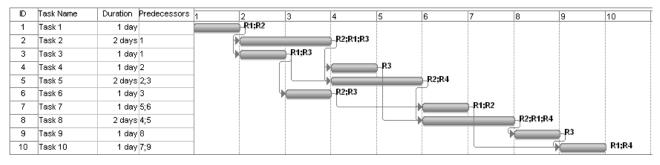
Figure 2-3: Gantt chart representation of the introduced construction project in Figure 2-1. The bars represent the planned execution time interval of a task. Behind the bars the for the tasks execution necessary resources are illustrated. The interrelationships between the tasks are hardly traceable. (MS Project 2007)
