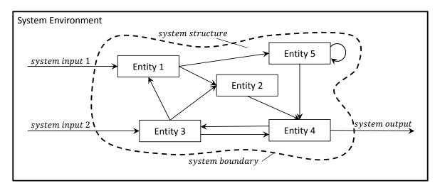
Figure 3-2: Representation of the system environment, the system boundaries and the system with its entities and their interactions. (Based on Page and Kreutzer 2005)
