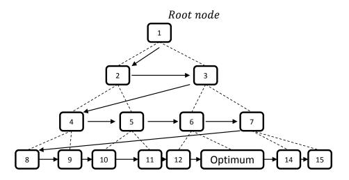
Figure 6-12: Schematic representation of the working mechanism of the breadth first search without fathoming any nodes (numbers: order of determination)
