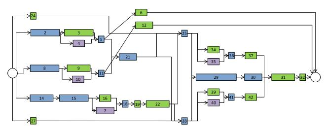
Figure 5-19: Precedence graph of the introduced test case. Colors: resources, such as blue: "concreting", purple: "armouring" and green: "casing".
