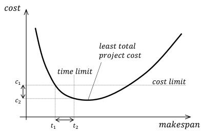
Figure 1-3: Restricting the area of feasible schedules by applying cost and time limits for the completion of the project
