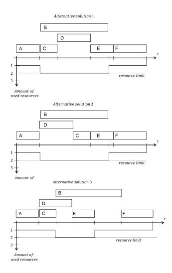
Figure 5-3: Alternative solutions for the in Figure 5-2 introduced resource limit exceeding problem: pushing one of the tasks B, C or D forward in time.
