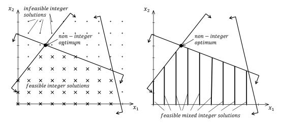
Figure 6-6: IP (left) and MIP (right) representation of the introduced two-dimensional problem (the feasible integer solutions are marked with X.
