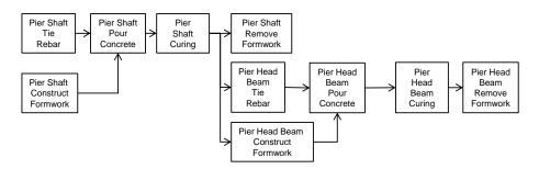
Figure 4-10: Corrected precedence graph of the introduced task sequence in Figure 4-9
