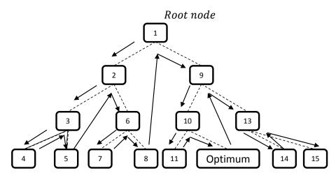
Figure 6-11: Schematic representation of the working mechanism of the depth first search without fathoming any nodes (numbers: order of determination)
