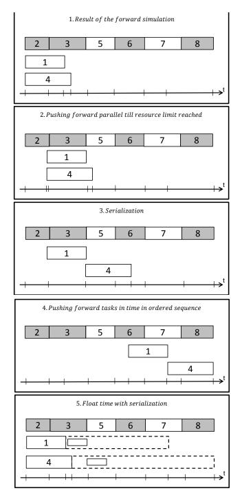
Figure 5-18: The effect of serialization for the determination of float time. (Dashed boxes: float time; boxes in float time: start point and order of serialization)
