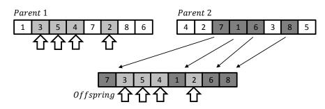
Figure 6-21: Position-based cross over: chromosomes made up of eight components that represent task IDs from a schedulable project. The selected component of the first parent (light grey) will be inserted into the offspring at the same position. The missing element will be filled up from the second parent (dark grey) keeping the sequence of the components.
