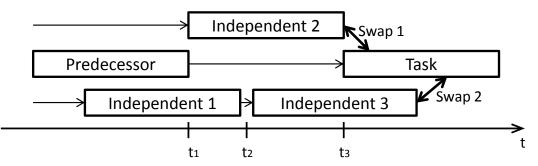
Figure 7-5: Schematic illustration of the reasonable swap determination: the list of possible swaps of independent tasks is restricted by the ones that start between the latest finish date of the task's predecessors (t1) and the task itself (t3). Priorities: Predecessor: 10, Independent 1: 8, Independent 2: 6, Independent 3: 4, Task: 2. Reasonable swaps: Task and Independent 2; Task and Independent 3.
