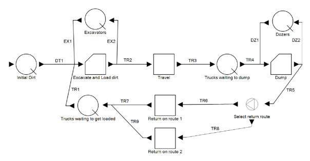
Figure 3-15: STROBOSCOPE ACD for the simple earthmoving system that was introduced in Figure 3-13 extended by a fork element allowing the trucks to select a return route. The meaning of link names: DT stands for dirt, EX for excavator, DZ for dozer and TR for truck.
