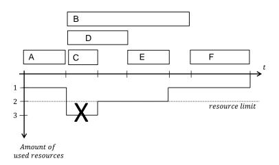
Figure 5-2: Exceeding the resource limits within a schedule determined by CPM. (Precedence graph of the tasks is depicted in Figure 5-1)
