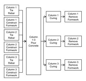
Figure 4-12: Grouped assignment for pouring concrete to three columns
