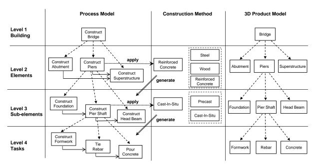
Figure 4-4: Representation of the *levels-of-detail* approach on a simple bridge project. Normal arrows: precedence constraints, dashed arrows: hierarchic decomposition, dotted arrows: construction method selection, double arrows: automatic generation of new components (Wu et al. 2010a).
