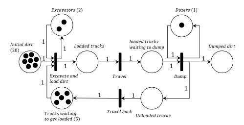
Figure 3-21: Petri Net model of the in Figure 3-13 introduced simple earth moving project at the initial state
