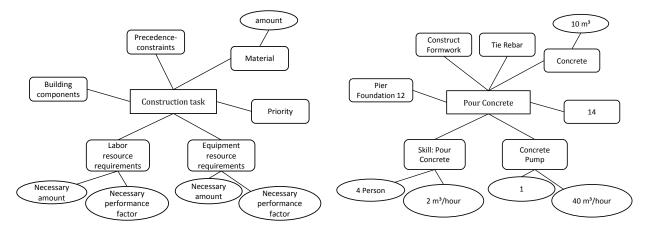
Figure 4-6: Activity package. Left: content, right: example (based on Wu et al. 2010a)
