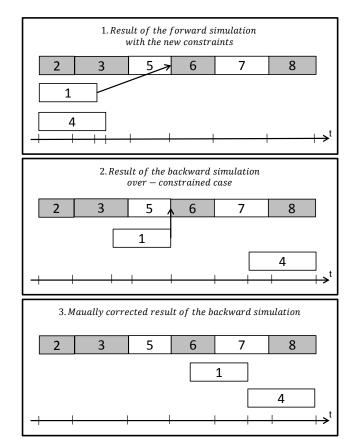
Figure 5-17: The simulation results from the example introduced in Figure 5-16. In the bottom are the manually corrected or expected results.
