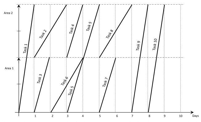
Figure 2-4: Linear schedule representation of the introduced construction project from Figure 2-1. The construction site is divided into two regions: area 1 and area 2. The execution direction of every task is forward from the start point to the end of area two. There are tasks, such as task1, task 5, task 9 and task 10, which are executed continuously in both areas and the other tasks that are executed only in one area (e.g. task 2 in area 2 and task 3 in area 1).
