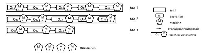
Figure 2-16: Schematic representation of a job shop problem: the jobs are made up of different  $(n_i)$  amounts of operations  $(O_{ij})$  that are connected to each other with precedence relationships as described by the flow shop problem. For the job shop problem the ID of the required machine for a task's execution is not necessarily equal to the task's place in the flow sequence.
