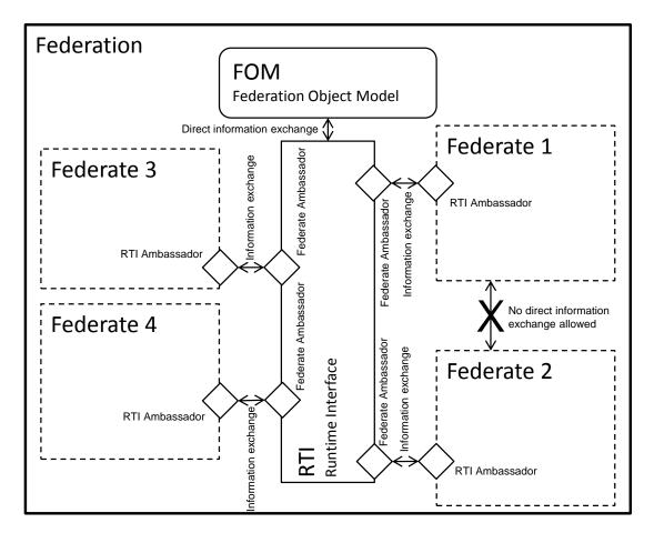
Figure 3-19: Components of the High Level Architecture: The federation, the RTI, the FOM, federates and Ambassadors
