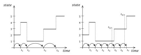
Figure 3-8: Comparison of the event-based (left) and the fix time increments-based (right) simulation clock advancement techniques. Due to the wrong time step size selection the last two events of the simulation must be delayed.  $(t_{3/1} \text{ and } t_{4/1} \text{ represent the time steps } t_3 \text{ and } t_4 \text{ in the first diagram on the left})$
