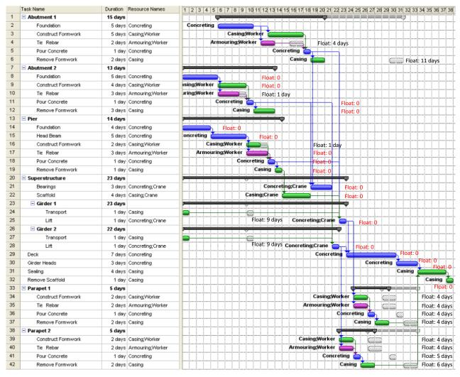
Figure 5-24: The expected results of the introduced example with multiple resource constraints
