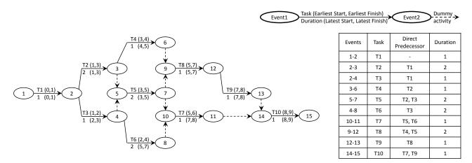
Figure 2-6: Activity-on-Arrow representation of the introduced construction project in Figure 2-1. Ellipses: Events, Arrows: tasks, dashed arrows: dummy activities.
