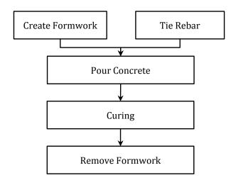
Figure 4-5: Process pattern for cast-in-situ constructed reinforced concrete building component (based on Wu et al. 2010a)
