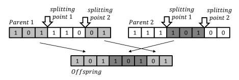
Figure 6-19: Two-point cross over: chromosomes made up of eight binary component. The components of the offspring are originated before the first splitting point and after the second one from the first parent (light grey), between them from the second parent (dark grey).
