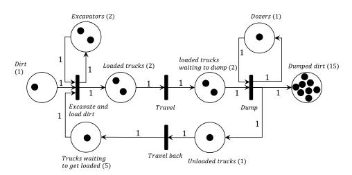
Figure 3-22: Petri Net model of the in Figure 3-13 introduced simple earth moving project in the state after transporting 15 entities of dirt to the dump area.
