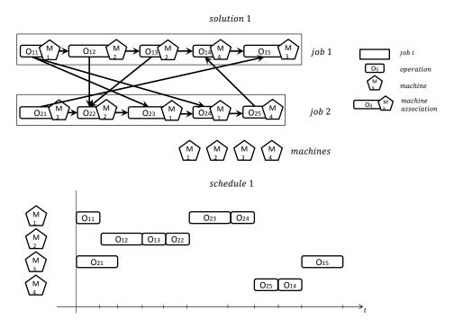
Figure 2-18: One feasible solution for the introduced disjunctive graph from Figure 2-17. Every disjunctive arc has been turned into a fixed arc resulting in an acyclic graph defining exact execution orders of the operations for every single machine.
