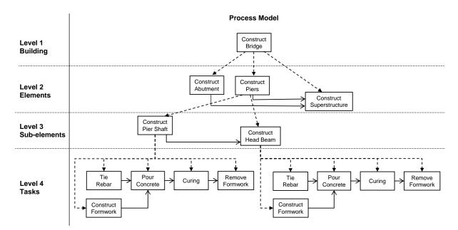
Figure 4-7: Hierarchic precedence graph representation of a simplified bridge construction project's process model. Arrows: precedence constraints, dashed arrow: hierarchic decomposition
