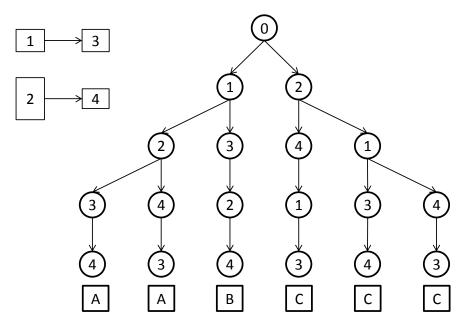
Figure 6-14: Representation of a precedence tree for the task chains  $1 \rightarrow 3$  and  $2 \rightarrow 4$ . The higher the activity the more resources it needs. The letters in the boxes at the bottom represent the resulting schedules from Figure 6-15.
