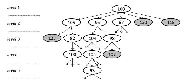
Figure 7-9: Schematic representation of the greedy-like heuristic algorithm. Grey: Fathomed nodes, dashed ellipse: current best solution, arrows: applied swaps. Tolerance factor: 15%.
