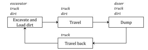
Figure 3-17: ABC representation of the simple earth moving system that has been introduced in Figure 3-13
