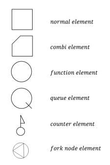
Figure 3-14: Nodal modeling elements of STROBOSCOPE
