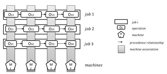
Figure 2-15: Example for a schematic representation of a flow shop problem: the *m* operations  $(O_{ij})$  of every job are connected as a flow with precedence relationships to each other. Every task is executed on the machine corresponding to the position of the operations in the flow sequence. The task is to find the optimal execution order for the jobs.
