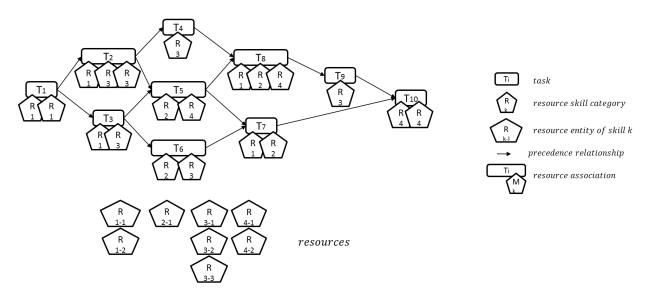
Figure 2-1: Schematic representation of a project scheduling problem under resource constraints. The tasks  $(T_i)$  are represented in a precedence graph with their necessary resources  $(R_k)$ . The longer the box, the longer the duration of the task.
