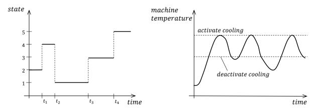
Figure 3-4: Representation of a discrete (left) and a continuous system (right)
