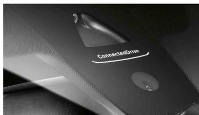
**Fig. 5.6** – Camera integrated in the front mirror mount of a BMW vehicle [12]
