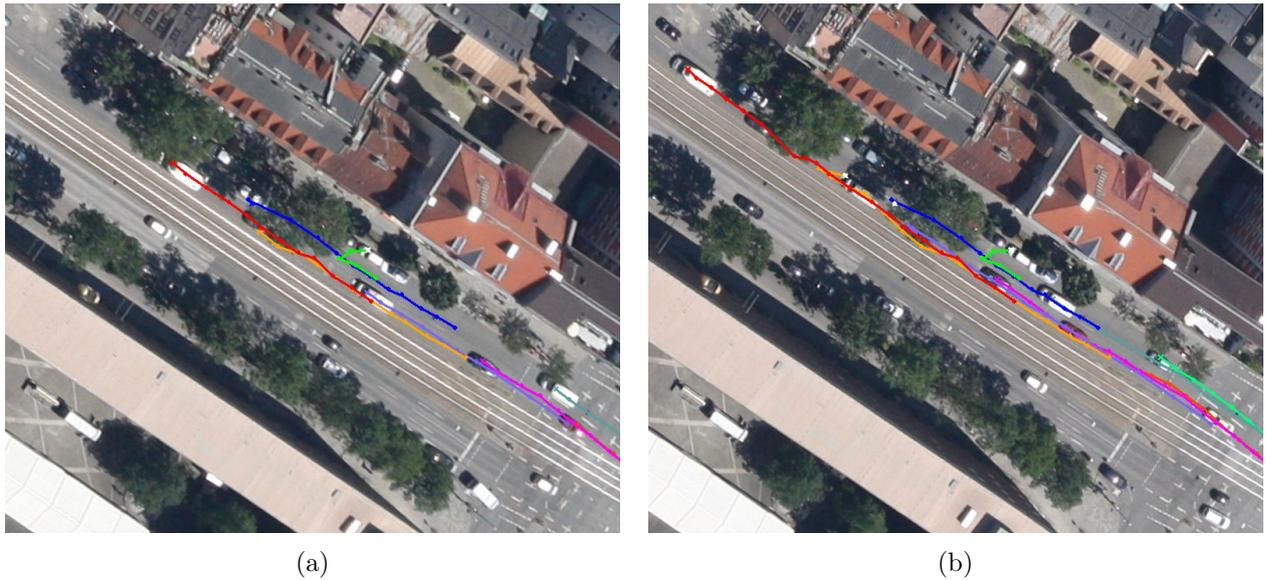
**Fig. 4.30** – Trajectories of tracked vehicles, (a) frame 11, (b) frame 19. Occlusions from trees and their shadows confuse the tracker, which leads to target losses. After the first occlusion in frame 11, the first vehicle (red) and the following two (blue, orange) are tracked successfully. After the second occlusion in frame 19, only the first vehicle is captured while the other two are lost under the trees and in the shadows.
