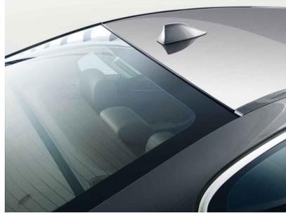
**Fig. 2.7** – GPS antenna integrated in fin mounted on vehicle roof [14]
