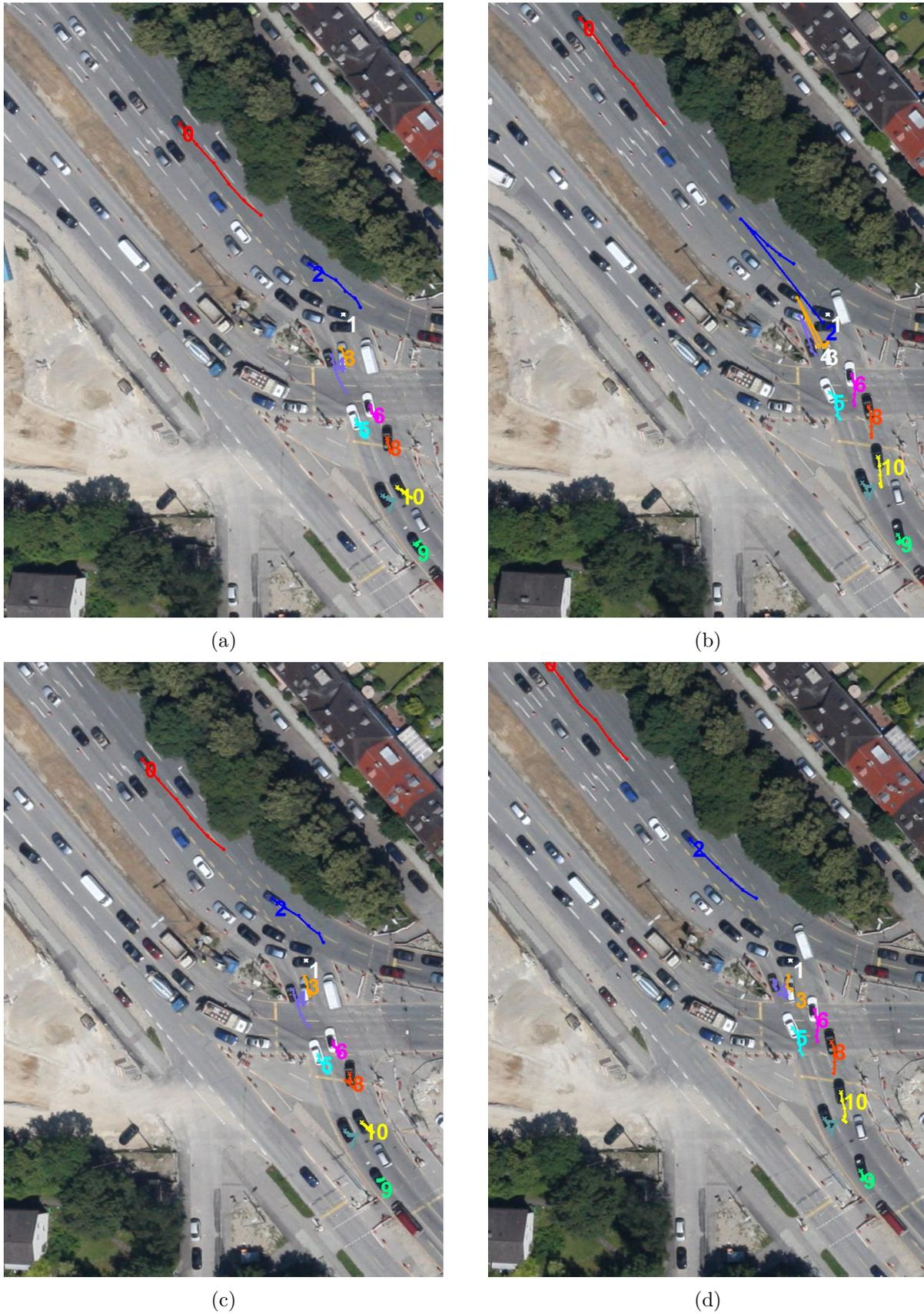
**Fig. 4.15** – Tracking results for small vehicle group from the  $3K+C$  scene. Frames 17 and 22 are shown for (a), (b) non-adaptive sampling and (c), (d) adaptive sampling strategy. Vehicle 2 is lost with the non-adaptive sampling, but tracked successfully with the adaptive sampling strategy.
