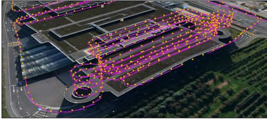
**Fig. 2.8** – Positioning quality of u-blox 3D Automotive Dead Reckoning solution [135]. Vehicle trajectories on this test drive inside a park garage are computed by dead reckoning only. The positioning error at the exit of the park garage (upper-right) is smaller than one lane width.
