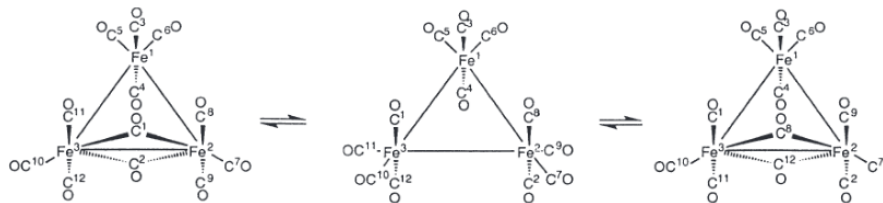
Scheme 4 Fluxionality of triiron dodecacarbonyl
