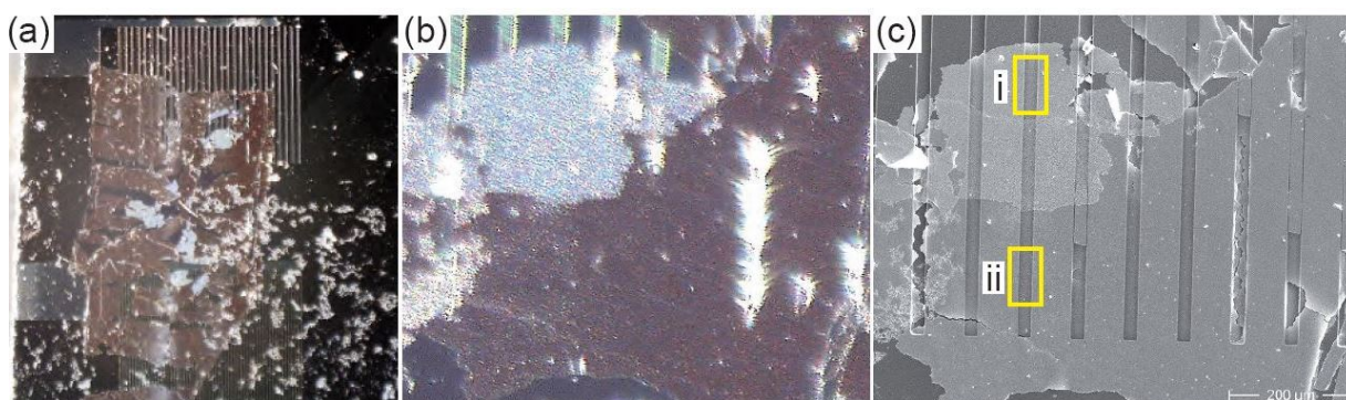
Figure 8.7. Transfer of a laser-sintered film: (a) Following the procedure described in the text, flakes of a laser-sintered NP film are transferred onto a Ge wafer with two trench structures in the upper and lower part of the wafer. In this optical micrograph face-down flakes appear brownish due to unsintered NPs at the backside of the film, whereas face-up flakes appear metallic. (b) Magnification of a flake in panel (a) which is suitable for investigation by the Raman shift method. (c) SEM micrograph of the same region as in panel (b), which shows that the flakes partly overlap. Regions i and ii are suited for Raman mapping.
