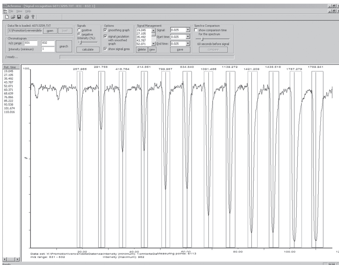
Figure 11.4 Results of the signal recognition with Achroma software tool. Signal areas of the product ((GlcNAc) 4 ) at different inhibitor concentrations (see Table 11.1) are shown.
