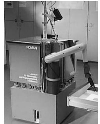
Fig. 3: The speech-understanding service robot ROMAN
