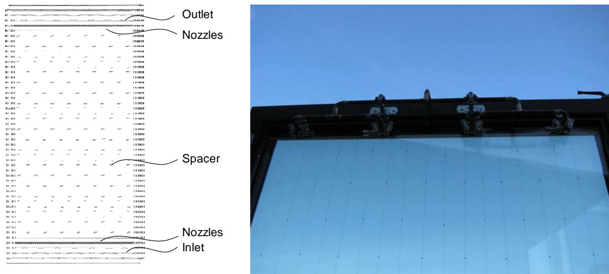
Figure 3 Left: Prototype façade element with 4 inlets at the bottom and 4 outlets at the top (1 m x 1.6 m). Right: Photograph of the upper part showing the positioning of the spacers by thin wires.
