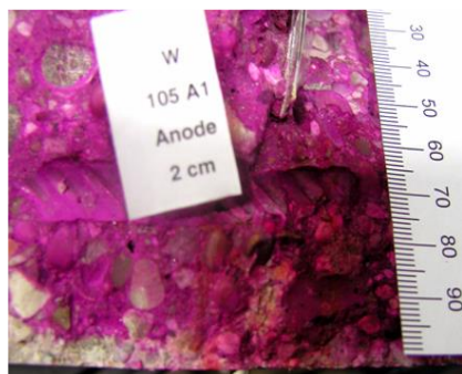
Figure 3-34: Carbonation tests, I05360, 1 year exposure
