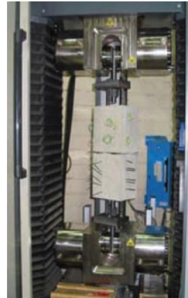
Figure 3-7: Creating cracks with tension tests
