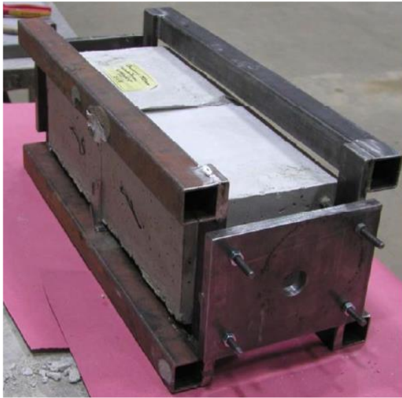
Figure 3-1: Cracked beam in the frame
