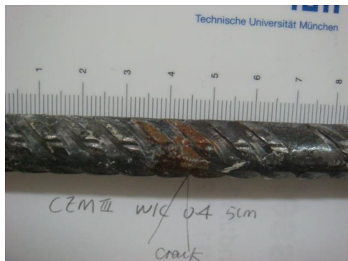
Figure 3-44: Corrosion area of III04360, Cl cycle, cover=5 cm, 3 years exposure
