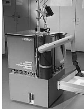
Fig. 19: Speech-understanding service robot ROMAN
