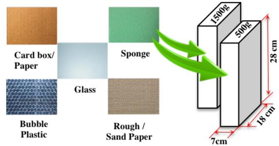
Fig. 2. Objects having the same size and two different weights ( $w \in W$ ) are covered with five most common surface textures, Rough Texture or Sand Paper, Glass, Sponge, Paper or Card box, and Bubble Plastic ( $t \in T$ ).
