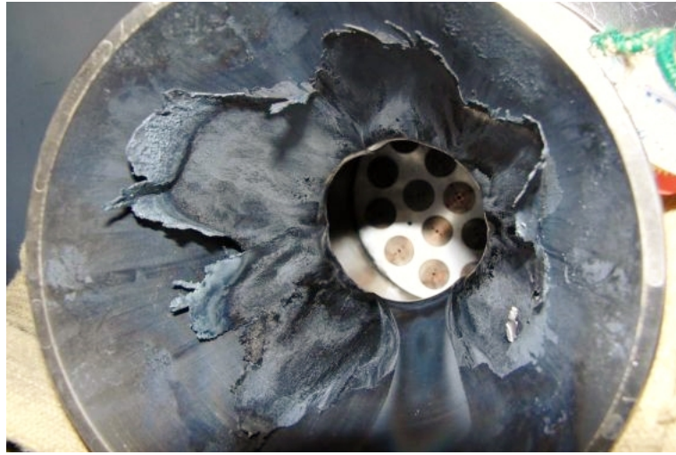
Figure 1.2: Image of a melted nozzle highlighting the possible impact of thermoacoustic oscillations. Image taken from [158].
