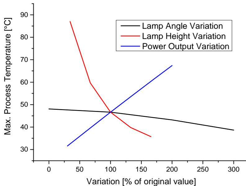
Figure 4.37. Process parameters variations for lamp angle, lamp normal height to the substrate and the lamp power output
