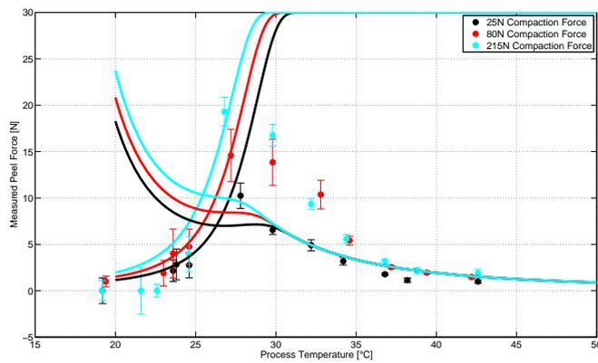
Figure 6.9. Peel Forces over Temperature for varying compaction pressures, experimental values from Crossley et al. [27]
