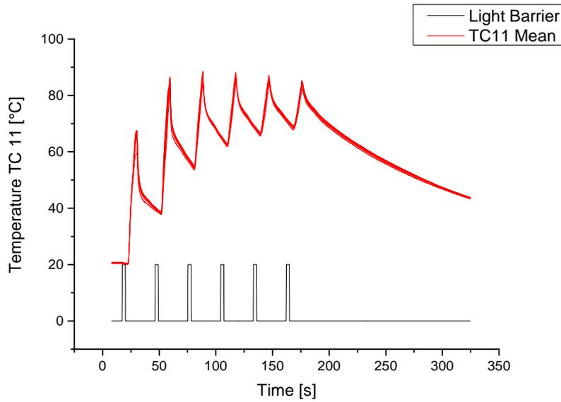
Figure 4.26. Experimental temperature of TC 11 during placement of all plies
