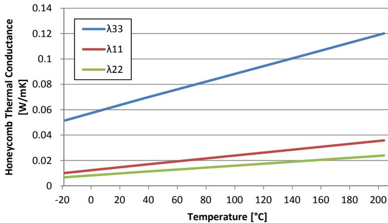
Figure 4.2. Orthotropic thermal conduction of *Hexcel Nomex honeycomb HRH-10-1/8-3.0*
