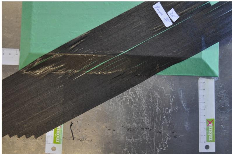
Figure 3.9. Emerging gaps at ramp angle 30° and a path angle of 30°
