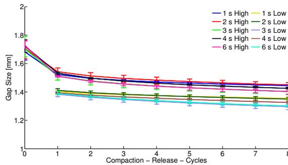
Figure 3.39. Compaction results of MD setup with compaction time Variation
