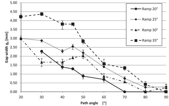
Figure 3.11. Experimental gap width  $g_3$  at the bottom of the ramp [42]
