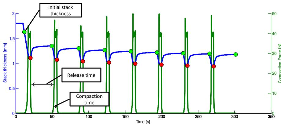
Figure 3.36. Experimental result for 55 °C Compression, with superimposed result evaluation procedure
