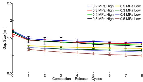
Figure 3.42. Compaction results of UD setup with pressure variation
