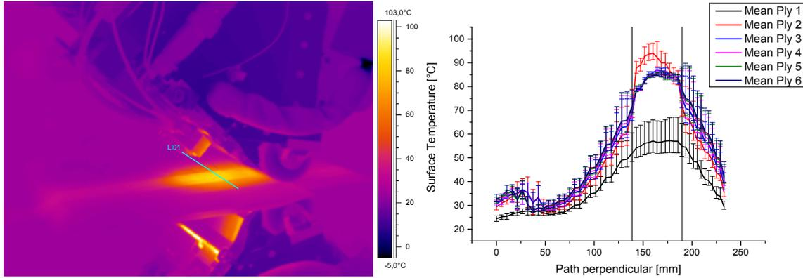
Figure 4.31. Surface temperature perpendicular to path direction (right) for all six plies (left)
