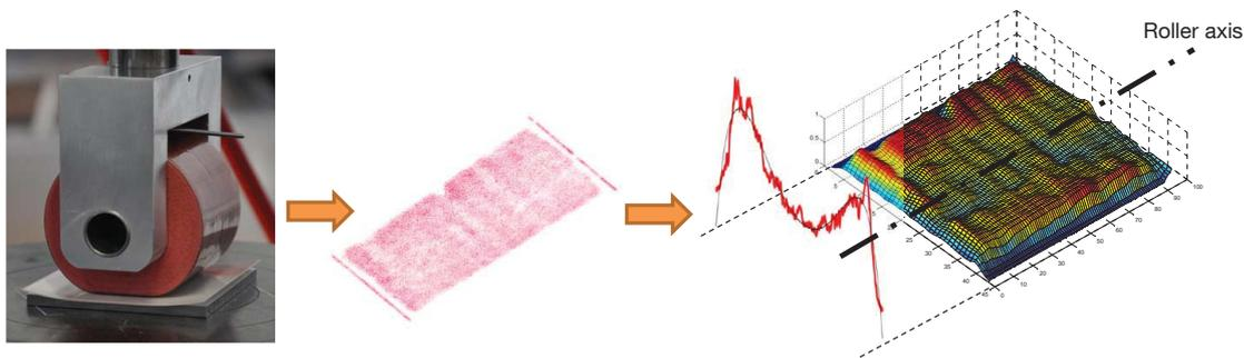
Figure 3.18. Pressure evaluation procedure, compare Lichtinger et al.[42]
