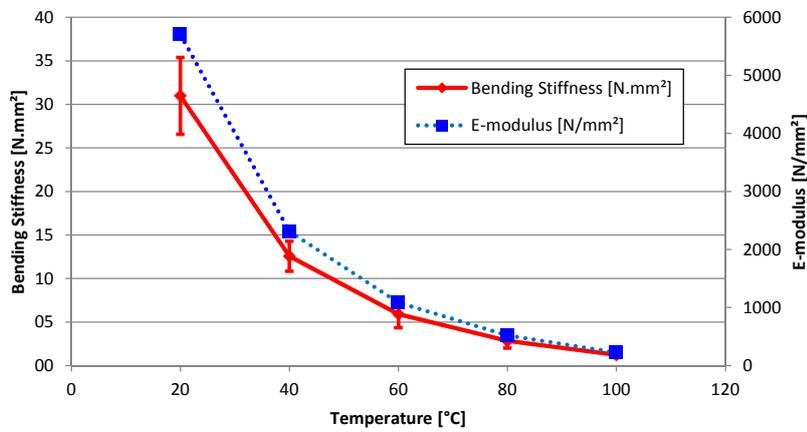
Figure 5.2. Slit-tape bending stiffness as a function of temperature of material 2
