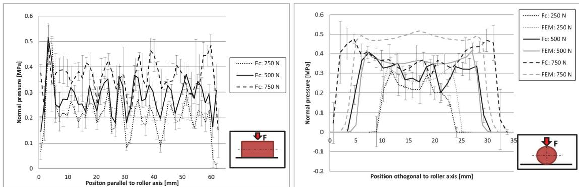
Figure 3.24. Pressure distribution of the compaction roller on the flat tool parallel to roller axis [42].
