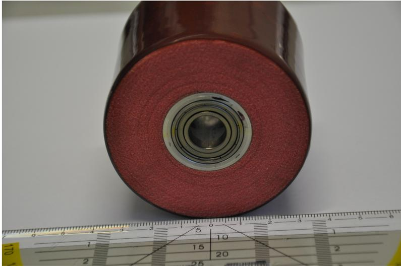
Figure 3.16. *Coriolis Composites* compaction roller for  $8 \times 1/4$  inches slit-tapes [42].
