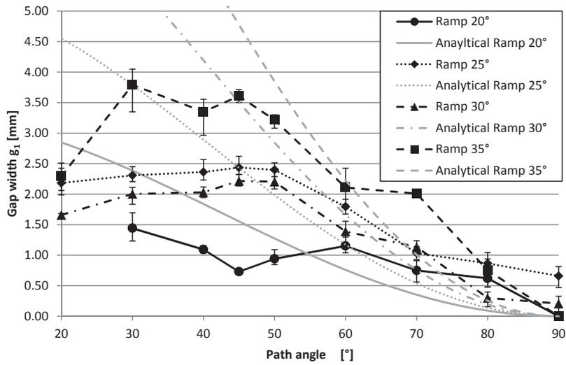
Figure 3.8. Gap width analytical results compared to experimental values
