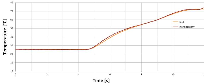
Figure 4.3. Thermography Emissivity calculation with help of the thermal video analysis, the light barrier as well as the TC recording
