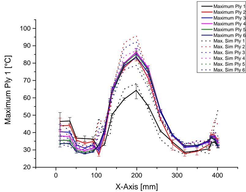
Figure 5.7. Maximum temperatures after the placement of each ply at every TC
