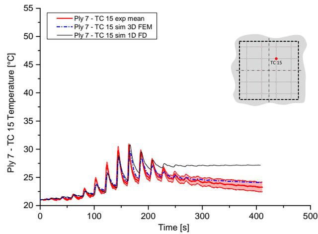
Figure 4.15. Bulk temperature of TC 15 during placement of ply 7, compare Lichtinger et al. [28]
