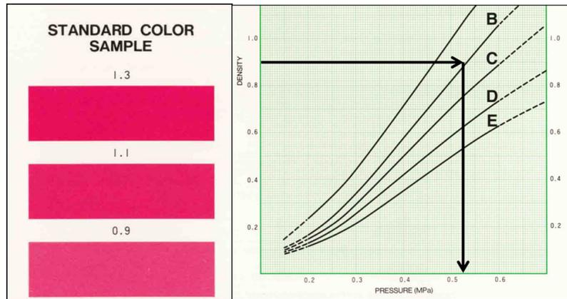
Figure 3.20. Evaluation procedure of the *FUJIFILM Prescale* pressure sensitive film [70]
