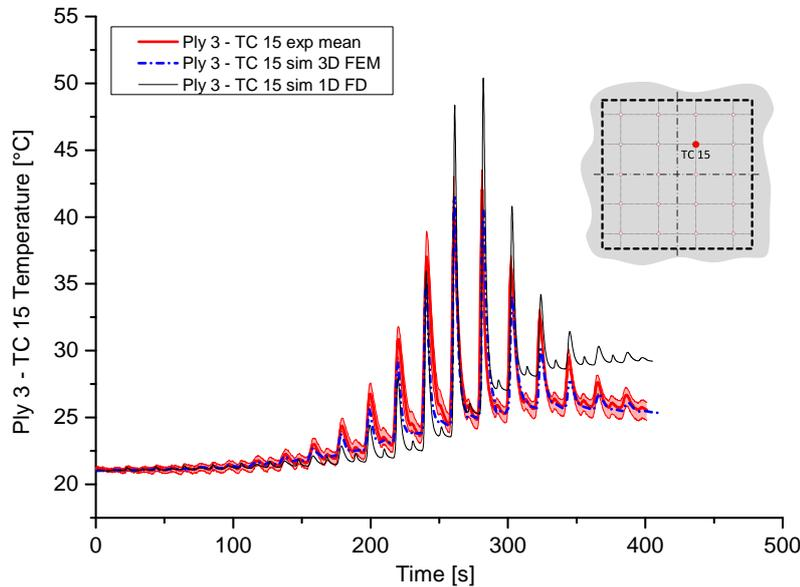
Figure 4.14. Bulk temperature of TC 15 during placement of ply 3, compare Lichtinger et al. [28]
