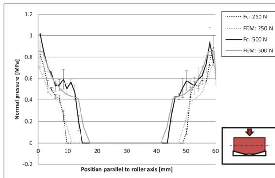
Figure 3.29. Normal pressure of the compaction roller in lateral direction parallel to roller axis on the concave tool, compare Lichtinger et al. [42]
