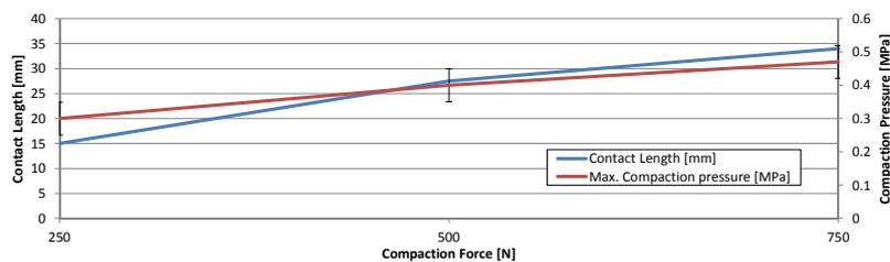
Figure 3.26. Contact length and maximum pressure over the compaction force
