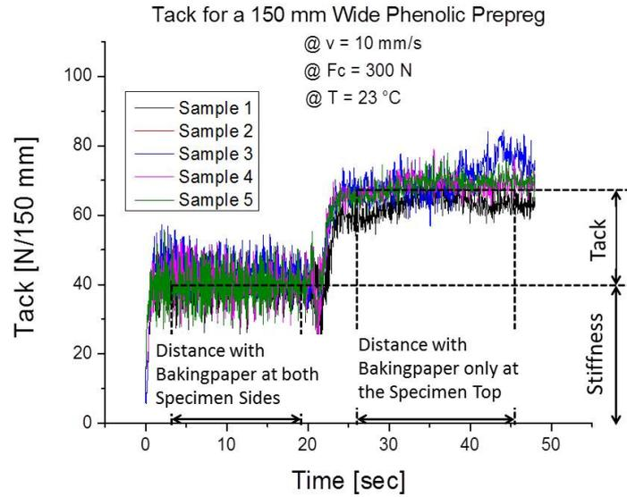
Figure 6.5. Exemplary data from measurement of the peel tack setup [122]
