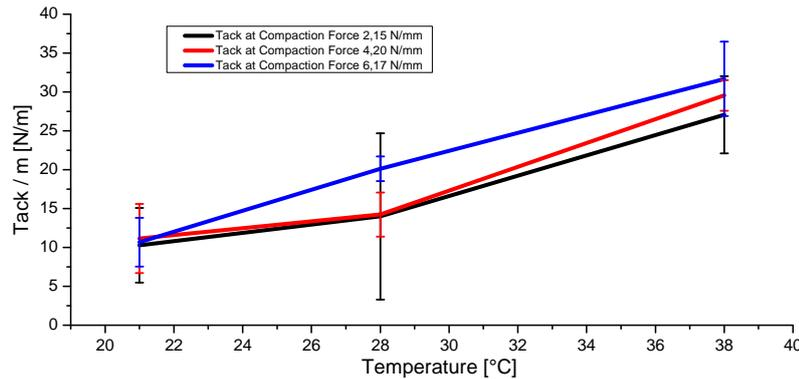
Figure A.2. Measured Tack over temperature, with standard variance after three measurements
