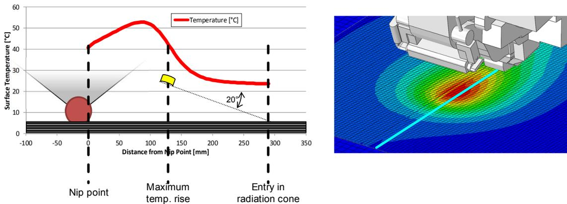
Figure 4.23. Temperature along the path direction from simulation (left) and evaluation path (right)
