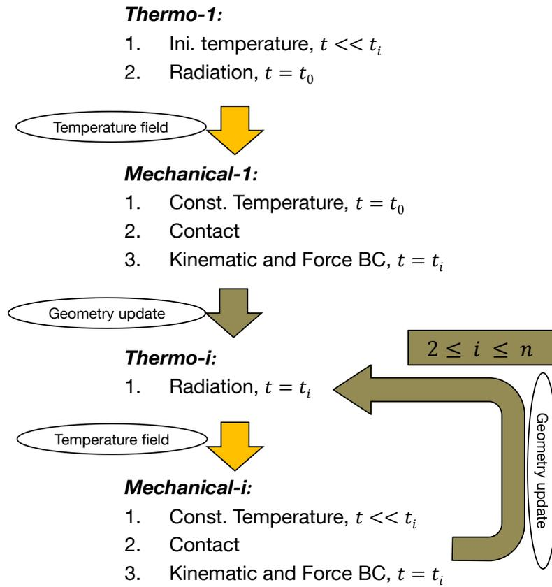
Figure 5.4. Sequential coupling procedure of the thermo-mechanical coupled model
