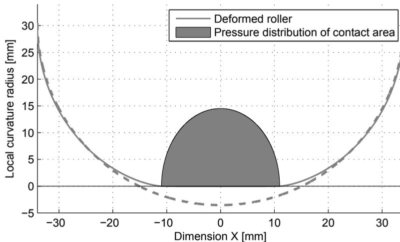
Figure 3.17. Indentation of a roller cross section according to Hertzian theory, along with the pressure distribution
