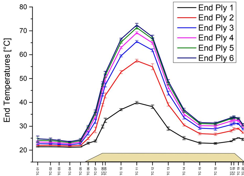
Figure 4.28. Temperature values of all TCs at the end of each ply
