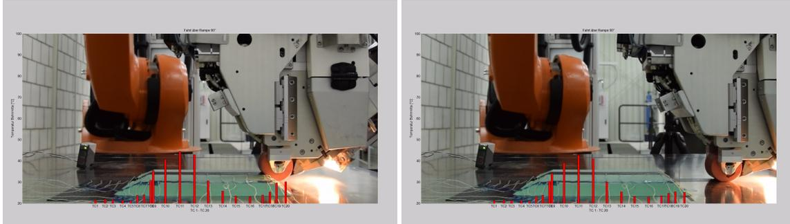
Figure 4.25. Series of images showing the temperature distribution along the placement path on the honeycomb during the placement of the first path
