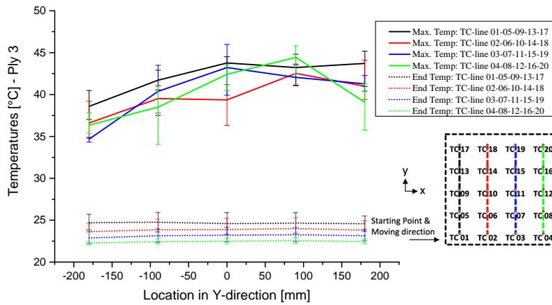
Figure 4.17. Max. and end temperature of ply 3 distributed over the placement area, compare Lichtinger et al. [28]
