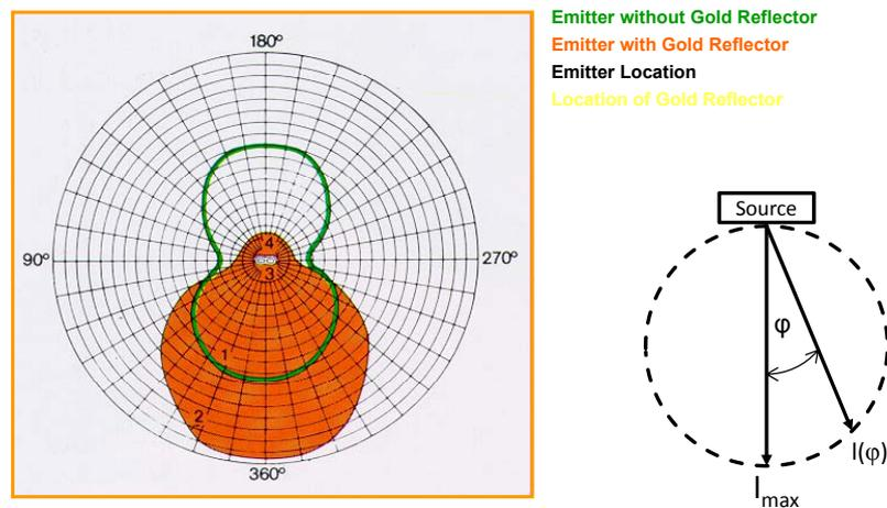
Figure 4.1. Lambert cosine law compared with the radiation distribution of Heraeus Noblelight IR emitter [76]
