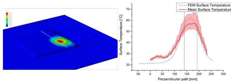
Figure 4.36. Surface temperature during placement of ply 1, 8 s after movement start
