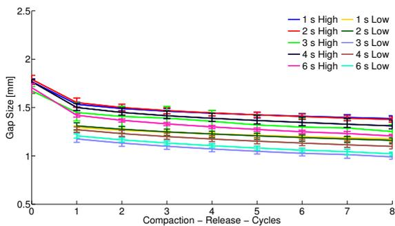
Figure 3.43. Compaction results of UD setup with compaction time Variation
