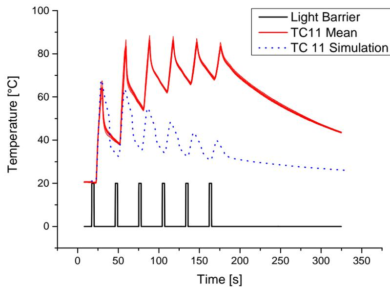
Figure 4.33. Experimental values compared to simulation results at TC 11
