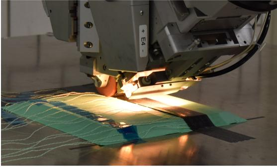
Figure 4.6. *Coriolis Composites* AFP machine for 8 1/4" slit-tapes, located at *Fraunhofer Institute for functional Lightweight Design* in Augsburg, Germany
