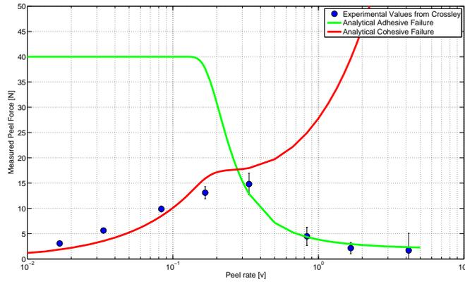
Figure 6.8. Results of the parameter fit for peel tack depending on peel rate; Experimental values from Crossley et al. [44]
