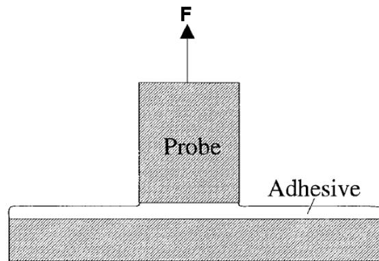
Figure 6.3. Probe Tack Test Setup, compare Lin et al. [117]
