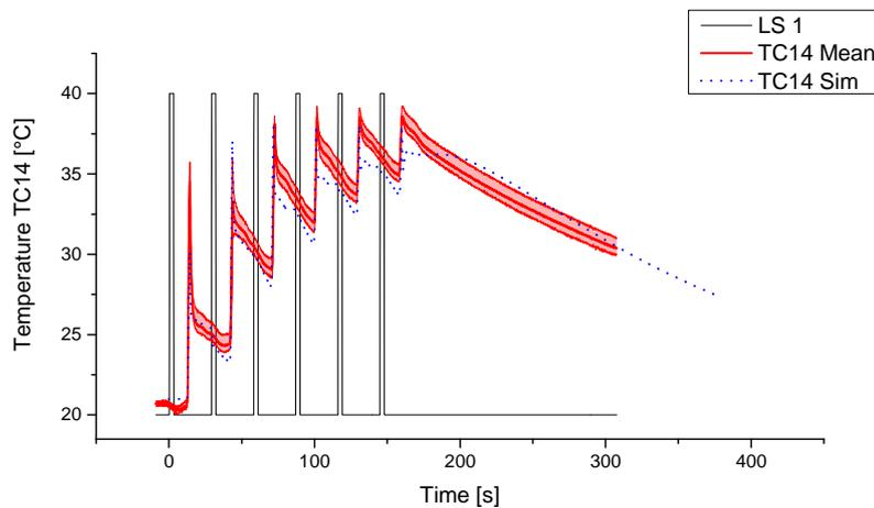
Figure 5.6. Temperature at TC 14: Comparison between Experiments and thermo-mechanically couples simulation results
