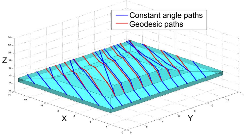
Figure 3.1. Tapered honeycomb on a flat surface with constant angle paths and geodesic paths
