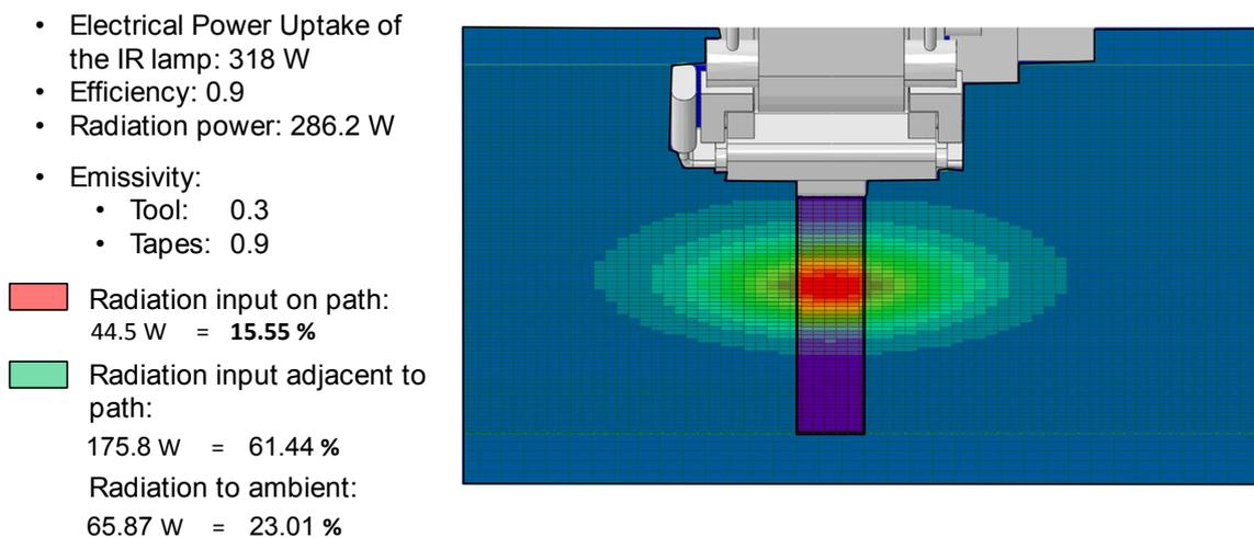
Figure 4.24. Radiation distribution as simulation result
