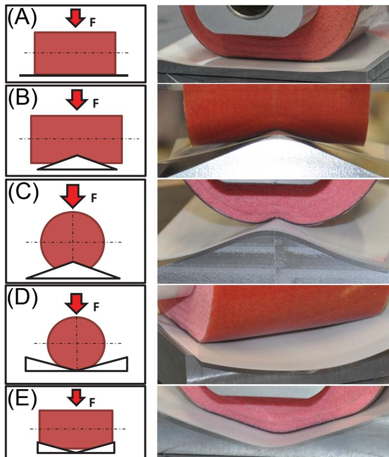
Figure 3.22. Typical roller deformation for all five test setups. (A) Flat tool, (B) convex tool lateral, (C) convex tool longitudinal, (D) concave tool lateral, (E) concave tool longitudinal, compare Lichtinger et al. [42]
