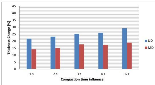
Figure 3.47. Influence of compaction time in thickness change [%] after eight compaction cycles
