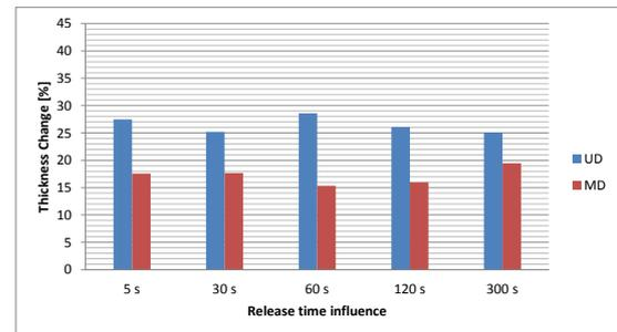
Figure 3.48. Influence of release time in thickness change [%] after eight compaction cycles
