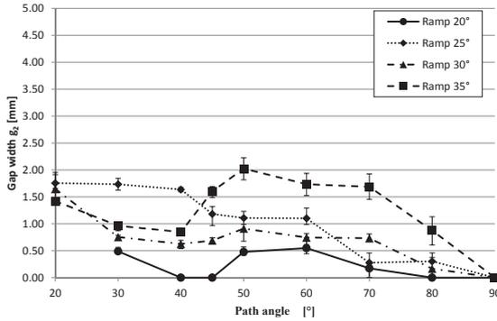
Figure 3.10. Experimental gap width  $g_2$  at the top of the ramp [42]
