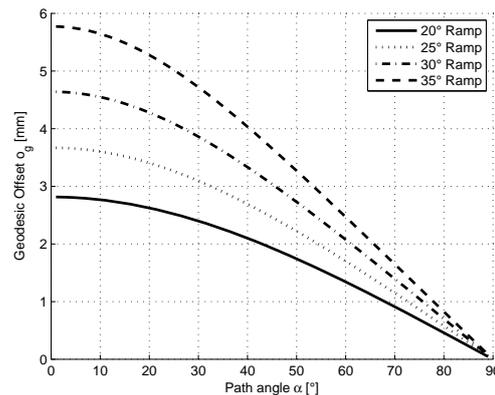
Figure 3.7. Parallel offset due to geodesic path generation [42]
