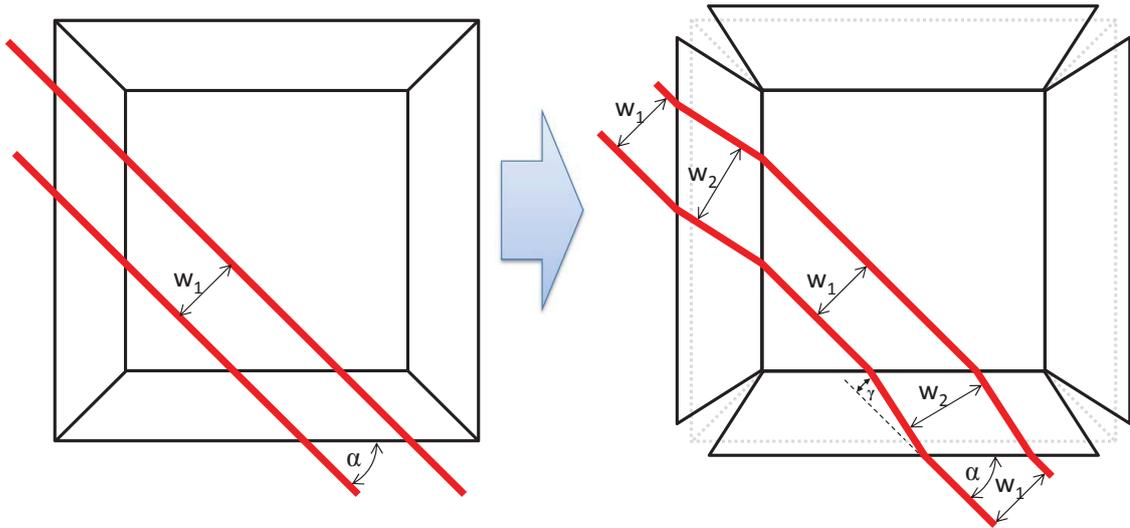
Figure 3.2. Projected path for constant angle paths on a ramped structure (left) with the flat projection (right), compare Lichtinger et al. [42].
