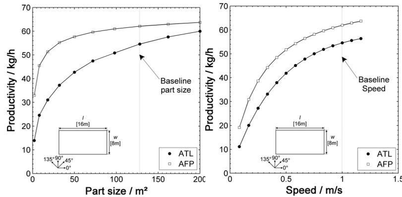
Figure 2.5. Material Throughput of AFP compared to ATL in part size (left) and layup rate (right) [6]
