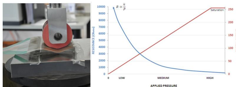
Figure 3.33. Test setup with the *Tekscan* system (l) and its pressure evaluation procedure (r)
