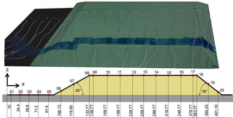
Figure 4.13. Fixtures of the TCs on the adhesive film of the honeycomb structure including their location
