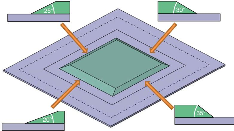
Figure 3.4. Layout of the tool for the testing of gaps, compare Lichtinger et al. [42]
