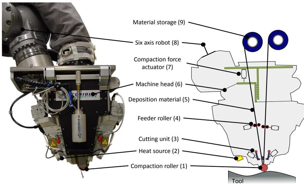
Figure 2.2. *Coriolis Composites* AFP machine (left) with design principle (right)
