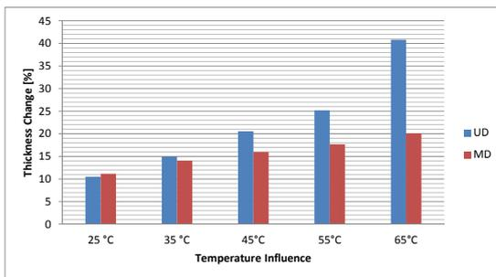
Figure 3.45. Influence of temperature in thickness change [%] after eight compaction cycles
