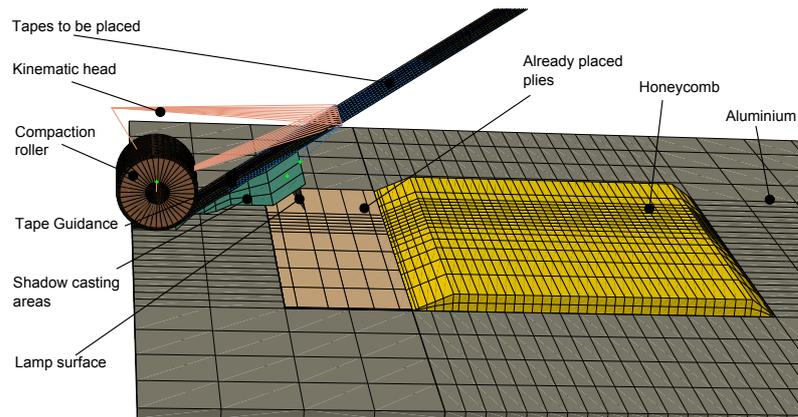
Figure 5.3. Overview of the mechanical model. Image not to scale.
