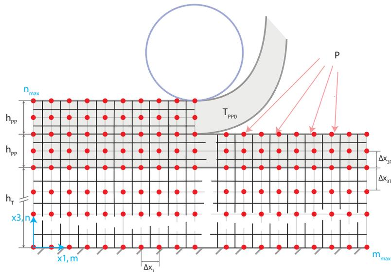
Figure 4.4. 2D FD simulation model discretised with a rectangular mesh
