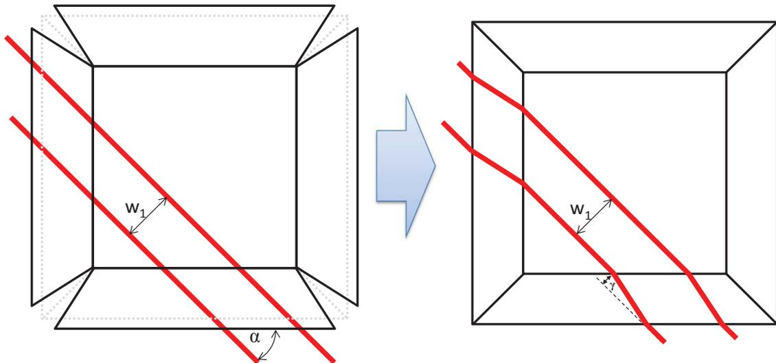
Figure 3.3. Projected path for geodesic paths on a ramped structure (right) with the flat projection (left), as depicted in Lichtinger et al. [42].
