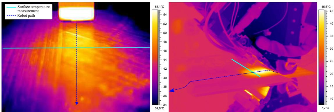
Figure 4.9. Resulting thermography images of flat placement tests (left) and placement on tapered honeycomb (right)
