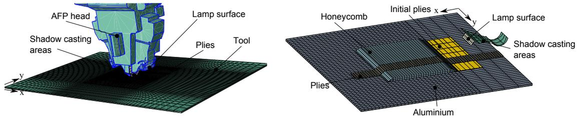
Figure 4.5. Abaqus 3D FEM Models for flat placement experiments on the *Coriolis Composites*  $8 \times 1/8''$  slit-tapes by *LCC* (right) and for the placement on the honeycomb surface *Coriolis Composites*  $8 \times 1/4''$  slit-tapes (left) by *Fraunhofer ICT FIL*. Images not to scale.
