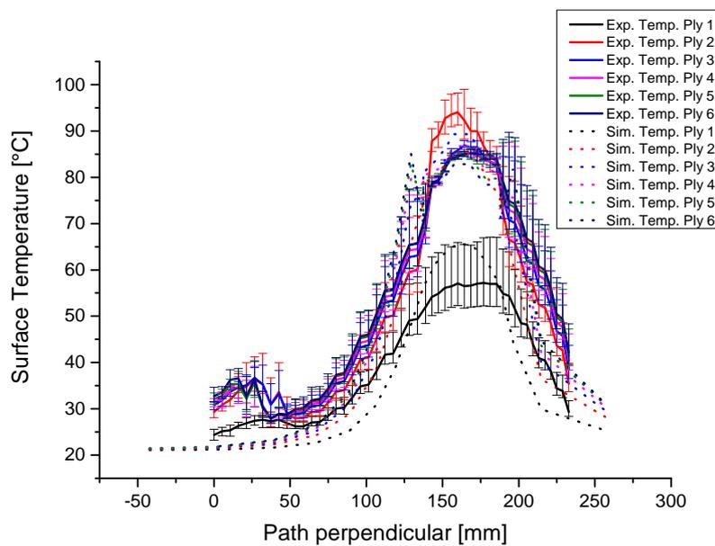
Figure 5.9. Surface temperatures perpendicular to placement direction, 8 s after movement start
