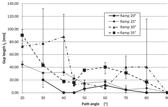
Figure 3.12. Experimental gap length  $l_2$  at the top plane [42]
