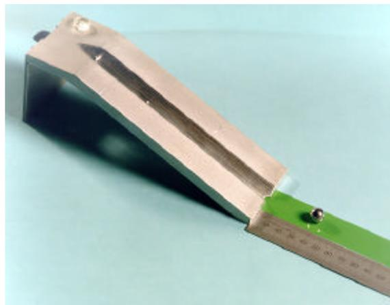
Figure 6.2. Rolling Ball Tack Test, from Duncan et al. [116]
