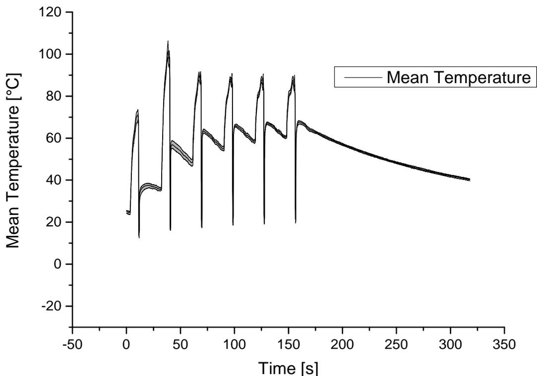
Figure 4.30. Surface temperature spot at location between TC 10 and 11 during the placement of all plies
