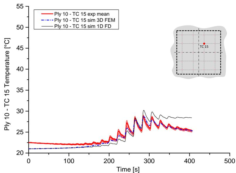
Figure 4.16. Bulk temperature of TC 15 during placement of ply 10, compare Lichtinger et al. [28]
