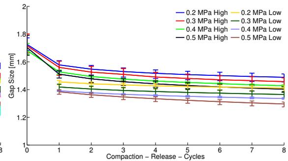
Figure 3.38. Compaction results of MD setup with pressure variation
