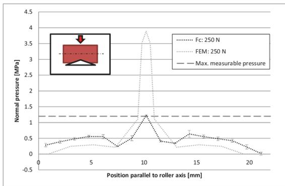
Figure 3.27. Normal pressure of the compaction roller on the convex tool in lateral direction parallel to roller axis, compare Lichtinger et al. [42]
