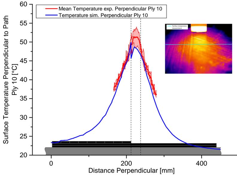
Figure 4.22. Results of Thermography and simulation of surface temperature during the placement of ply 10 [28]
