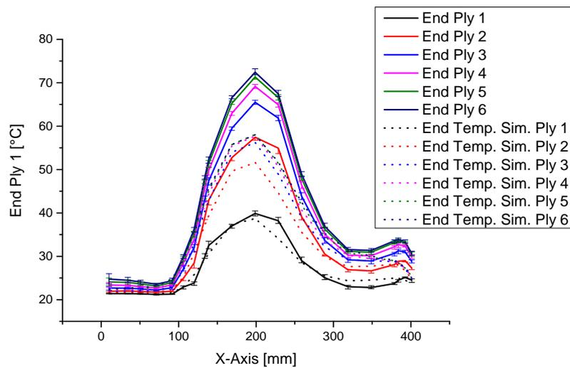
Figure 5.8. Final temperatures after the placement of each ply at every TC
