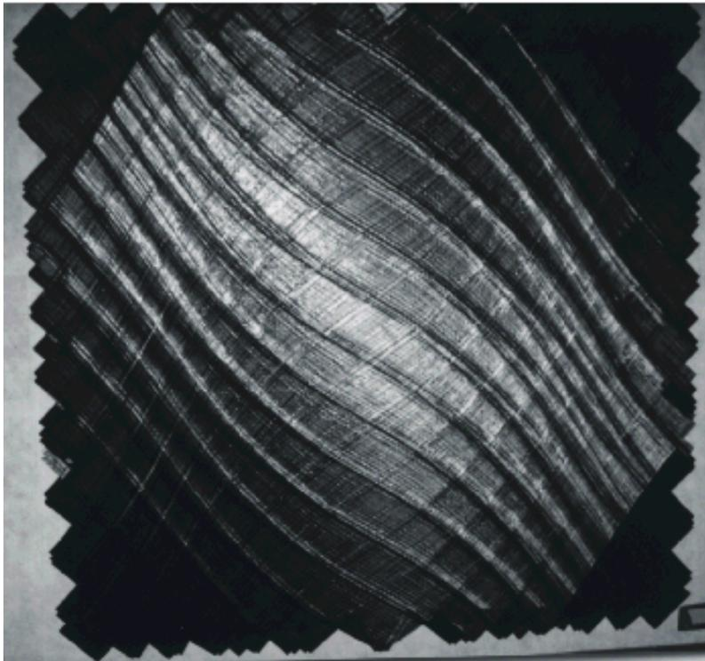
Figure 2.4. A panel manufactured with fibre steering, therefore increasing eigenfrequencies, compare Tatting and Gürdal [16]
