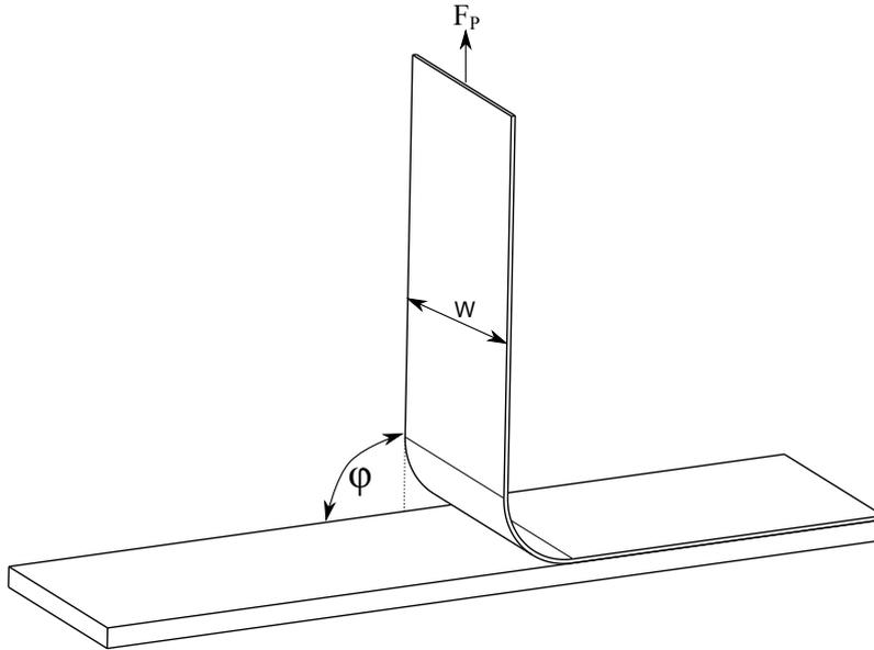
Figure 6.6. Sketch of the peel tack test with process variables
