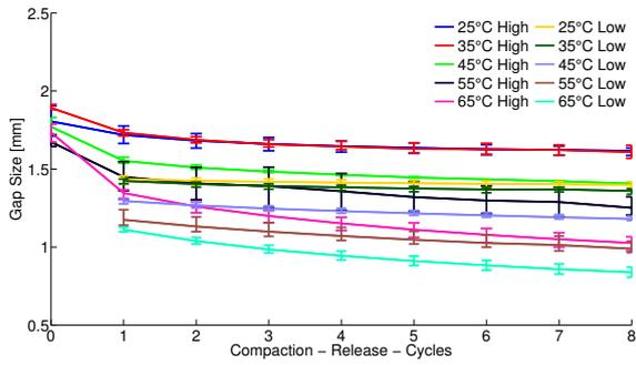
Figure 3.41. Compaction results of UD setup with temperature variation
