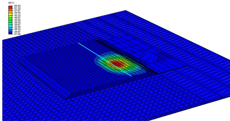
Figure 4.32. Plot of the simulation result in the Abaqus CAE environment 8 s after placement start with perpendicular temperature evaluation path
