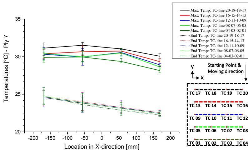
Figure 4.18. Max. and end temperature of ply 7 distributed over the placement area, compare Lichtinger et al. [28]
