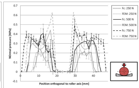
Figure 3.30. Normal pressure of the compaction roller in longitudinal direction orthogonal to roller axis on the concave tool. [42].
