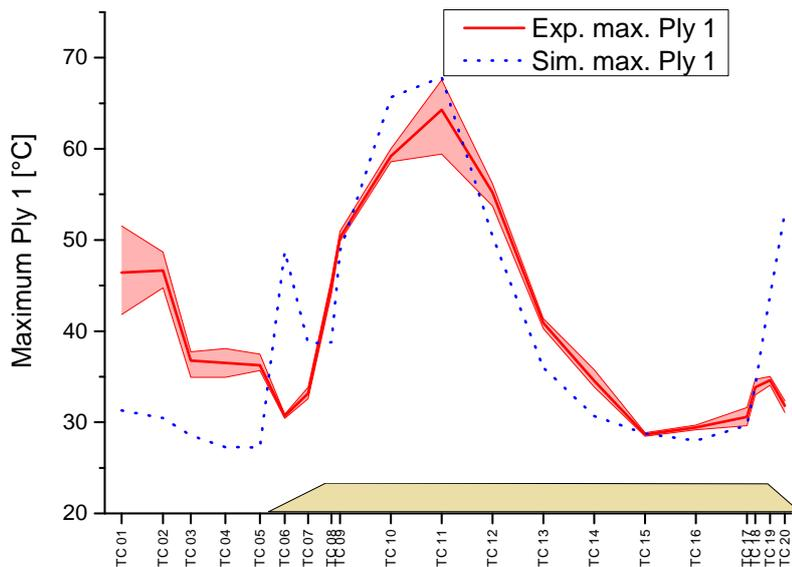
Figure 4.35. Maximum temperature values during the placement of ply 1 for experimental and simulation results
