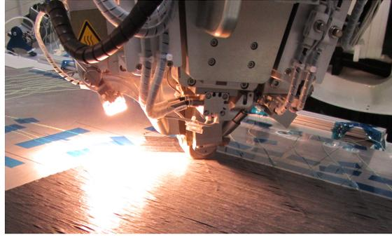
Figure 4.7. *Coriolis Composites* AFP machine for 8 1/8" slit-tapes, located at *Institute for Carbon Composites* in Munich, Germany
