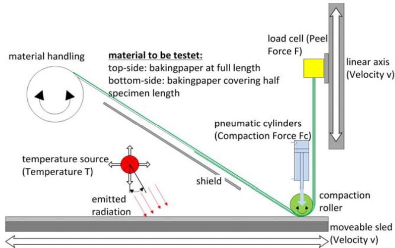
Figure 6.4. Principle of the Peel Tack Test Rig, Stelzl et al. [122]
