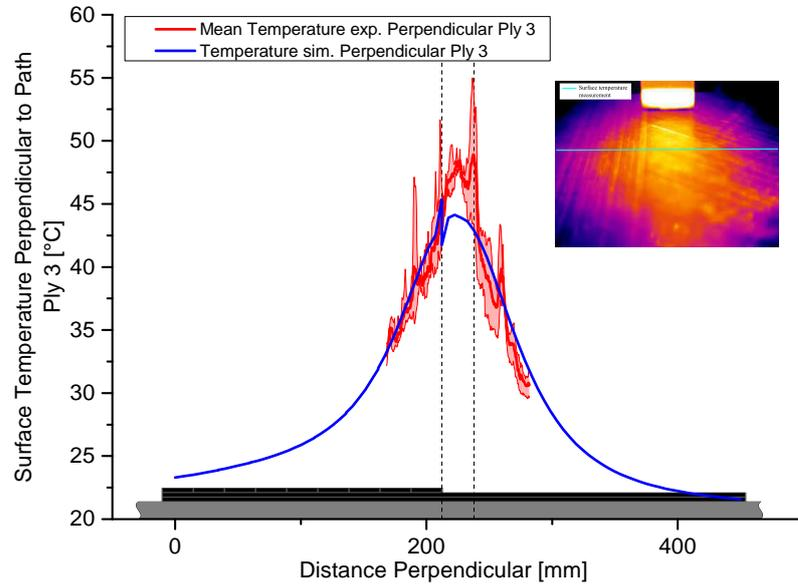
Figure 4.21. Results of Thermography and simulation of surface temperature during the placement of ply 3 [28]
