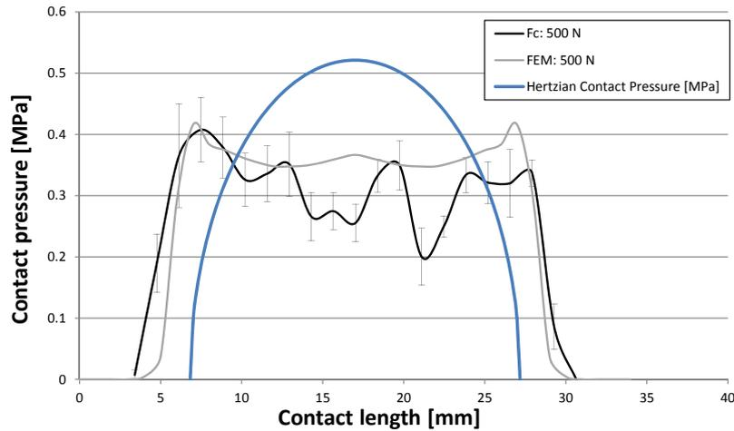
Figure 3.32. Comparison of the experimental and simulation values of static pressure of the compaction roller the analytical hertzian pressure
