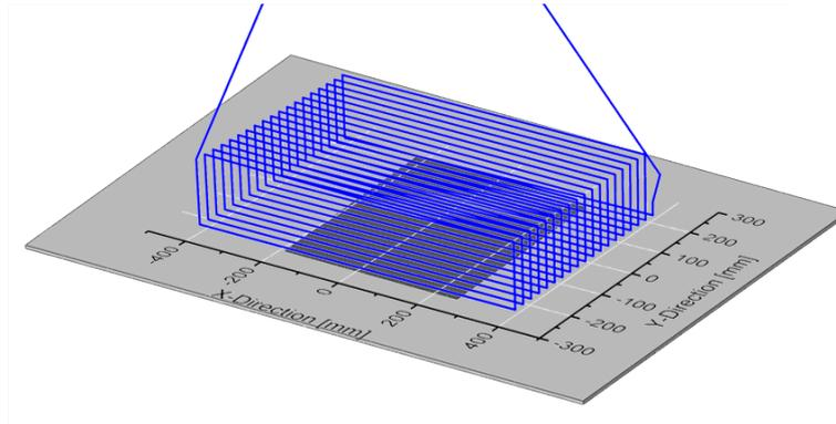
Figure 4.11. Robot Path for the placement on ply 3
