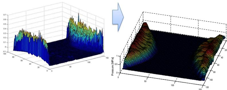
Figure 3.21. Evaluated image of the Prescale results of Test setup 5 (Concave tool lateral) before (l) and after (r) application of the smoothing algorithm
