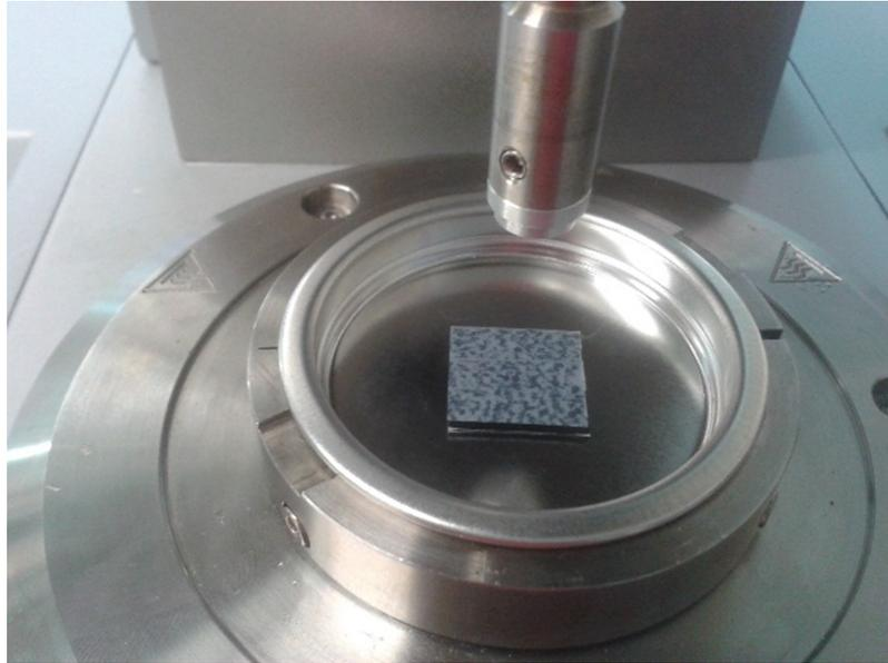
Figure 3.35. Experimental Setup of the compression tests. For elevated temperature a thermal controlled hood was used (not shown).
