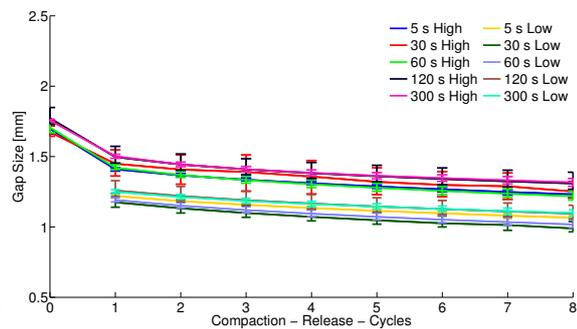
Figure 3.44. Compaction results of UD setup with release time variation
