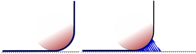
Figure 6.7. Adhesive (left) and cohesive (right) failure mechanisms during peel, compare Lichtinger et al. [29]
