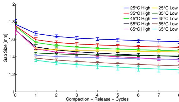
Figure 3.37. Compaction results of MD setup with temperature variation
