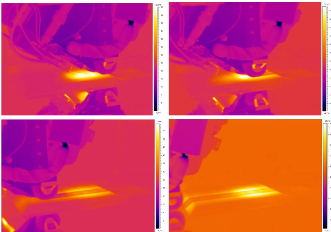
Figure 4.29. Series of images showing the surface temperature during the placement of the first path
