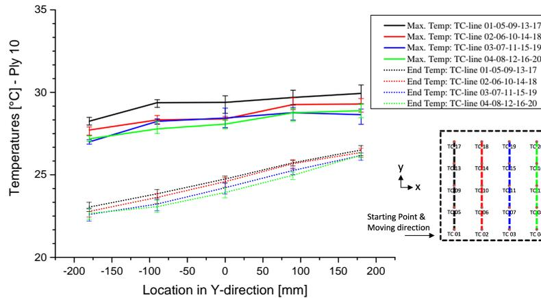
Figure 4.19. Max. and end temperature of ply 10 distributed over the placement area, compare Lichtinger et al. [28]
