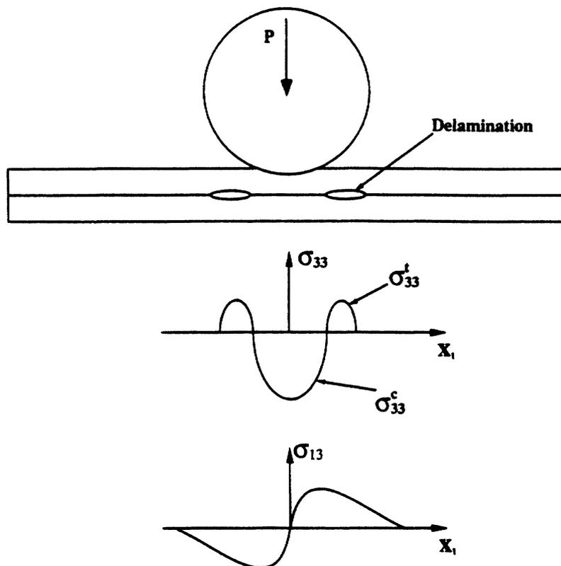
Figure 3.31. Induced stresses under a radial compaction roller from Sarrazin and Springer [17]
