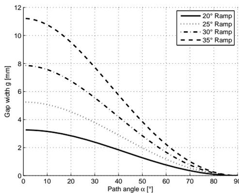
Figure 3.6. Resulting gap width  $g_1$  as a function of path angle for different ramp angles [42].
