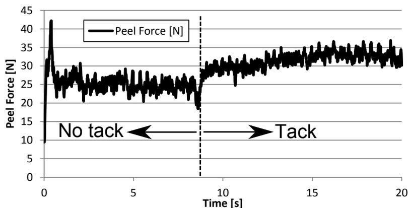
Figure A.1. Measured peel force signal at 25 mm/s peel rate, 3.2 N/mm compaction force and 3 W/mm heat output of the heat source
