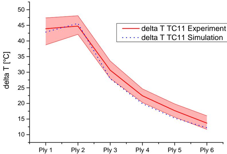
Figure 4.34. Temperature differences while passing of the IR lamp for all six plies: experimental values compared to simulation results
