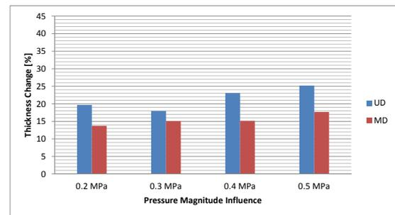
Figure 3.46. Influence of pressure variation on compaction [%] after eight compaction cycles
