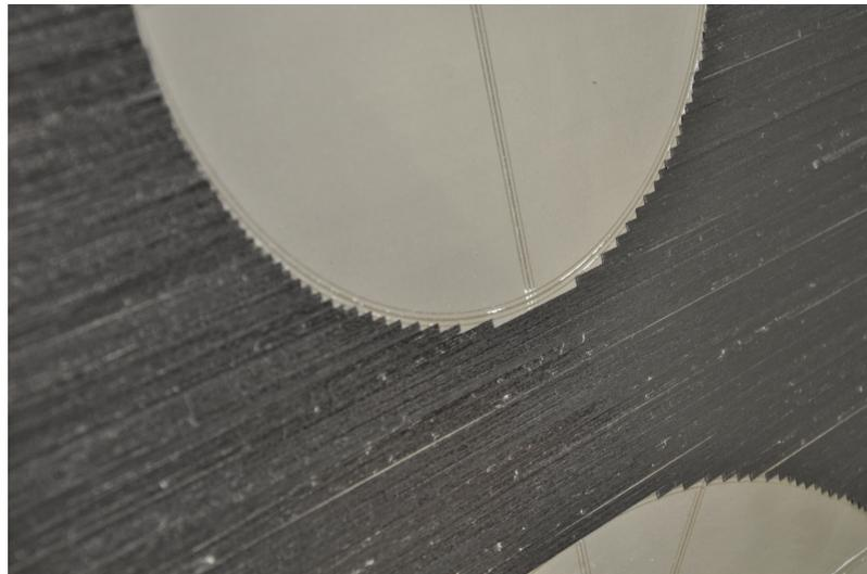
Figure 2.3. Reduced material scrap with the help of cut-and-restart operations and near net shape manufacture
