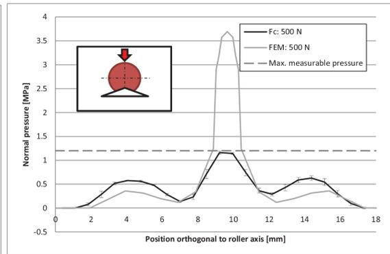
Figure 3.28. Normal pressure of the compaction roller in longitudinal direction orthogonal to roller axis on the convex tool. [42].
