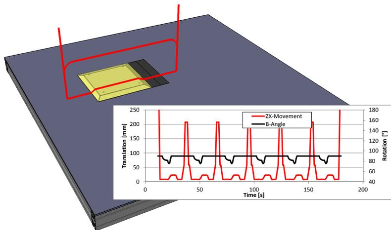
Figure 4.12. CAD Drawing of the test setup of the placement on the tapered honeycomb including the path of the AFP head with superimposed translational (red) and rotational (black) movement of the robot
