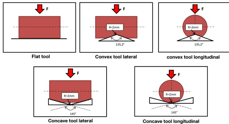
Figure 3.19. Five different test scenarios with three tool designs for static roller tests, according to Lichtinger et al. [42]
