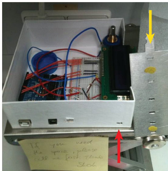
Figure 5.12: The plunger speed measurement device was designed by the author. A laser pointer (not shown) was aligned horizontally to illuminate the photodiode sensor (red arrow). This enables detection of the time differences between holes in the metal pinhole strip (right, yellow arrow, built by the workshop) when it is attached to a plunger and dropped.
