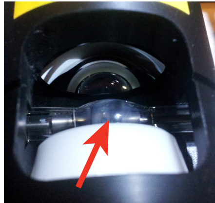
Figure 5.24: UV flash lamp deterioration by contamination build-up (red arrow) on the glass surface. In the back, part of the parabolic reflector can be seen.
